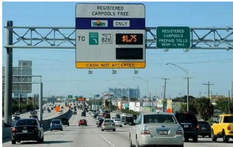
Figure 2.3: Posted Dynamic Toll Price on I-95 Express Lanes in Florida (Source: Link )
