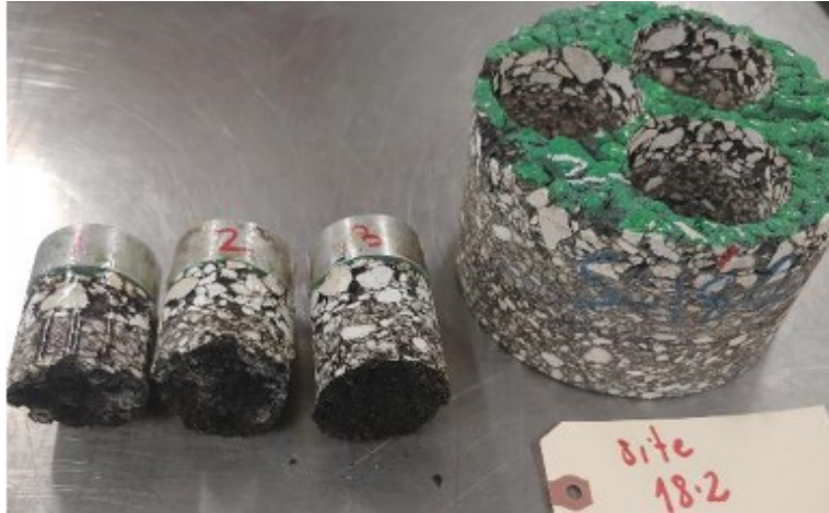
Figure B-13. Pull-Off Test for Specimen 18-2.
