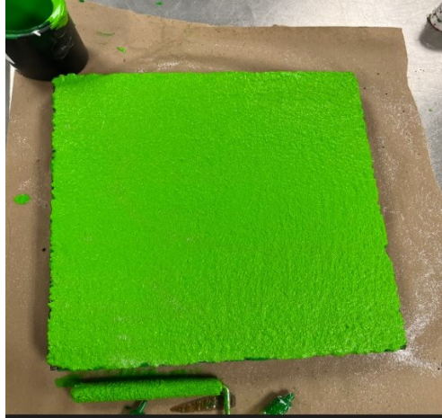
Figure 4-1. GCPM Slab Immediately after Application of MMA.
