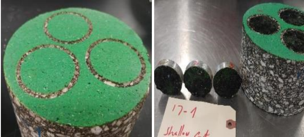
Figure 3-13. Forced Surface Debond.
