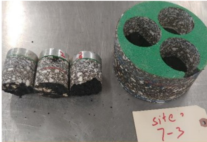
Figure B-16. Pull-Off Test for Specimen 7-3.
