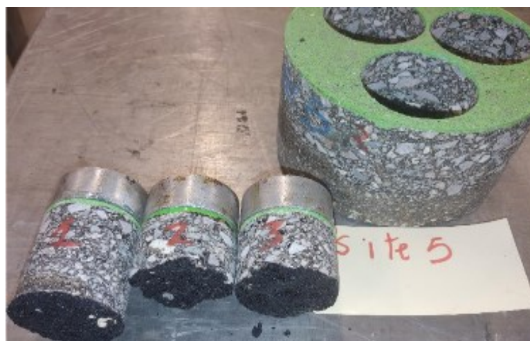
Figure B-4. Pull-Off Test for Specimen 5-1.
