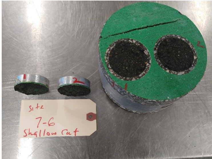
Figure B-18. Pull-Off Test for Specimen 7-6.
