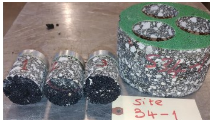
Figure B-6. Pull-Off Test for Specimen 34-1.
