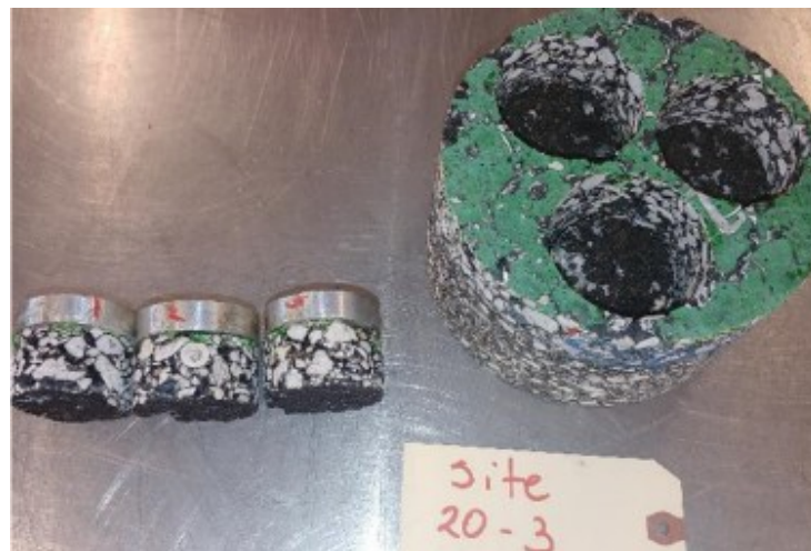
Figure B-10. Pull-Off Test for Specimen 20-3.
