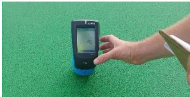
Figure 3-4. Green Color Recording Using Spectrophotometer.
