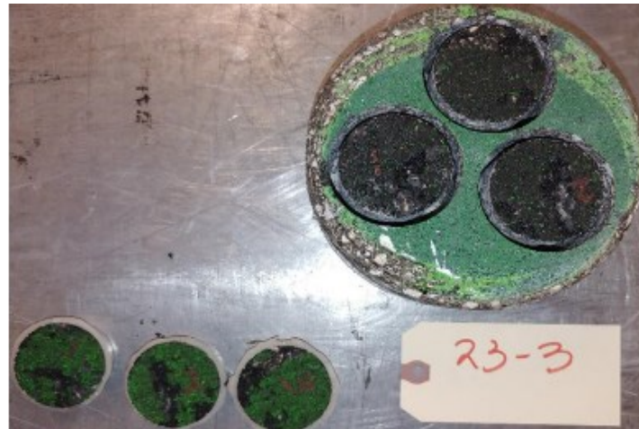
Figure B-3. Pull-Off Test for Specimen 23-3.
