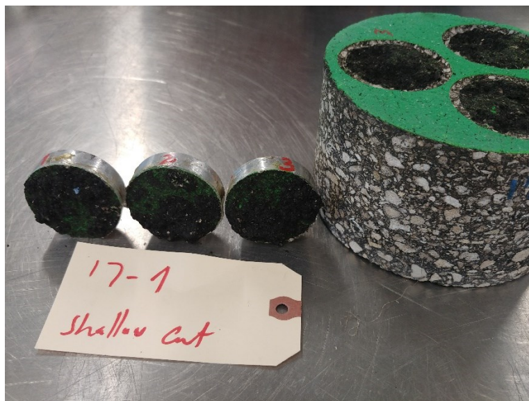
Figure B-19. Pull-Off Test for Specimen 17-1.
