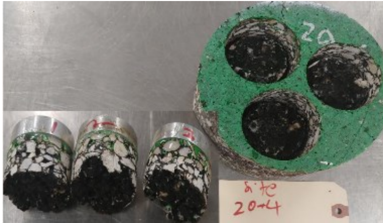
Figure B-11. Pull-Off Test for Specimen 20-4.
