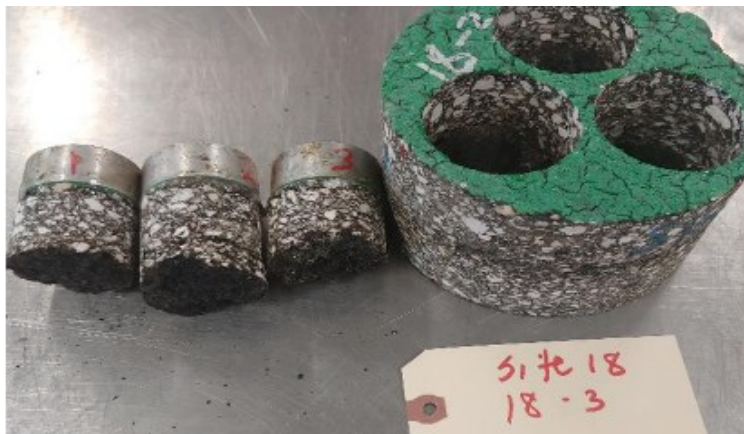
Figure B-14. Pull-Off Test for Specimen 18-3.
