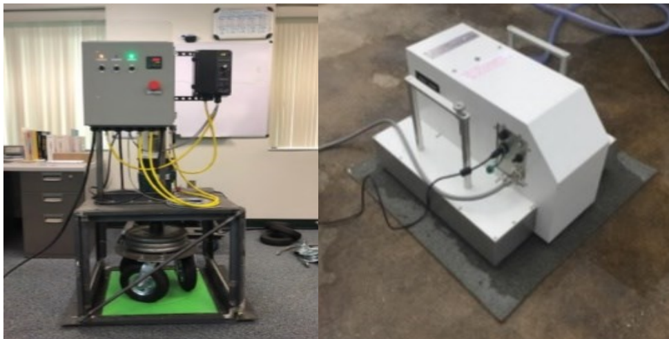
Figure 2-8. Three-Wheel Polisher and Dynamic Friction Tester.
