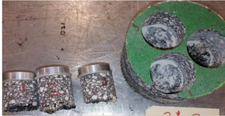
Figure B-1. Pull-Off Test for Specimen 21-1.
