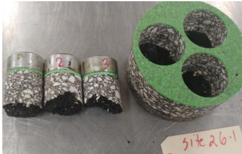
Figure B-17. Pull-Off Test for Specimen 26-1.
