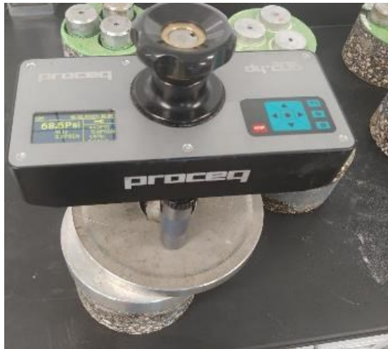
Figure 3-9. Pull-Off Test in Progress.
