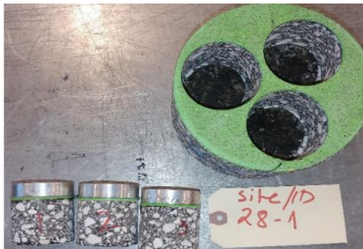
Figure B-8. Pull-Off Test for Specimen 28-1.
