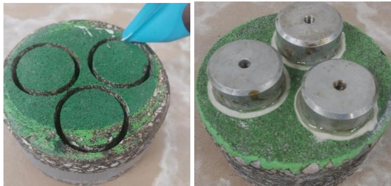
Figure 3-8. Gluing the Pull-Off Test Loading Discs.
