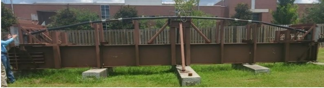
Figure 80. Filled external tendon mock-up
