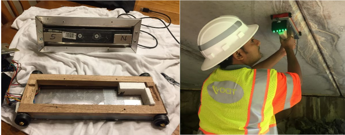
Figure 28. MFL device for corrosion detection in traditional prestressed (pre-tensioned) concrete box girders 28
