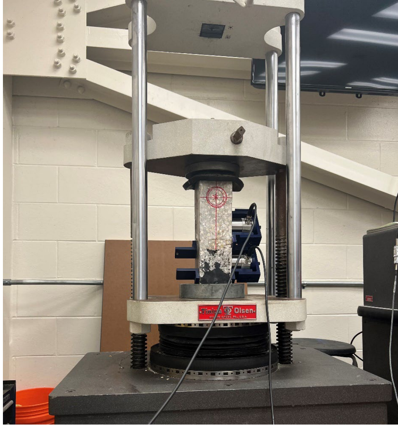
Figure 113. Testing setup for small-scale block testing
