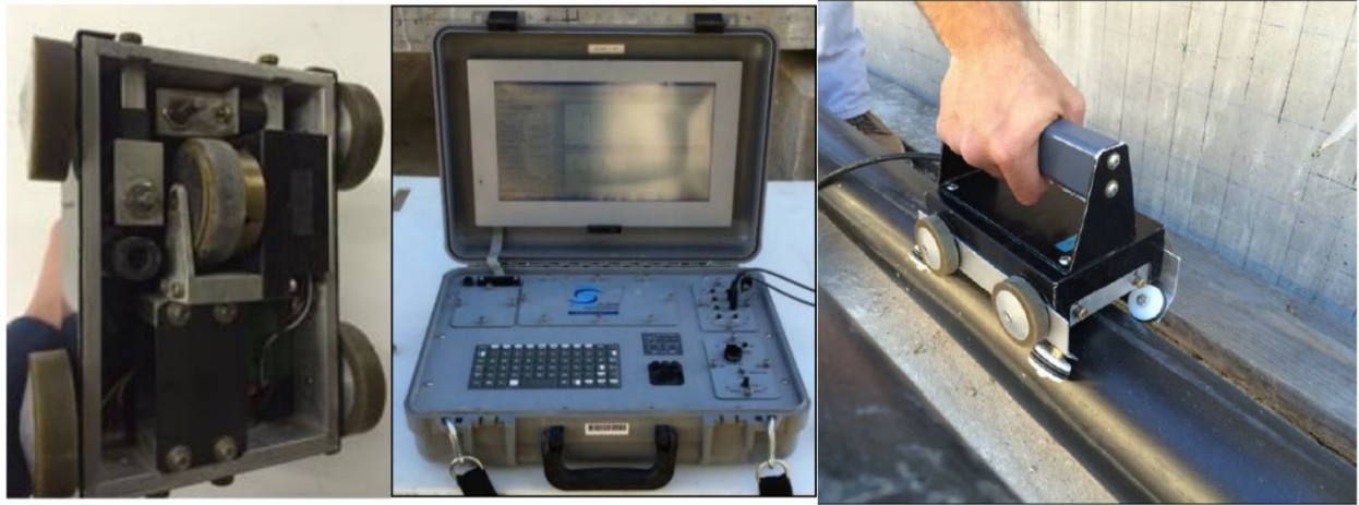
Figure 40. IE scanner test head, the PC data acquisition platform, and the IE device in use on an external duct (Hurlebaus et al. 15 )
