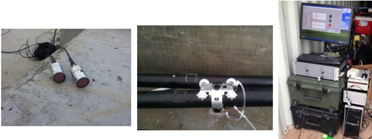
Figure 44. Pulse transmitter and receiver, prototype scanning head with encoder and data acquisition system
