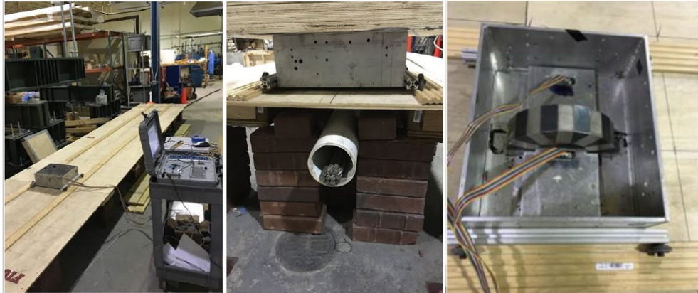
Figure 18. Experimental testbed and sensor for MFL inspections by Azizinamini 21
