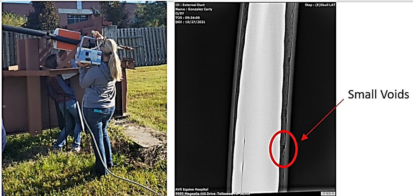
Figure 88. Specimen 2: filled duct results
