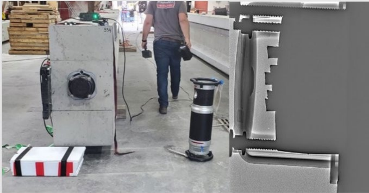
Figure 91. YXLON machine on internal specimen anchorage cap
