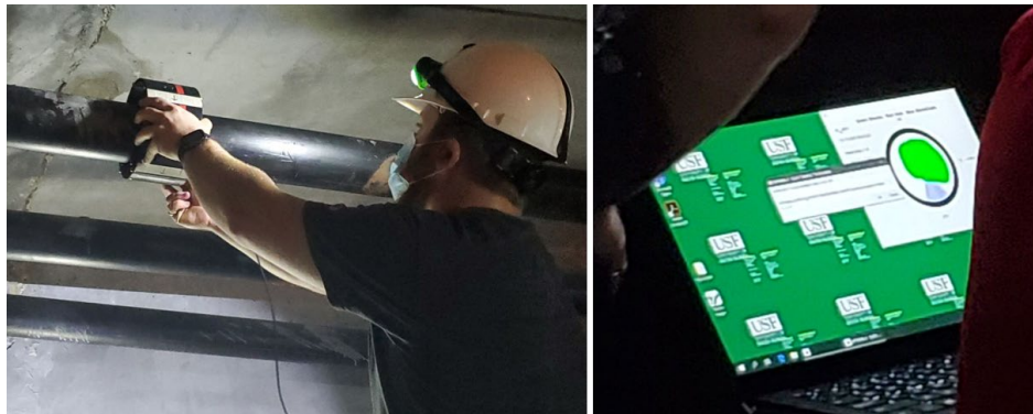
Figure 6. Electrical impedance inspection. Broadway Bridge, Daytona Beach
