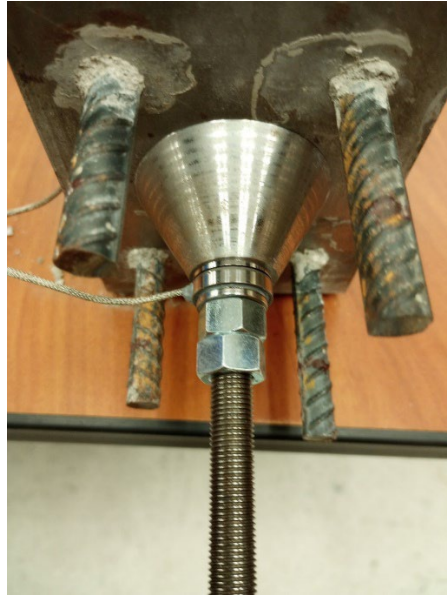
Figure 114. Load cell used for post-tensioning measurements on small-scale beam
