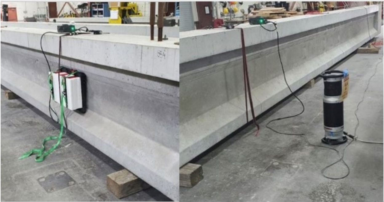
Figure 90. YXLON X-Ray machine on internal duct specimen
