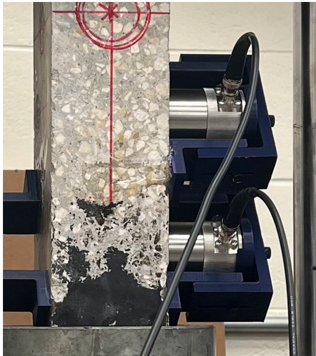
Figure 107. Test setup for compressive loading with fixture-assisted mounting for UT transducers.
