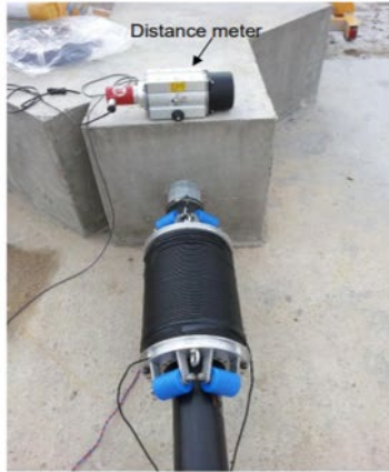
Coil System around the PT duct
