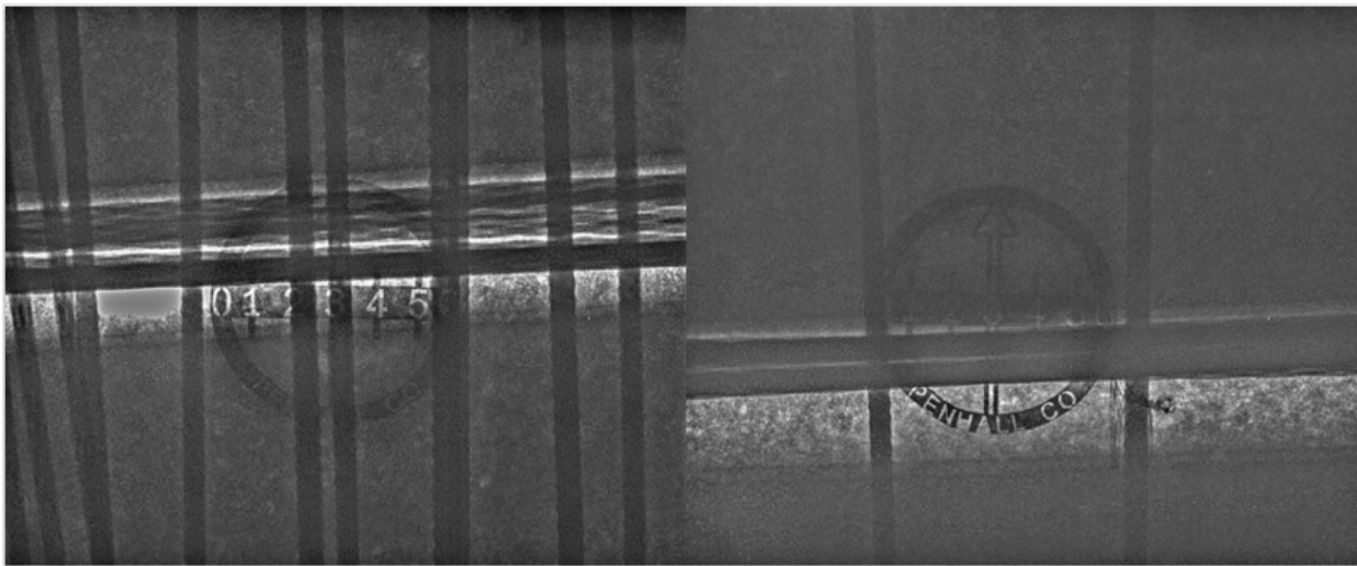
Figure 93. Internal Duct Specimen: duct with strands 1ft away from end block (Left) and 5ft away from end block (Right)
