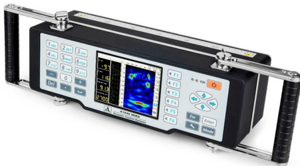
Figure 41. A1040 MIRA device and results from the deviator blocks (left is defect key, and right is the UST scan) (Hurlebaus et al. 15 )
