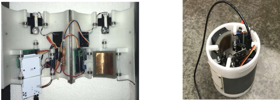
Figure 25. Layout of electronics for tendon imaging unit 10
