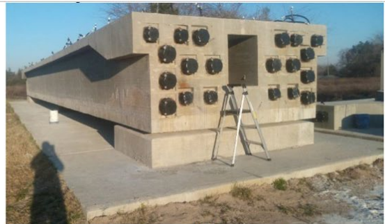
(e) Finished post-tensioned (U-beam) girder specimen
