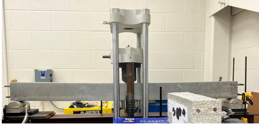
Figure 112. 3-point load testing frame and the Tinius and Olsen universal testing machine.
