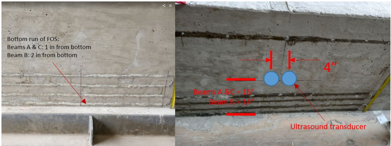
Figure 137. Fiber-optic sensor location and ultrasound transducer location for post-tensioning
