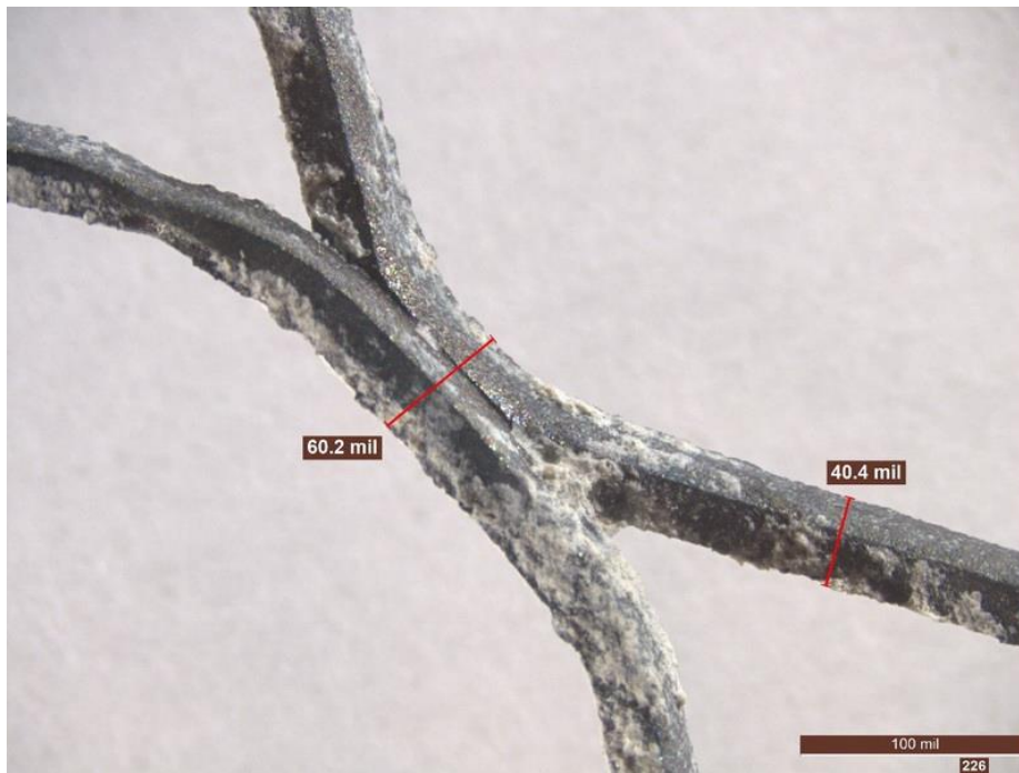
Figure 68. Microscopic view of titanium mesh, including thickness measurements (Gandy 226)
