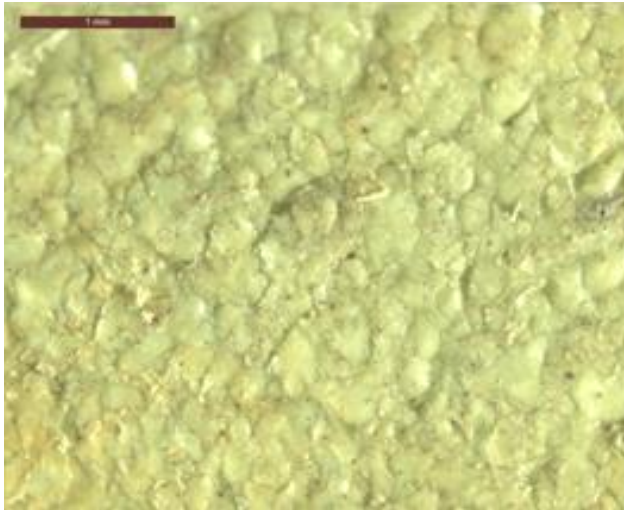
Figure 37. A2-1 30-40% Backside Contamination.
