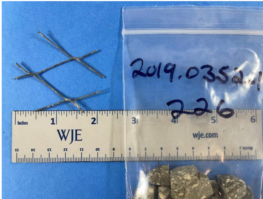
Figure 67. Representative titanium mesh sample (Gandy 226)
