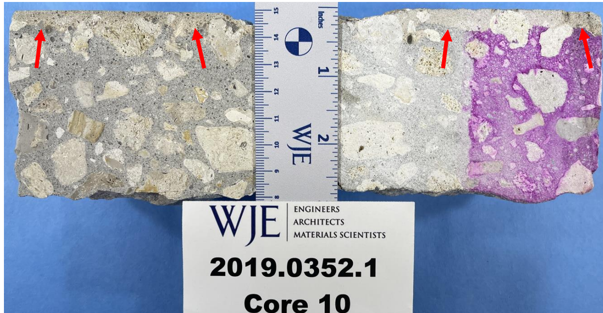
Figure 119. Core 10. Lapped cross section and matching saw-cut section stained with phenolphthalein solution to determine the depth of carbonation, which was approximately 0.3 inch as indicated by red arrows. Distribution of paste and aggregate appeared to be uniform and the concrete was well consolidated.
