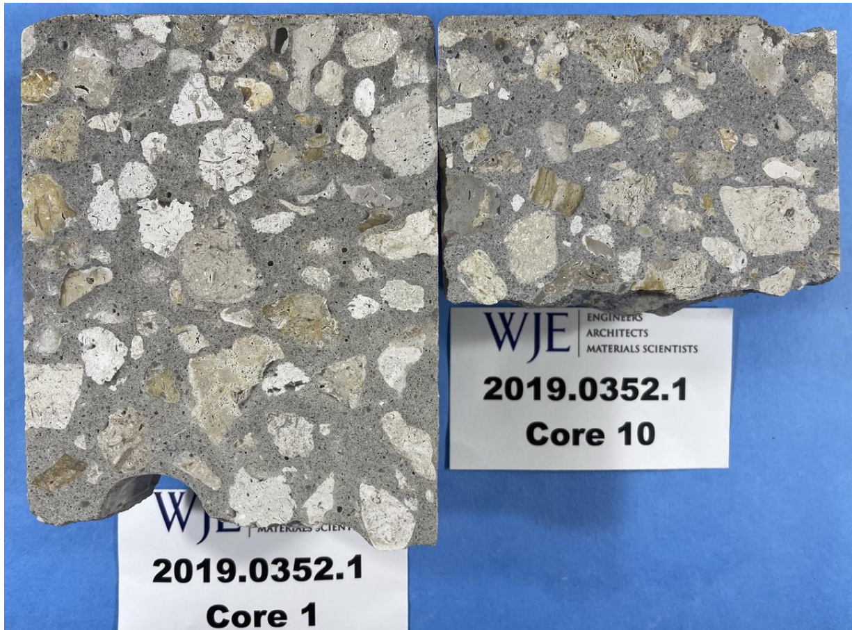
Figure 120. Core 1 and Core 10. Lapped cross sections show the overall similarity between the two cores.
