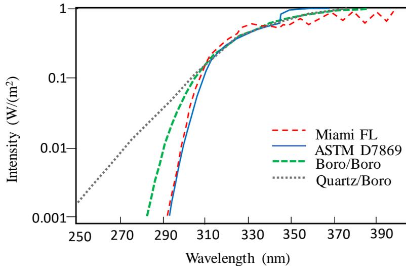
Figure 12 – The spectral power distribution of xenon lamp with different types of filters together with the noon-time sunlight in Miami, Florida. (replotted from Berry et al., 2018)
