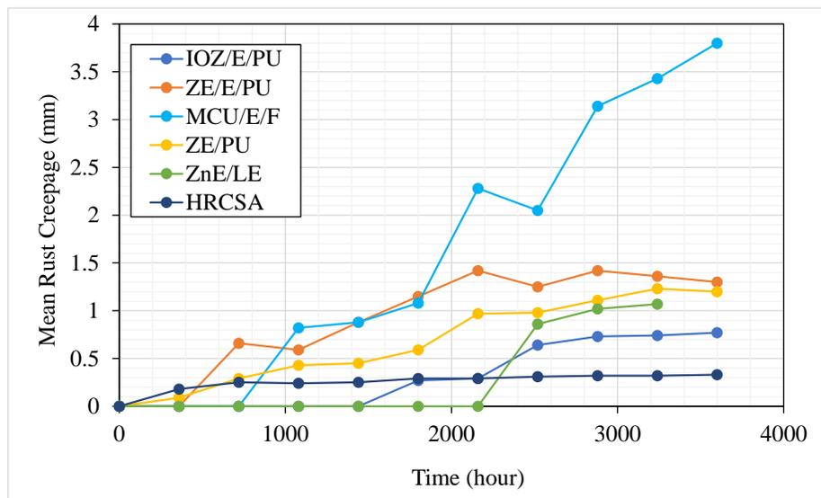
Figure 7 – Mean creepage value versus ALT time.
