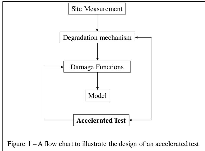
Figure 1 – A flow chart to illustrate the design of an accelerated test
