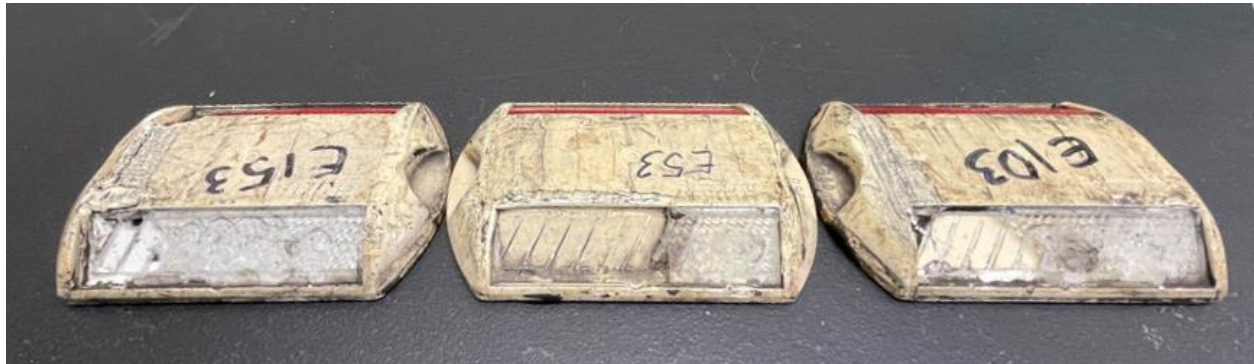
Figure 5-14. Low retroreflectivity RPMs with MRU readings below 10,000 R_L .
