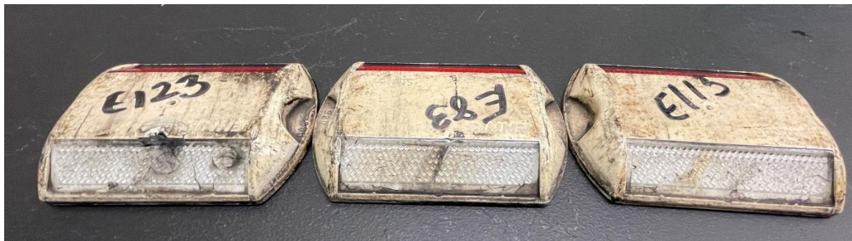
Figure 5-15. Mid retroreflectivity RPMs with MRU readings between 10,000 and 30,000 R_L .
