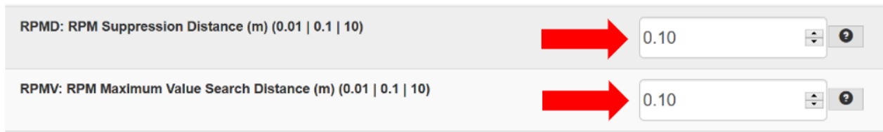
Figure C-2. RPM parameters exclusive to the updated Laserlux firmware (post v1.318).
