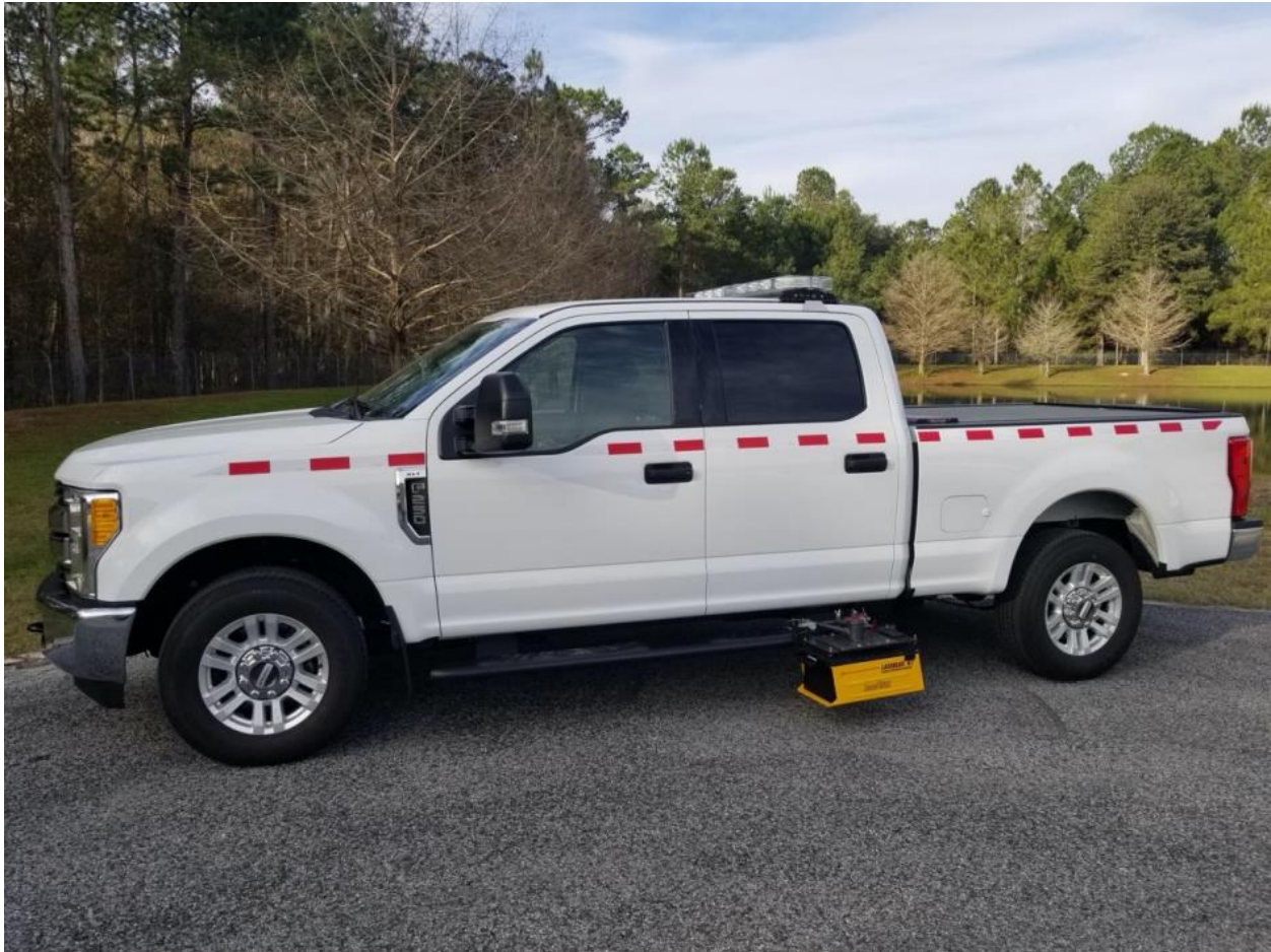
Figure 5-1. High-speed testing vehicle equipped with the modified MRU device.
