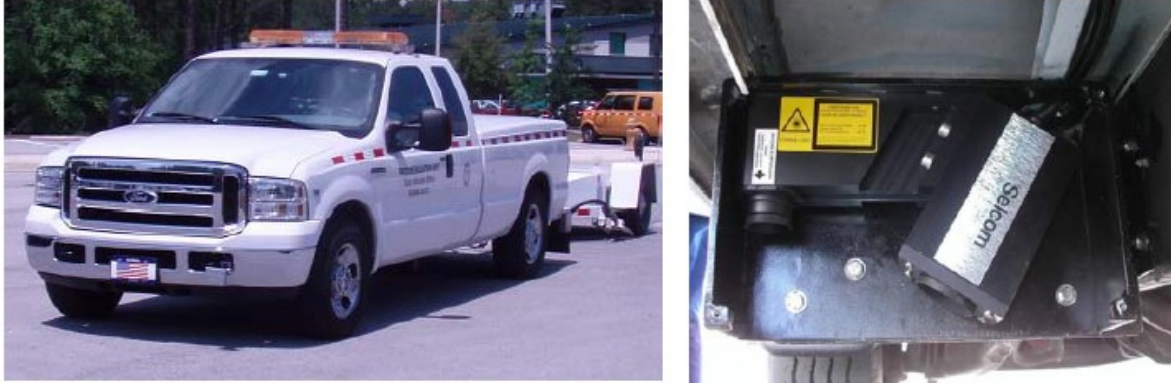
Figure 2-6. Test vehicle (left). Point-laser measurement device (right) [17].
