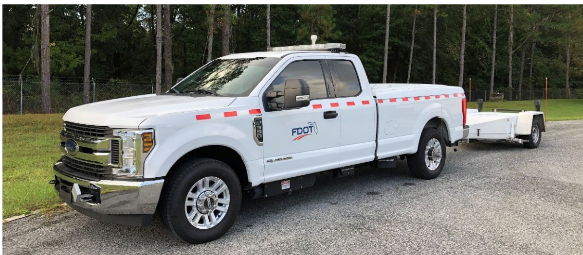
Figure 3-6. FDOT pavement friction testing unit with line-laser.
