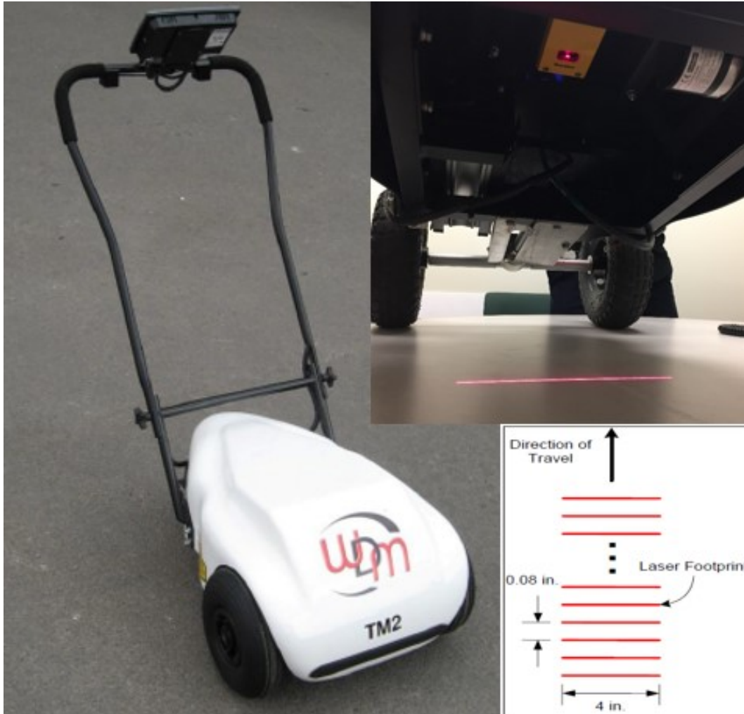
Figure 3-10. Texture meter 2 (TM2) [26].
