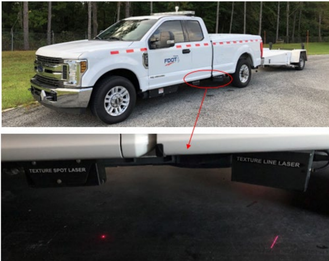
Figure 5-5. Unit 12 test vehicle (top). Texture laser locations (bottom).
