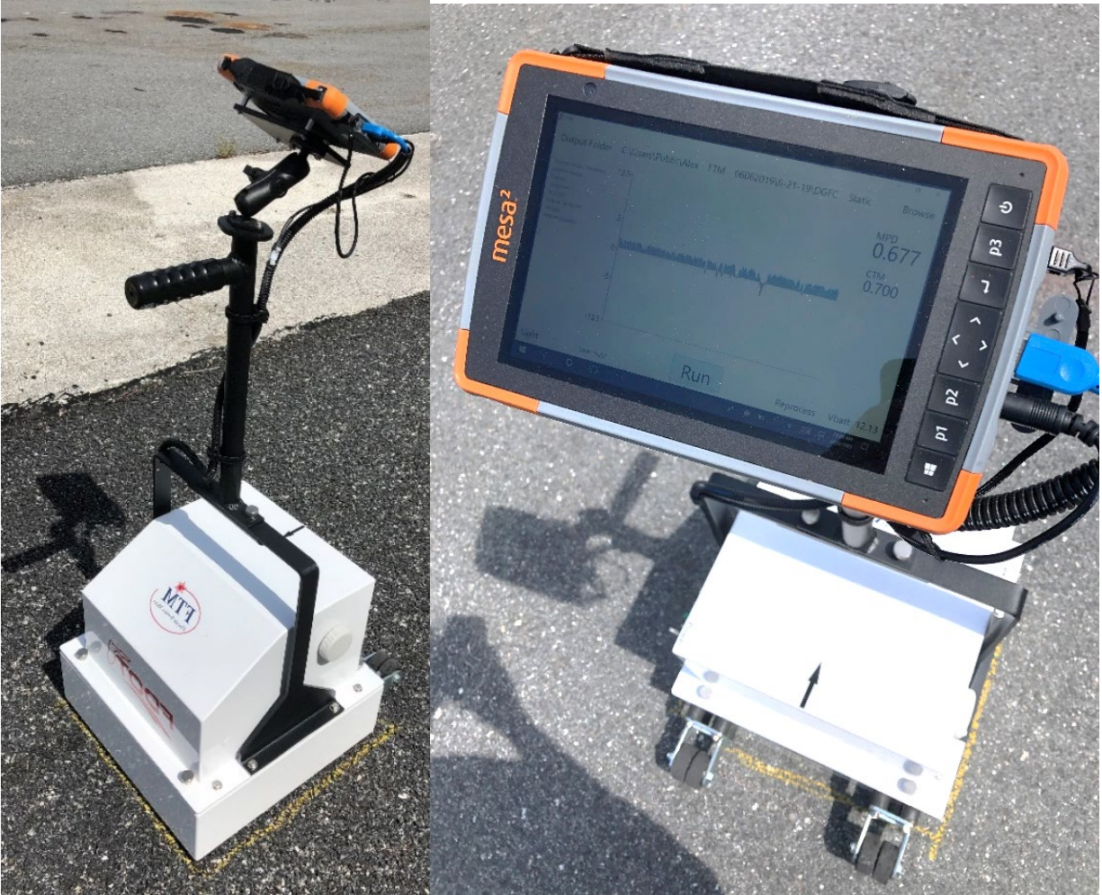
Figure 3-9. Fast texture meter (FTM).
