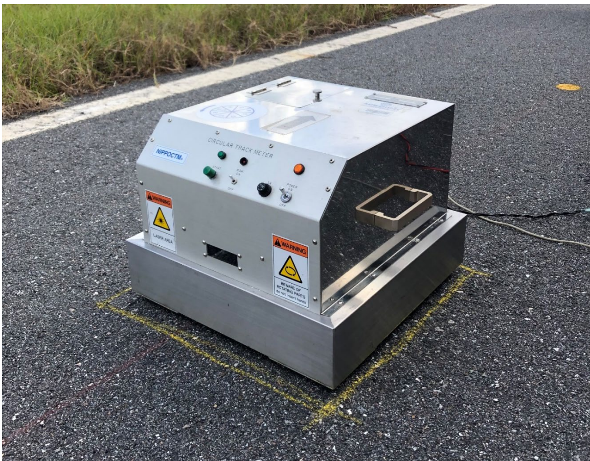
Figure 4-9. CTM measurement at Williston Airport.
