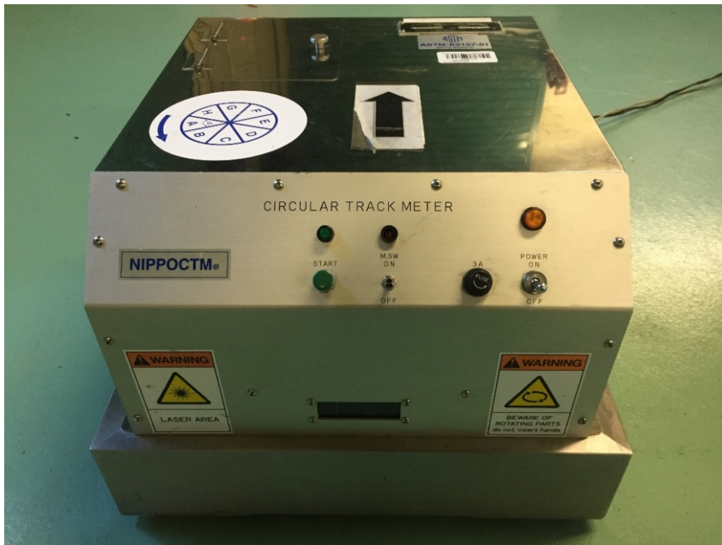
Figure 3-7. Nippo Sangyo circular track meter.
