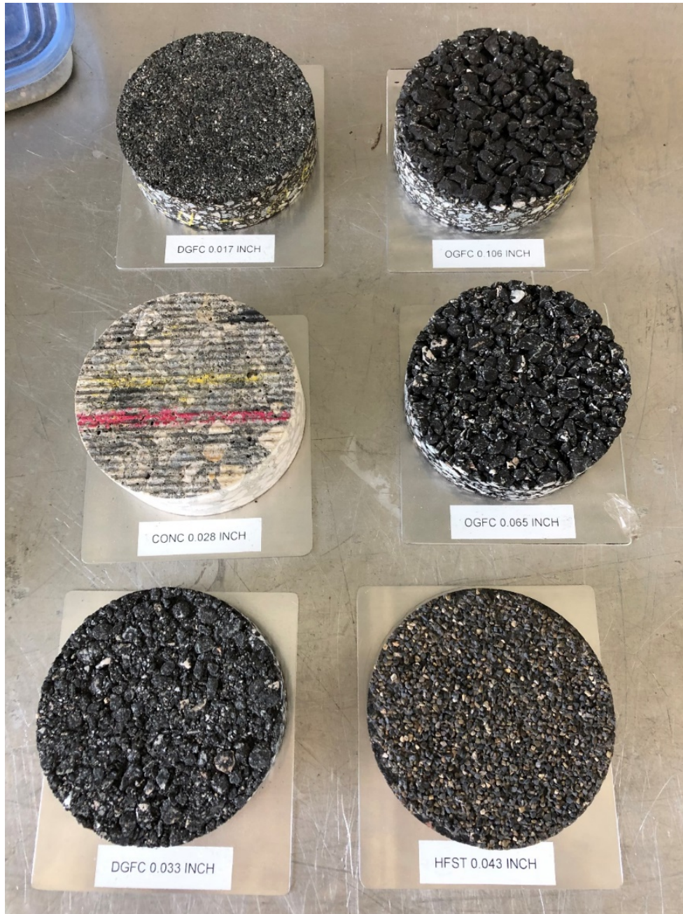
Figure 3-13. FDOT pavement samples.
