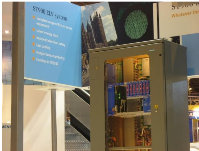
Figure 2. Siemens ST900 ELV system
