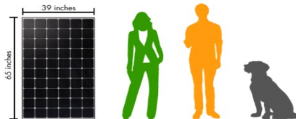
Figure 12. Solar panel size [58]
