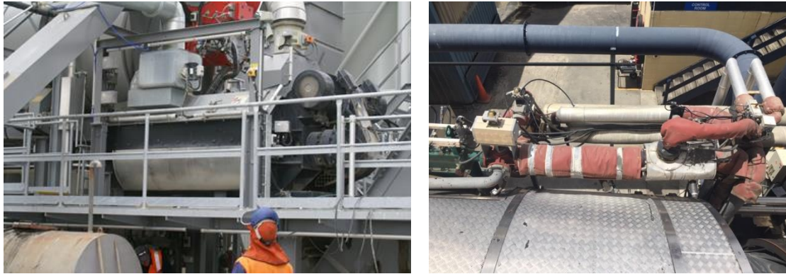
Figure 26. In-line Mixing Chamber at a Drum Plant in New Zealand (Waters et al., 2018; van de Linda, 2019)
