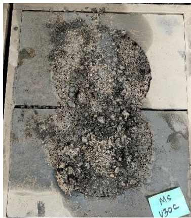
Figure 114. U30C GRN3 Mixture Specimens after Testing in HWTT
