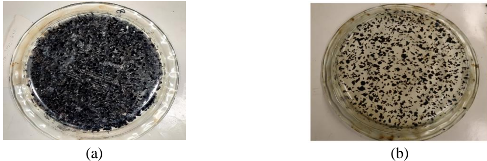
Figure 87. Pie Plates of GRN2 Mixture with J30Z EMA Binder at JMF OBC (6.6%): (a) With Loose Mixture, (b) Without Loose Mixture
