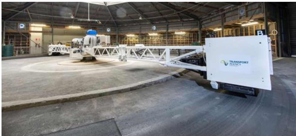
Figure 17. EMA OGFC Test Section at CAPTIF (Herrington et al., 2007)
