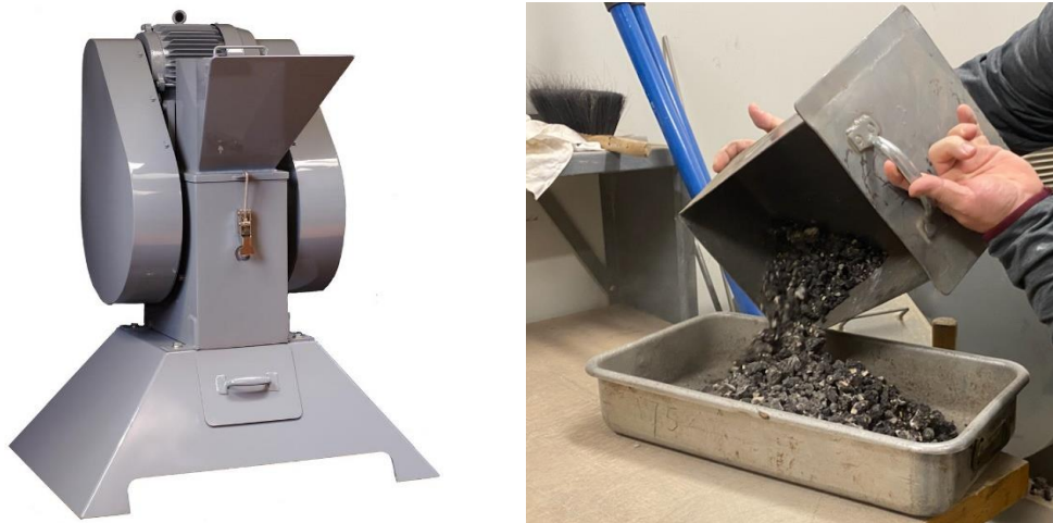
Figure 117. Jaw Crusher (left) and Loose Mixture Particles after Crushing (right)
