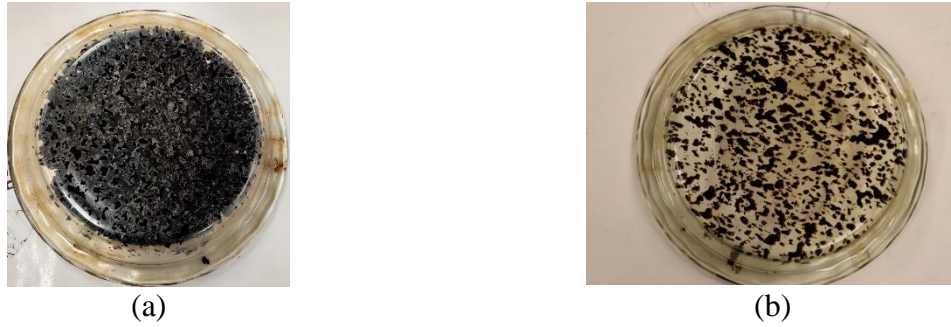
Figure 84. Pie Plates of GRN1 Mixture with U30C EMA Binder at JMF OBC (6.8%): (a) With Loose Mixture, (b) Without Loose Mixture
