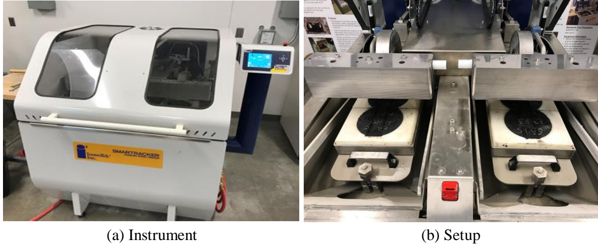
Figure 5-12. HWT Test: (a) Instrument; (b) Setup
