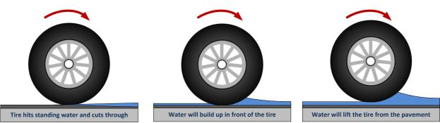
Figure 1. Simplified illustration of hydroplaning.
