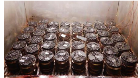
Pavement samples are conditioned by the asphalt pavement weathering system.
