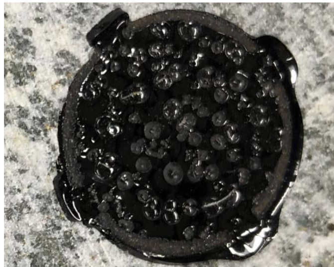
Figure 23. Cohesive Failure in the BBS Test
