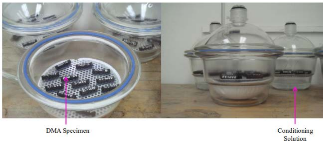
Figure 8. FAM Specimens Conditioned in Vacuum Desiccators (Tong, 2013)
