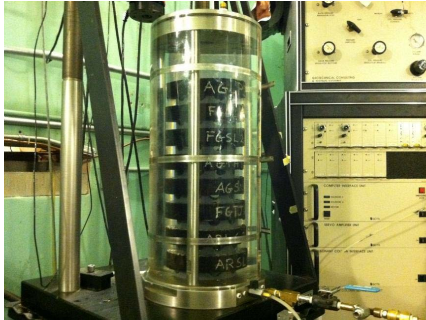
Figure 7. CPPC System and Triaxial Chamber (Roque et al., 2012)
