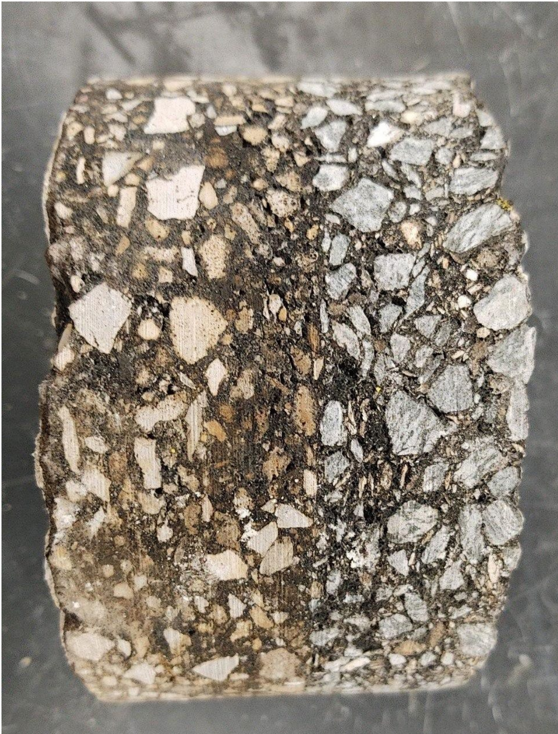
Figure 4-89. Close-up of Air Voids at US 17 Worm Core Layer Interface
