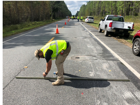
Figure 3-15. PCI Rutting Survey Process
