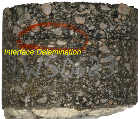
Figure 4-52. SR 26 MP 8.837 Worm Core Cross-Section – Stripping/Voids at Layer Interface
