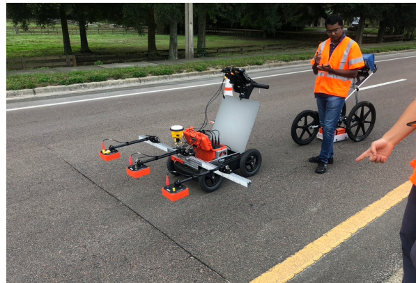
Figure 3-17. GSSI PavScan RMD
