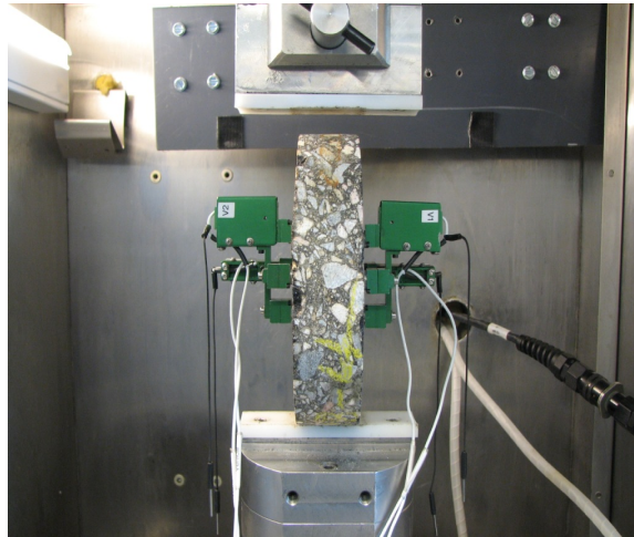
Figure 4-99. Indirect Tensile Test Setup
