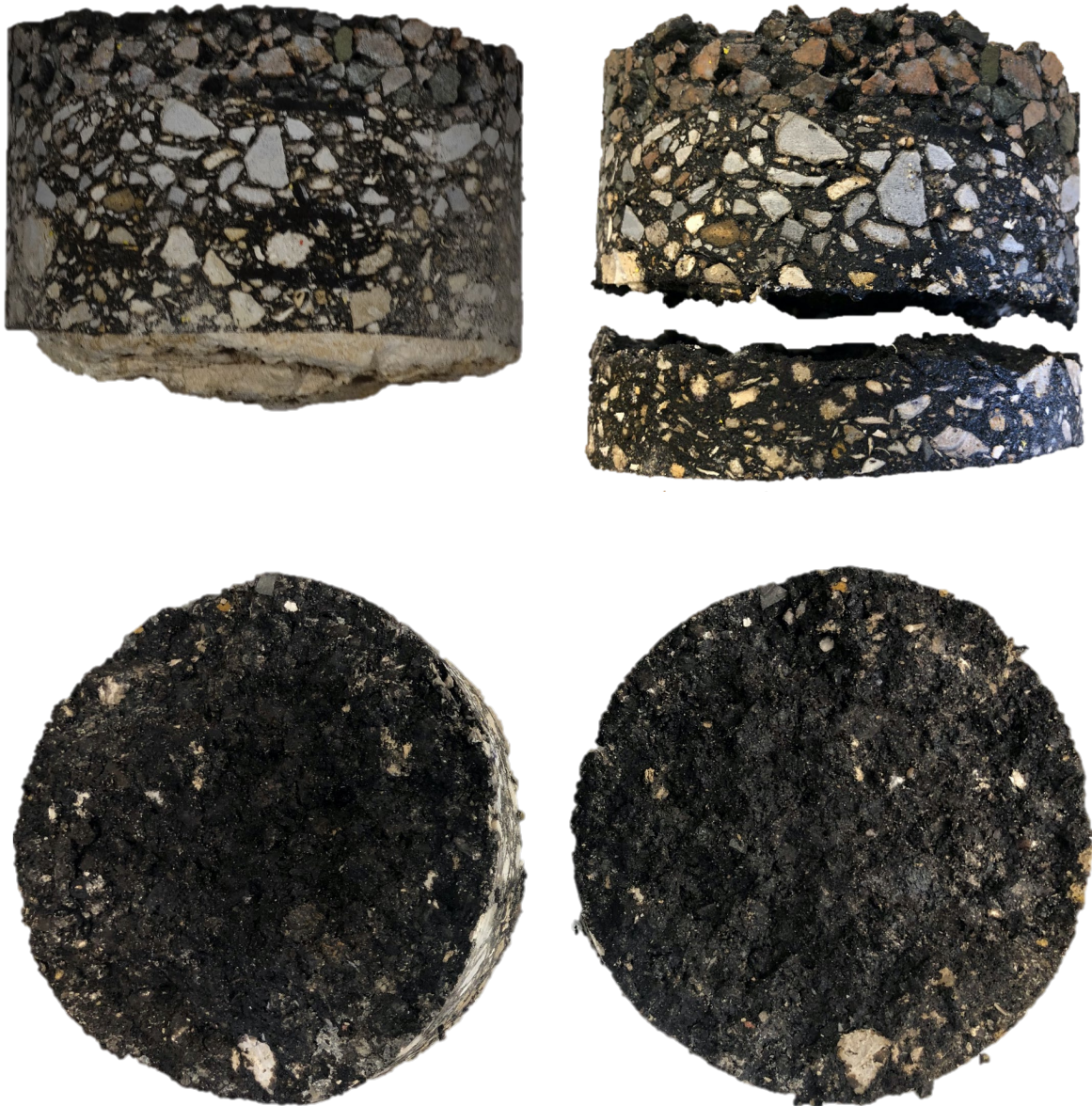
Figure 4-94. US 17 Control Section MP 17.401 Bond Test Failure Outside of Interface
