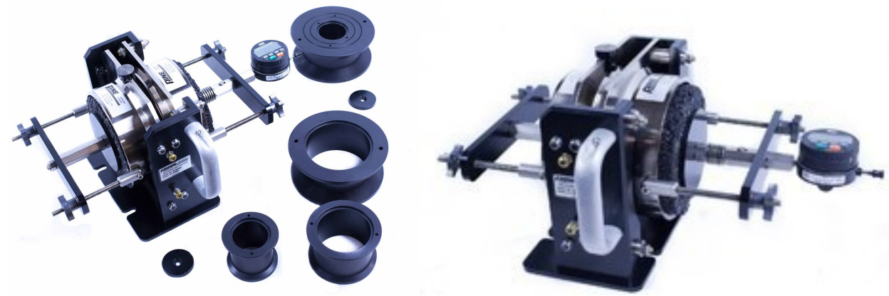
Figure 2-3. Bond Strength Shear Test Fixture
