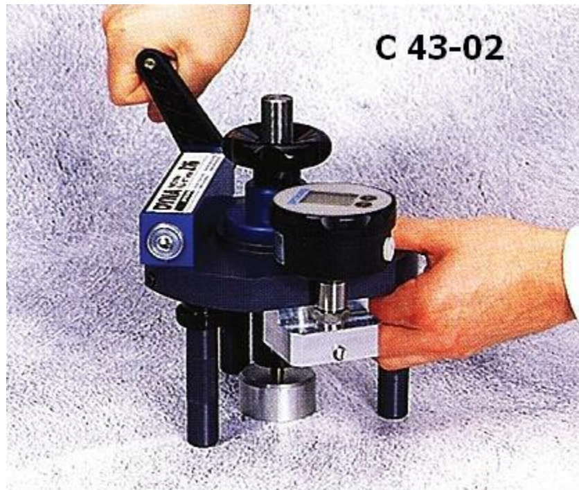
Figure 2-2. Tensile Pull-Off Tester
