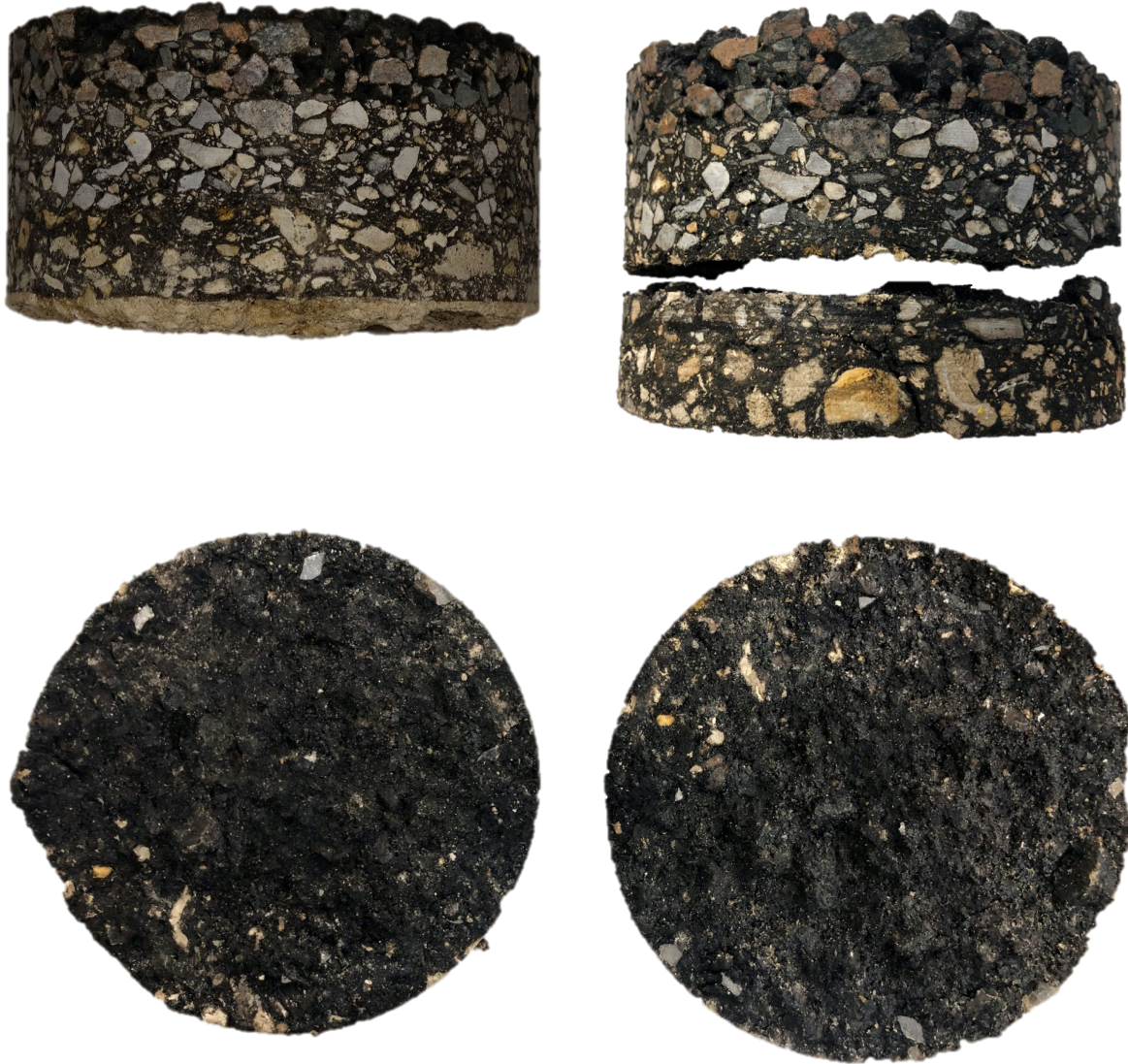
Figure 4-93. US 17 Control Section MP 17.403 Bond Test Failure Outside of Interface
