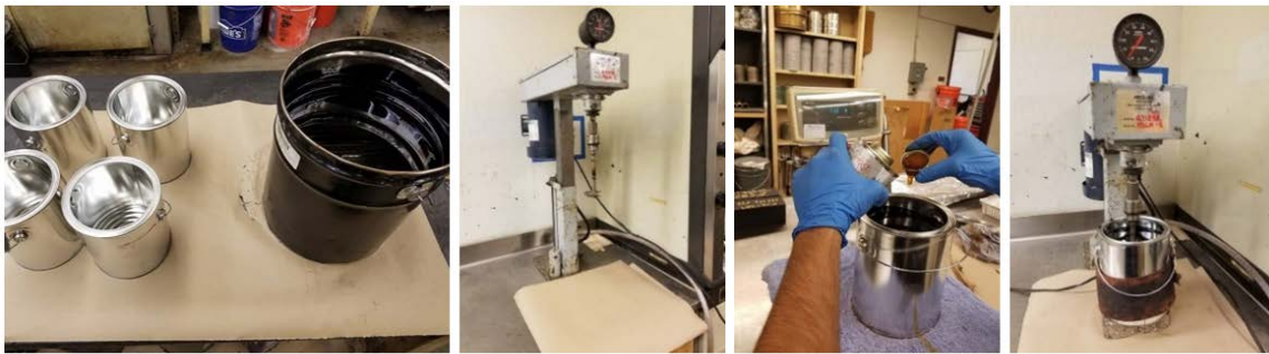
Figure 3-2. Steps followed to mix the liquid anti-strip with asphalt binder.
