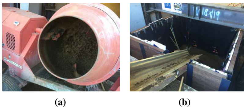
Figure 7-23. SG deposition: (a) soil mixing in the mechanical mixer, and (b) placement of moist soil in PaveBox.
