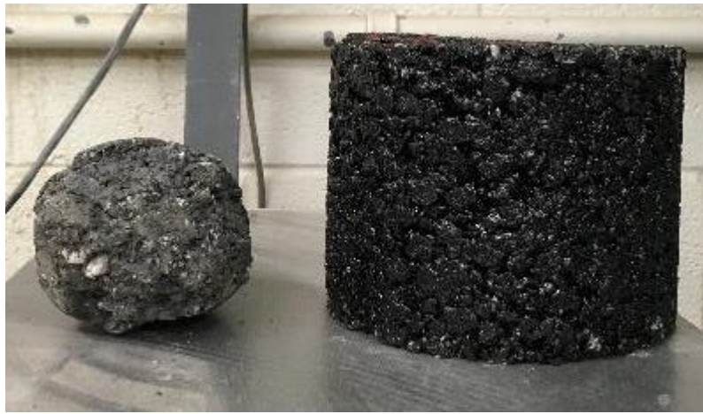
Figure 5-22. Comparison of a Granite-PMA Cantabro Specimen That Reached 80% Mass Loss with Respect to Its Initial Condition.
