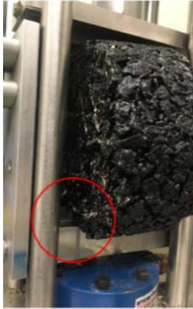
Figure 5-19. Specimen in Contact with the Edge of the IDEAL-CT Loading Frame during Testing.
