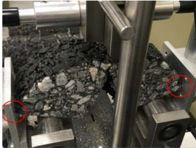
Figure 5-14. Specimen of a Granite-HP Binder Mixture in Contact with the Edges of the SCB Loading Frame during Testing.
