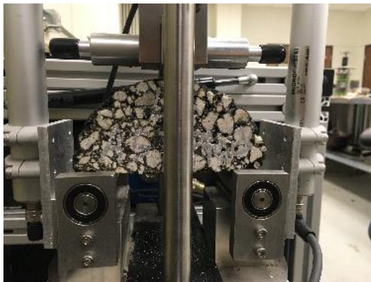
Figure 5-13. Semicircular Bending Test Setup.
