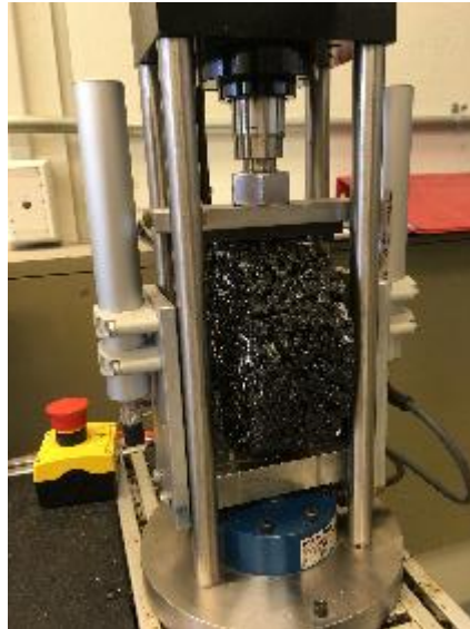
Figure 5-18. IDEAL-CT Test Setup.
