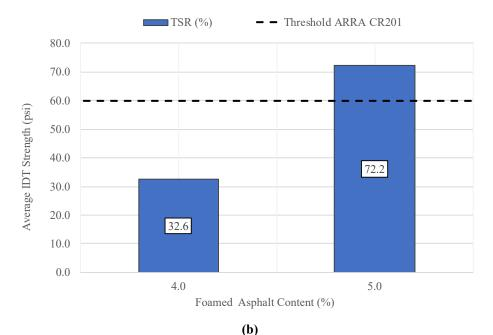
Figure 93. Foamed Cold Recycled Mixture Trial Results: (a) IDT Strength and (b) TSR
