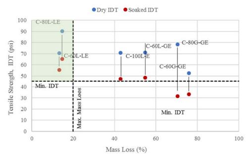
Figure 143. Cantabro Mass Loss and IDT, Cold Recycling—Emulsion
