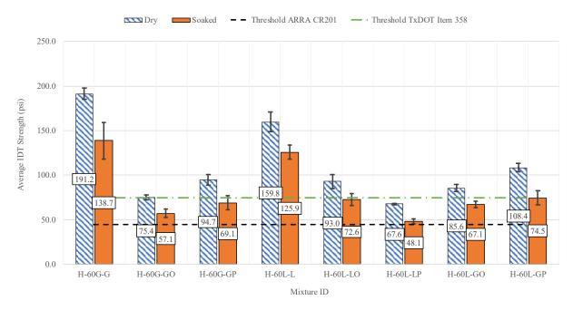
Figure 59. Hot Recycled Mixtures' Unconditioned and Moisture Conditioned IDT Strength
