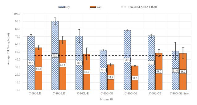
Figure 78. Emulsified Cold Recycled Mixtures' IDT Strength Results
