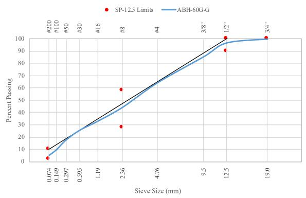
Figure 57. ABH-60G-G Aggregate Blend Gradation Curve
