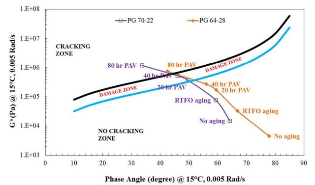
Figure 4. Black Space Diagram for Two Virgin Binders with Various Levels of Aging
