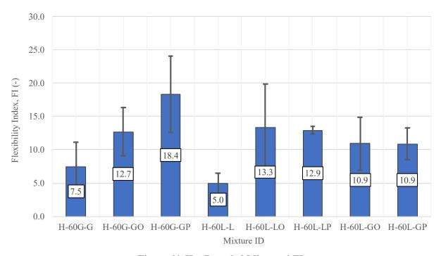
Figure 64. Hot Recycled Mixtures' FI
