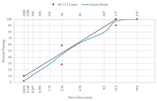
Figure 52. Granite Aggregate Blend Gradation Curve
