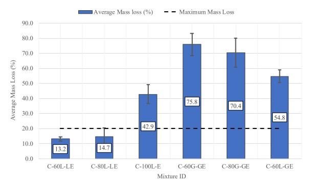
Figure 84. Emulsified Cold Recycled Mixtures' Cantabro Abrasion Mass Loss
