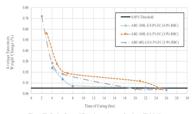
Figure 73. Curing Protocol Experiment Average Specimen Weight Loss
