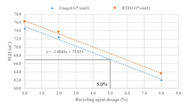
Figure 47. Recycling Agent Dose Verification for Blends with PG 52-28 Virgin Binder + O2 + Extracted and Recovered RAP from Stockpile 1-09
