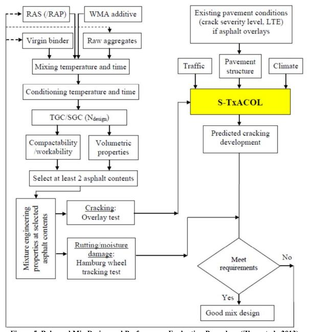
Figure 5. Balanced Mix Design and Performance Evaluation Procedure (Zhou et al., 2013)
