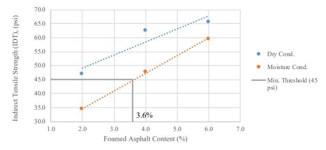
Figure K.9. Example of IDT Strength vs. Foamed binder Content ( $P_b$ )
