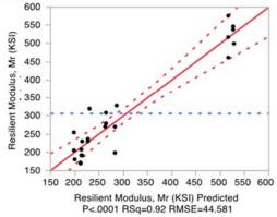
Figure R.9. JMP Statistical Package Output, Hot Recycled Mixtures M<sub>R</sub>
