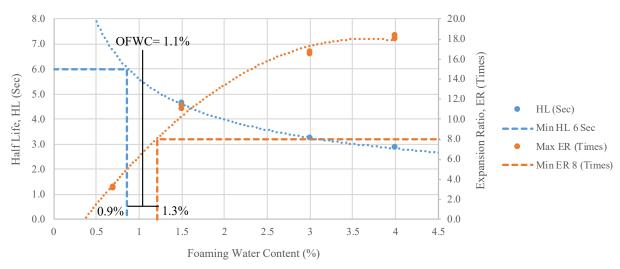
Figure K.8. Example of Optimum Foaming Water Content Determination
