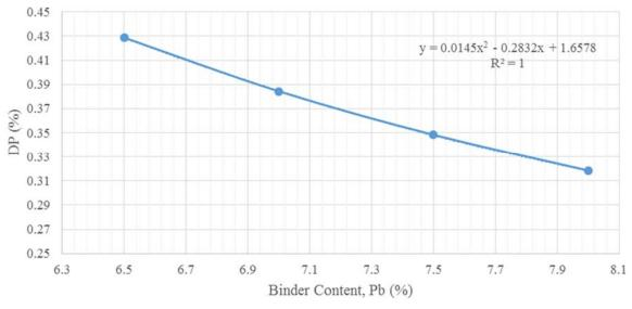
Figure M.3. DP Results, Limestone Mixture
