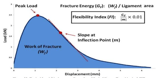
Figure 32. Typical Load-Displacement Curve for a Virgin Mixture Tested in the I-FIT
