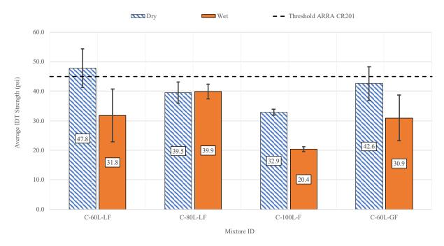
Figure 98. Indirect Tensile Strength of Foamed Cold Recycled Mixtures
