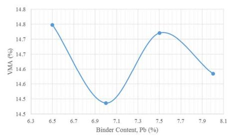
Figure M.2. VMA Results, Limestone Mixture
