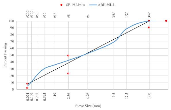
Figure 56. ABH-60L-L Aggregate Blend Gradation Curve
