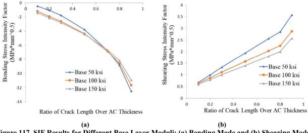
Figure 117. SIF Results for Different Base Layer Moduli: (a) Bending Mode and (b) Shearing Mode
