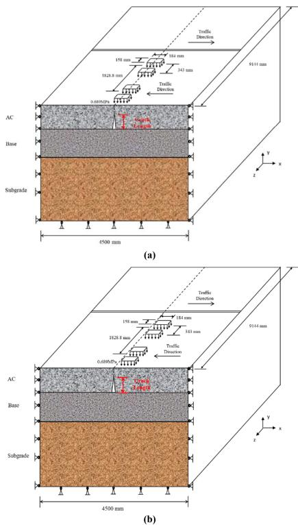
(b) Figure 114. Pavement Structure and Loading Schematic for SIF Analysis at (a) Bending Mode  $(K_1)$  and (b) Shearing Mode  $(K_2)$
