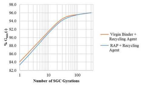
Figure J.2. Recycling Agent O2 Workability Test Results—G<sub>mm</sub> Evolution
