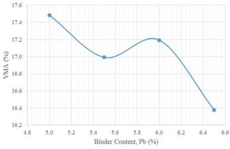
Figure M.5. VMA Results, Granite Mixture
