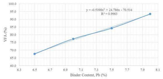
Figure M.1. VFA Results, Limestone Mixture
