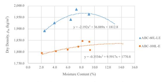
Figure 70. Aggregate Blends Moisture-Density Curves
