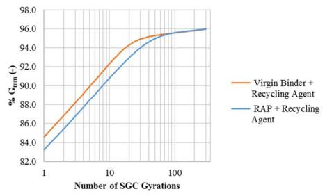
Figure J.4. Recycling Agent P2 Workability Test Results—G<sub>mm</sub> Evolution
