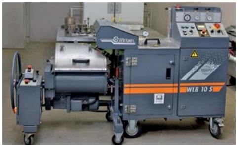
Figure 95. Wirtgen WLB 10S Foaming Unit
