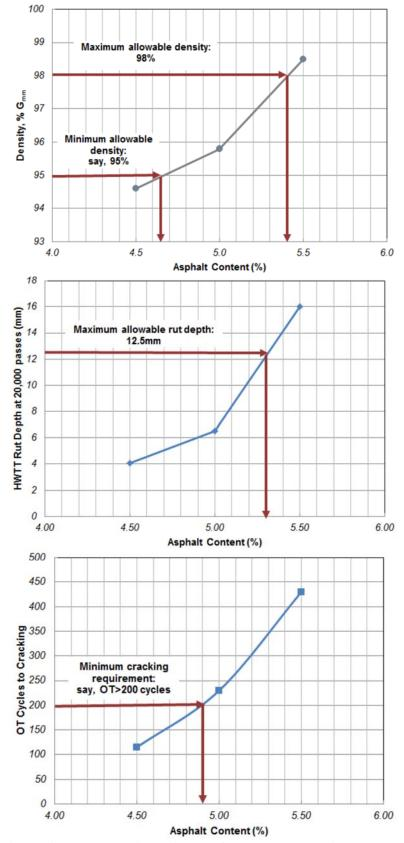
Figure 6. Balanced Mix Design Performance Evaluation Example
