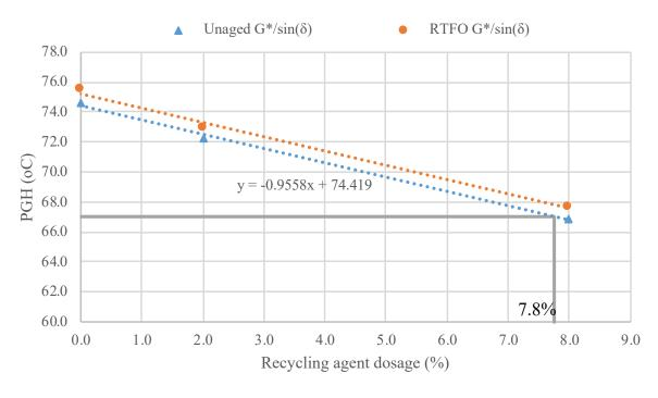
Figure 48. Recycling Agent Dose Verification for Blends with PG 52-28 Virgin Binder + P2 + Extracted and Recovered RAP from Stockpile 1-09
