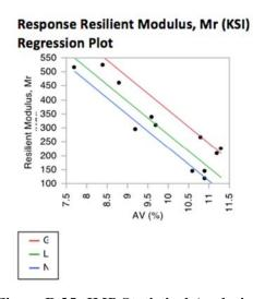
Figure R.35. JMP Statistical Analysis Output with Virgin Aggregate Type, Foamed Cold Recycled Mixtures  $M_R$
