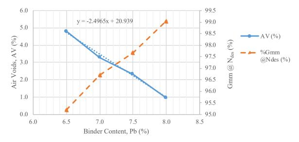
Figure 53. AV Content to Binder Content for the Limestone Virgin Mixture
