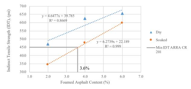
Figure 96. Foamed Cold Recycled Mixture C-60L-LF IDT Strength
