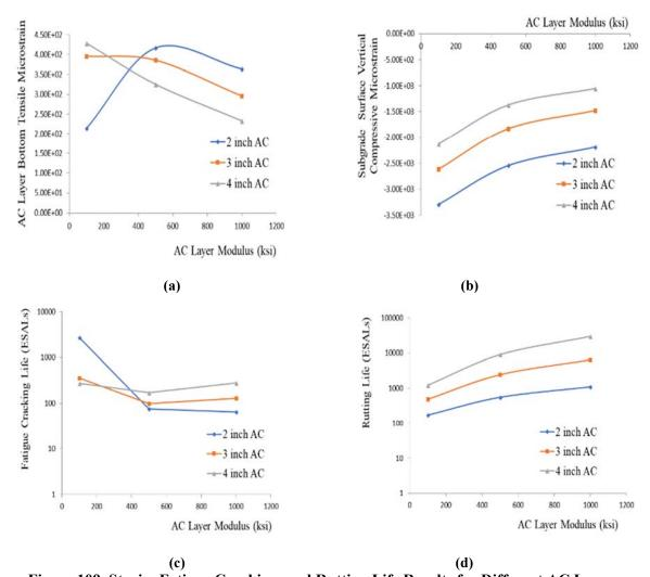
Figure 109. Strain, Fatigue Cracking, and Rutting Life Results for Different AC Layer Thicknesses: (a) AC Bottom Horizontal Strain, (b) Subgrade Surface Vertical Strain, (c) Fatigue Cracking Life, and (d) Rutting Life
