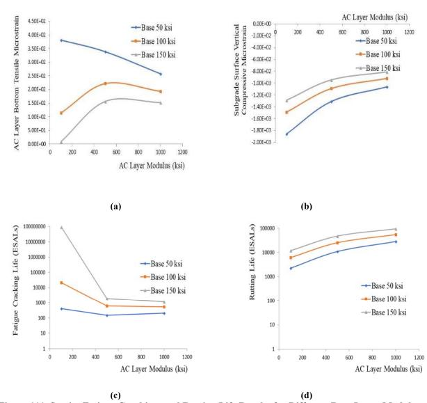
Figure 111. Strain, Fatigue Cracking, and Rutting Life Results for Different Base Layer Modulus: (a) AC Bottom Horizontal Strain, (b) Subgrade Surface Vertical Strain, (c) Fatigue Cracking Life, and (d) Rutting Life
