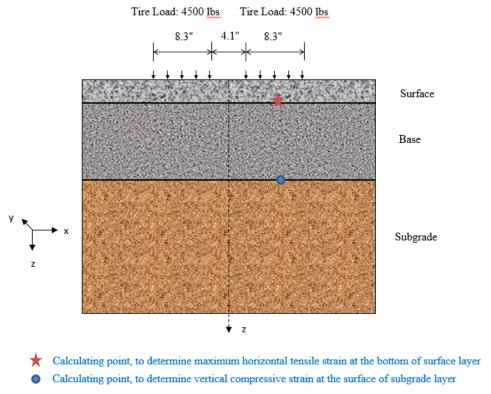
Figure 108. Schematic of the Pavement Structure under Dual-Tire Loading for Multilayer Elastic Analysis Using the BISAR Program
