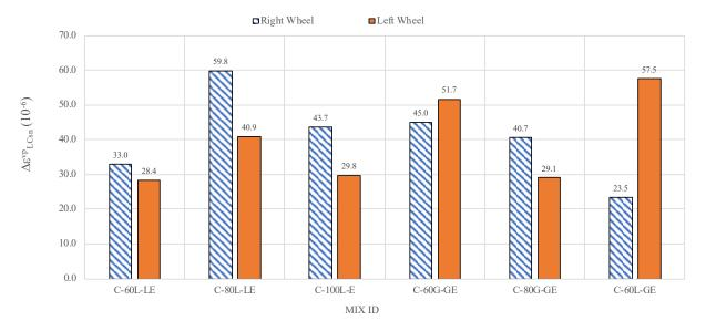
Figure 83. Emulsified Cold Recycled Mixtures' Rutting Resistance Parameter (Δε<sup>νρ</sup><sub>SN</sub>)
