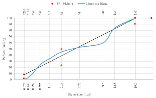
Figure 51. Limestone Aggregate Blend Gradation Curve
