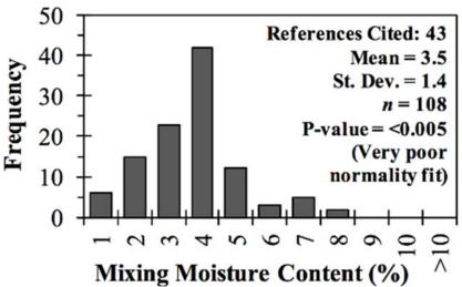
Figure 72. Cold In-Place Mixing Moisture Contents (Cox and Howard, 2015)
