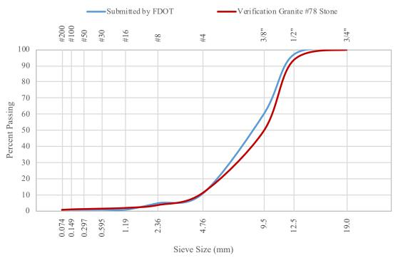
Figure C.3. Gradation Curve, #78 Stone of Granite
