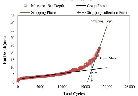
Figure 35. Traditional HWTT Analysis Parameters
