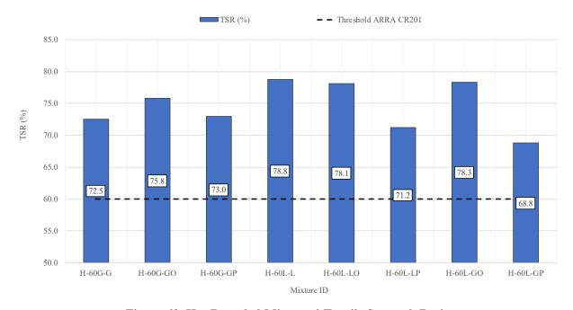
Figure 60. Hot Recycled Mixtures' Tensile Strength Ratio
