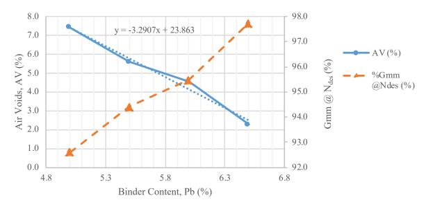
Figure 54. AV Content to Binder Content for the Granite Virgin Mixture
