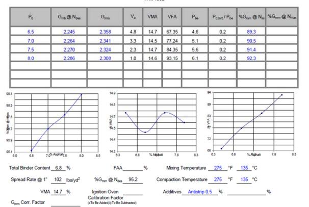
Figure N.2. Mix Design FDOT Format Page 2, Limestone Mixture
