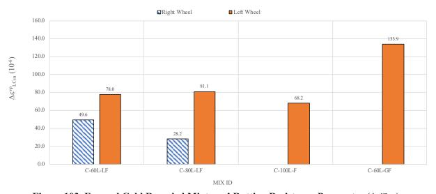
Figure 103. Foamed Cold Recycled Mixtures' Rutting Resistance Parameter (Δε<sup>vp</sup><sub>SN</sub>)
