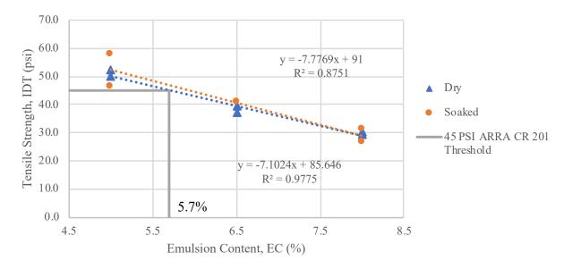
Figure 74. C-100L-E Emulsified Cold Recycled Mixture IDT Strength
