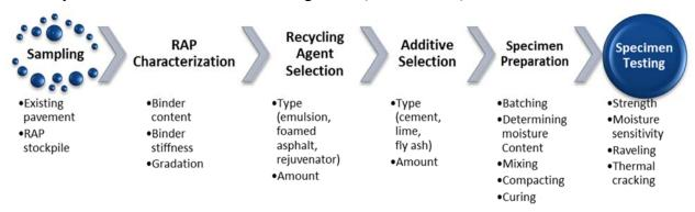
Figure 20. Cold Recycling Mix Design Step
