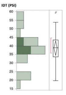
Figure R.24 (Continued). JMP Exploratory Analysis Output, Foamed Cold Recycled Mixtures IDT Strength
