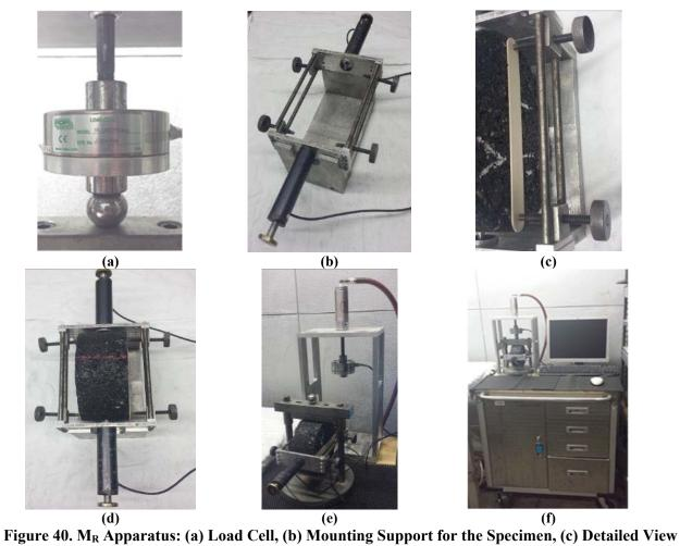
Figure 40. M<sub>R</sub> Apparatus: (a) Load Cell, (b) Mounting Support for the Specimen, (c) Detailed View of Support Pins, (d) Specimen on Mounting Support, (e) Mounting Support and Load Cell Assembly, and (f) Final Test Setup
