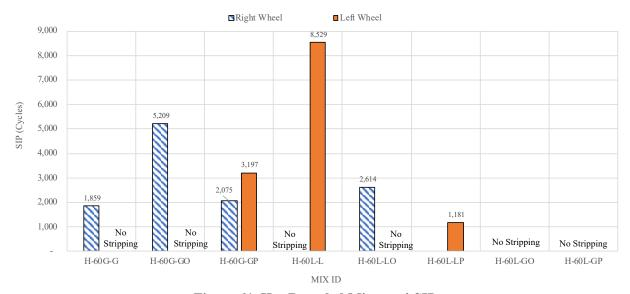
Figure 61. Hot Recycled Mixtures' SIP
