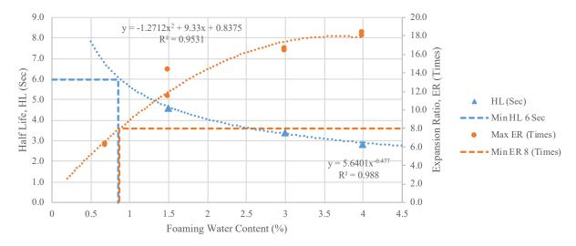
Figure 89. Optimum Foaming Water Content Determination at 338°F (170°C)
