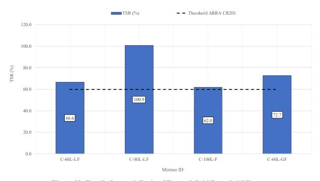
Figure 99. Tensile Strength Ratio of Foamed Cold Recycled Mixtures
