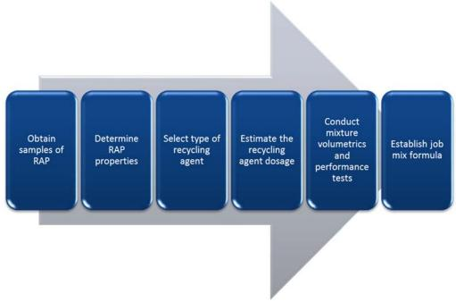
Figure 7. General Mix Design Procedure for Hot Recycling
