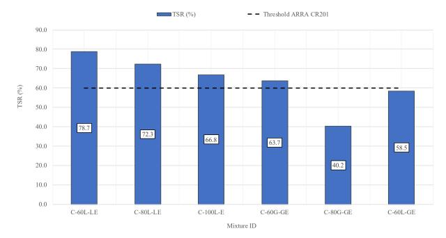
Figure 79. Emulsified Cold Recycled Mixtures' TSR Results
