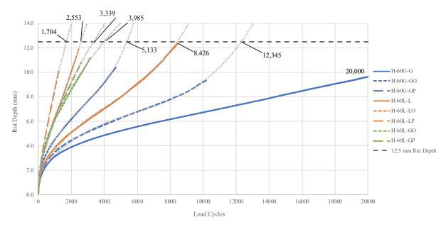
Figure 62. Hot Recycled Mixtures Rut Depth vs. Load Cycles
