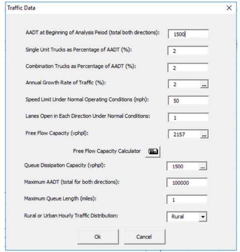
Figure 128. Example of Traffic Data Screen
