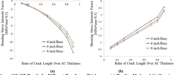
Figure 118. SIF Results for Different Base Layer Thicknesses: (a) Bending Mode and (b) Shearing Mode
