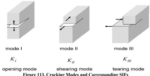
Figure 113. Cracking Modes and Corresponding SIFs
