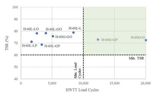
Figure 140. HWTT Load Cycles to Failure and TSR, Hot Recycling
