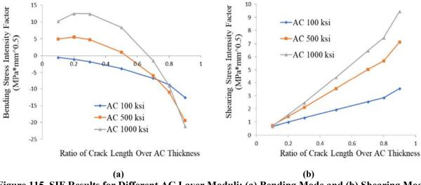
Figure 115. SIF Results for Different AC Layer Moduli: (a) Bending Mode and (b) Shearing Mode
