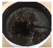
Figure K.4. Emulsion Sediment in Good Condition
