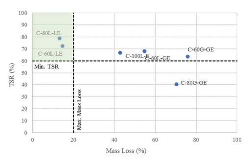
Figure 144. Cantabro Mass Loss and TSR, Cold Recycling—Emulsion
