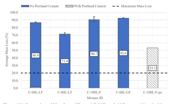
Figure 106. Comparison of Mass Loss of Foamed Cold Recycled Mixtures with and without Portland Cement
