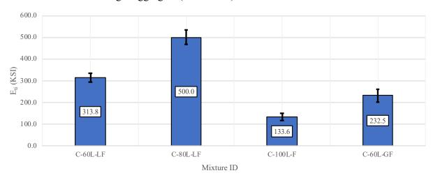
Figure 107. Foamed Cold Recycled M<sub>R</sub> Results
