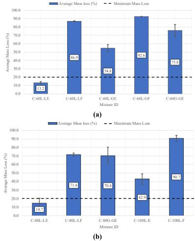
Figure 137. Cantabro Abrasion Mass Loss Comparison
