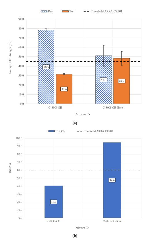
Figure 80. C-80G-GE Mixture Results with and without Hydrated Lime: (a) IDT Strength, and (b) TSR
