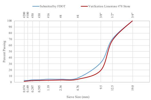
Figure C.1. Gradation Curve, #78 Stone of Limestone
