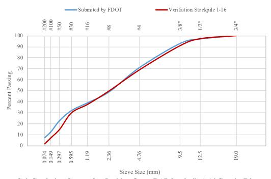
Figure C.6. Gradation Curve after Ignition Oven, RAP Stockpile 1-16 Granite/Limestone
