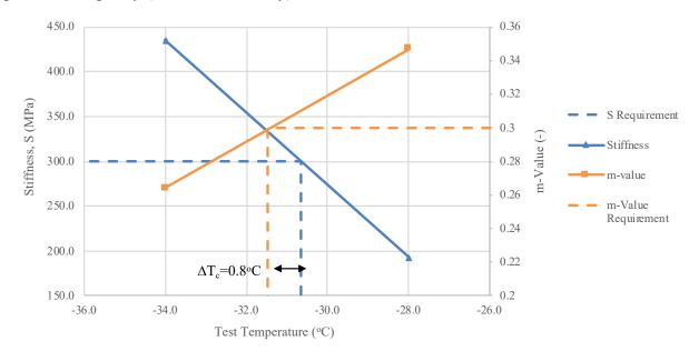
Figure 41. PG 52-28 ΔT<sub>c</sub> Parameter Estimation
