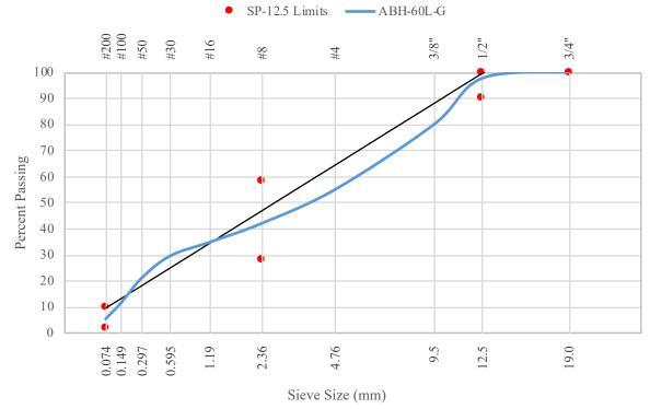
Figure 58. ABH-60L-G Aggregate Blend Gradation Curve
