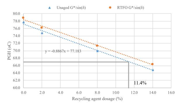
Figure 50. Recycling Agent Dose Verification for Blends with PG 52-28 Virgin Binder + P2 + Extracted and Recovered RAP Stockpile 1-16
