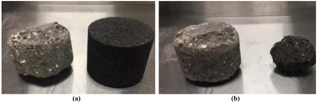
Figure 85. Cantabro Abrasion Loss Specimens: (a) Mixture C-60L-LE before (right) and after (left) Testing, and (b) Mixture C-60L-LE after Testing (left) and Mixture C-60G-GE after Testing (right)
