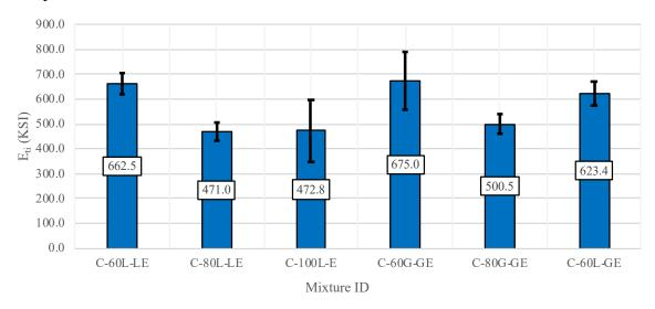
Figure 86. Emulsified Cold Recycled M<sub>R</sub> Results
