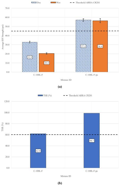
Figure 100. C-100L-F with and without Portland Cement: (a) IDT Strength and (b) TSR.
