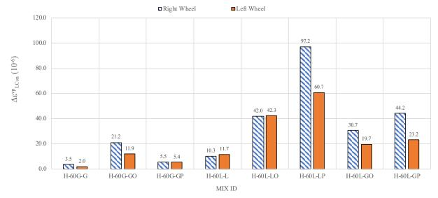
Figure 63. Hot Recycled Mixtures Rutting Resistance Parameter ( $\Delta \varepsilon^{vp}_{SN}$ )
