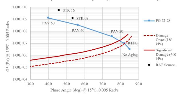
Figure 42. Aging Evaluation of Binder PG 52-28 in Black Space Diagram
