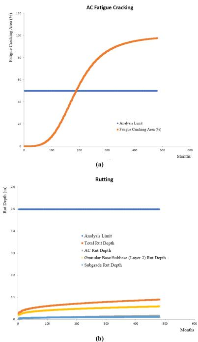
Figure 124. TxME Output for Case 1: (a) Fatigue Cracking Model Prediction Result and (b) Rutting Model Prediction Result
