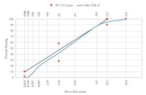
Figure 67. Emulsified Cold Recycled Mixtures ABC-100L-E Aggregate Blend Gradation Curve
