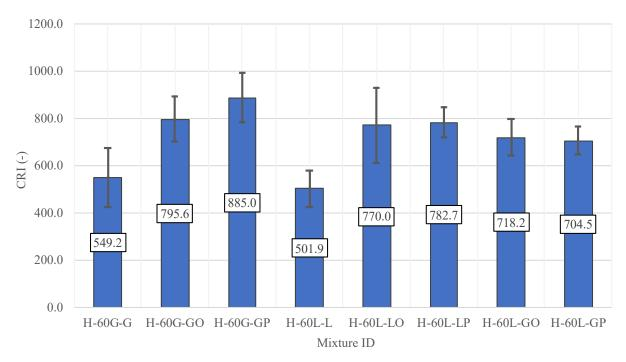
Figure 65. Hot Recycled Mixtures' CRI
