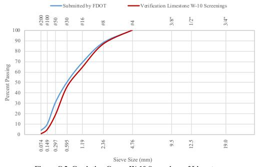
Figure C.2. Gradation Curve, W-10 Screenings of Limestone
