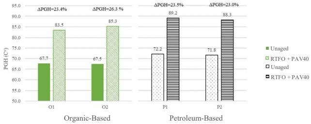
Figure 44. Change in PGH with Aging for Blends with PG 52-28 Virgin Binder + Extracted and Recovered RAP from Stockpile 1-16
