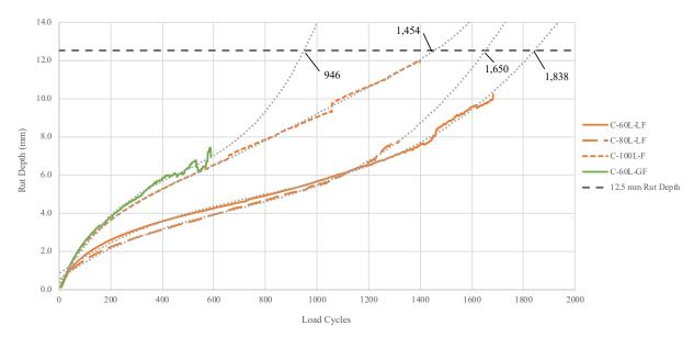
Figure 102. Foamed Cold Recycled Mixtures' Rut Depth vs. Load Cycles
