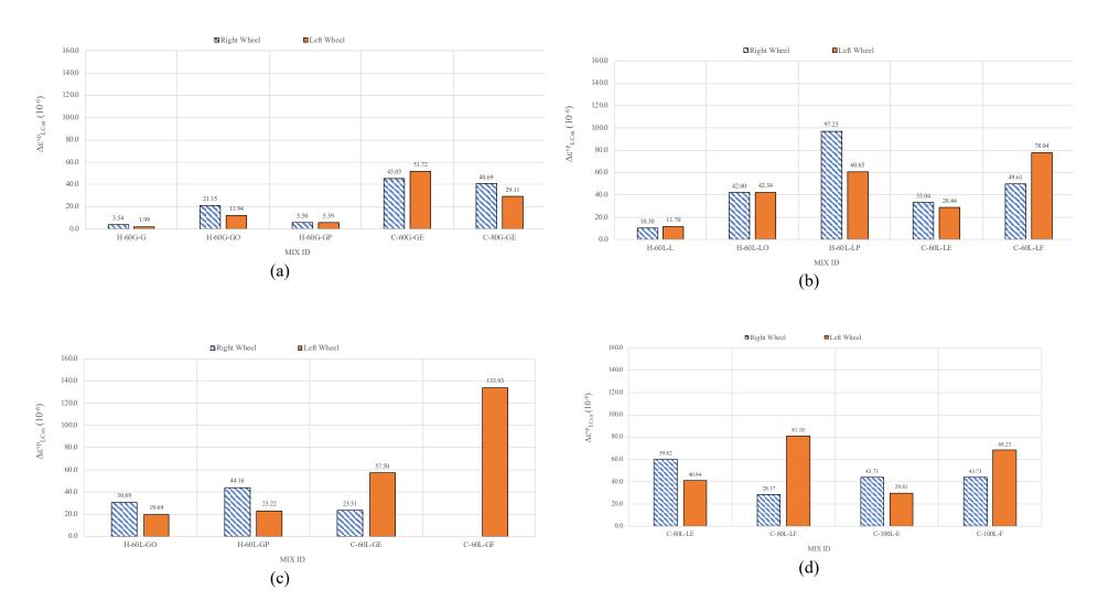
Figure 136. Rutting Resistance Parameter (Δε<sup>vp</sup><sub>SN</sub>) Comparison
