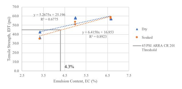
Figure 76. C-60G-GE Emulsified Cold Recycled Mixture IDT Strength
