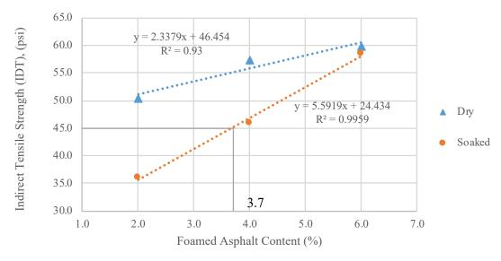
Figure 97. Foamed Cold Recycled Mixture C-60L-GF IDT Strength
