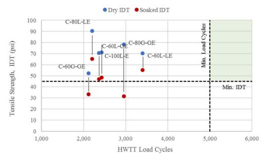
Figure 142. HWTT Load Cycles to Failure and IDT, Cold Recycling—Emulsion
