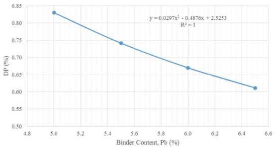
Figure M.6. DP Results, Granite Mixture
