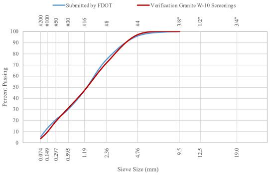
Figure C.4. Gradation Curve, W-10 Screenings of Granite
