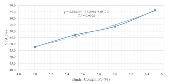
Figure M.4. VFA Results, Granite Mixture
