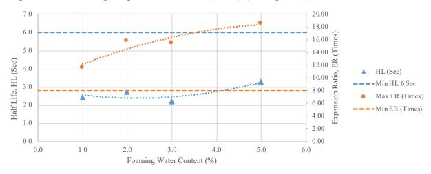
Figure 88. Optimum Foaming Water Content Determination at 320°F (160°C)
