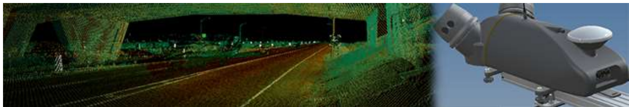
Figure 10. A LiDAR survey of a highway (left), and a LiDAR antenna (right)
