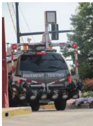
Figure 3. Road survey vehicle equipped with constant lighting
