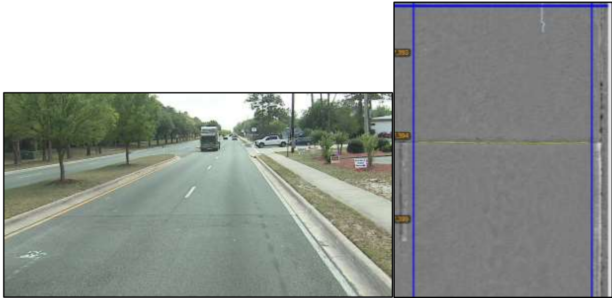
Figure 221. Patching Area Boundary Falsely Detected as Cracks
