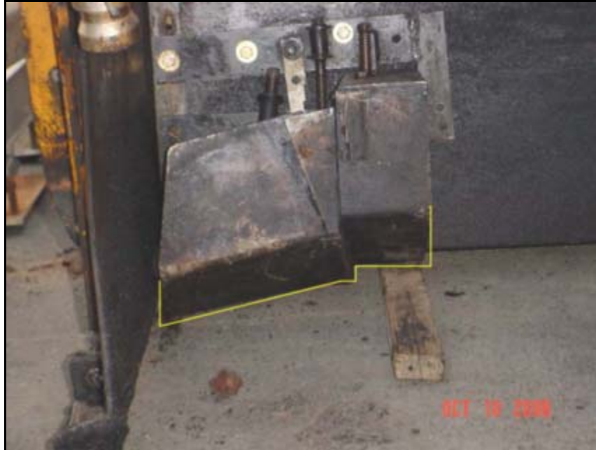
Figure 2. Notched wedge forming device.
