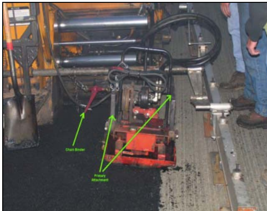
Figure 3. Wedge compaction device.
