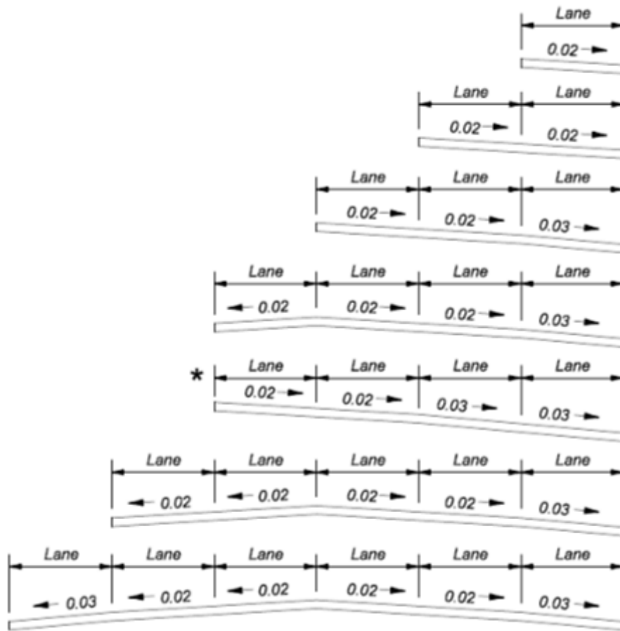
Figure 40. Standard FDOT freeway cross slopes.
