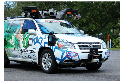
This experimental vehicle is part of a FDOT initiative to test CAV technologies. Components, such as sensors and communication devices, normally built in a vehicle, are exposed for testing purposes.
