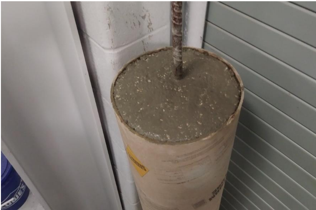
Figure 22. Example rebar-in-concrete experimental set-up.
