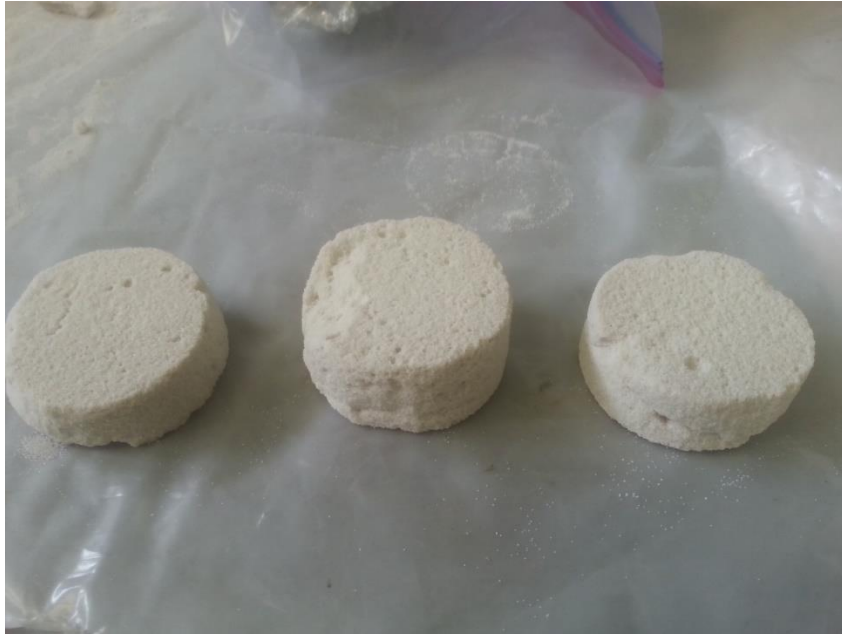
Figure 2-18. DST samples from varied height intervals from the bottom of the specimen
