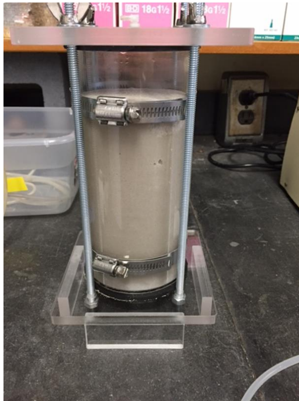
Figure 2-4. Traditional treatment chamber filled with Ottawa 50-70 sand
