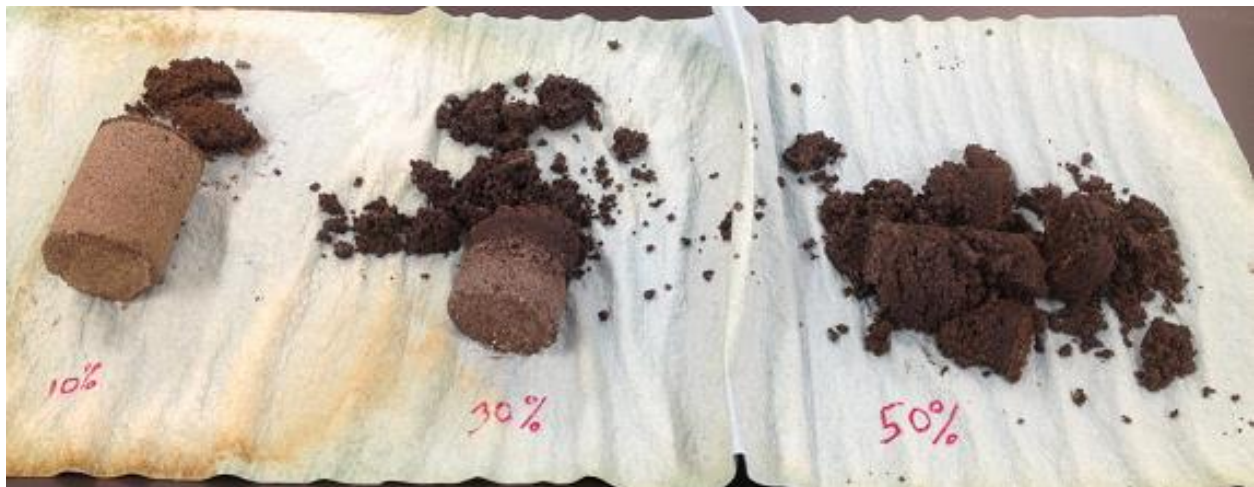
Figure 4-2. Typical results using pre-mixing MICP treatment in organic-rich specimens from Polk County, FL
