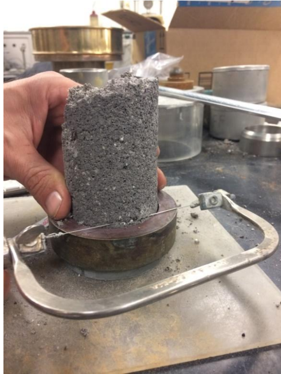
Figure 4-12. Careful trimming of sample into oedometer ring using a saw
