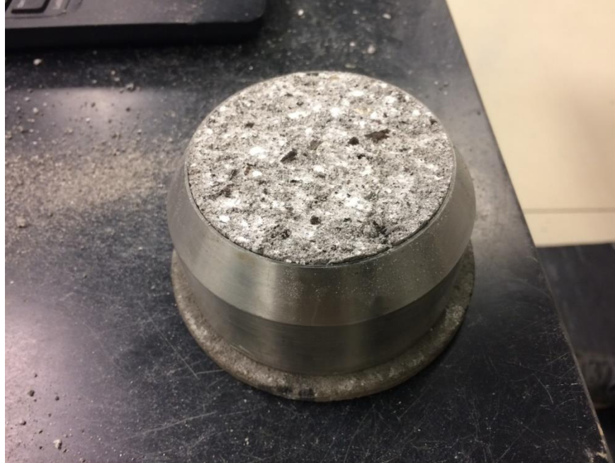
Figure 4-14. 2.8-inch diameter oedometer ring filled with treated soil
