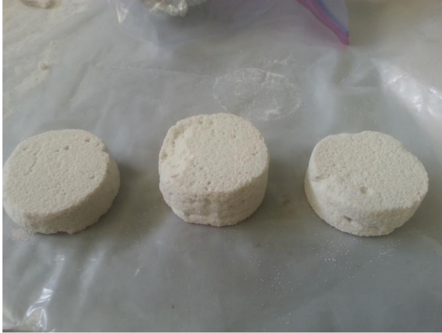
Figure 2-9. Treated percolation-treated sand samples prepared for DST
