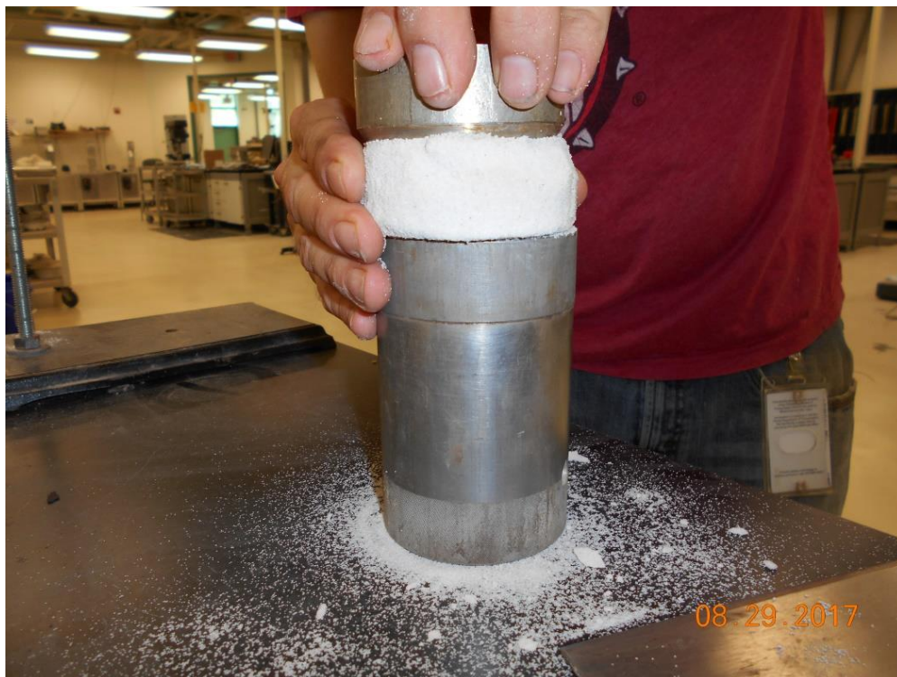
Figure 2-11. Careful trimming of calcified sand into oedometer ring
