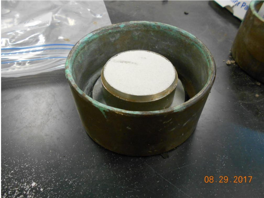
Figure 2-12. Calcified sand in ring after trimming
