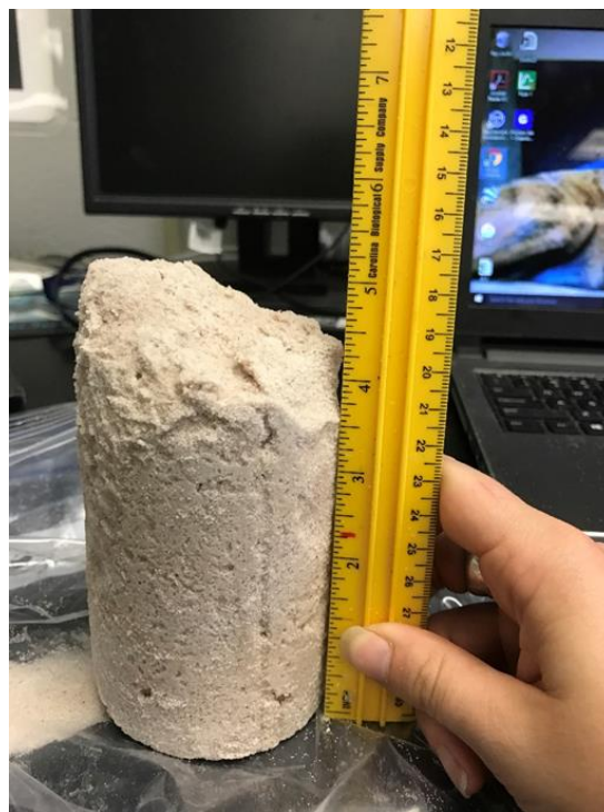
Figure 2-17. Example of fully cemented soil column
