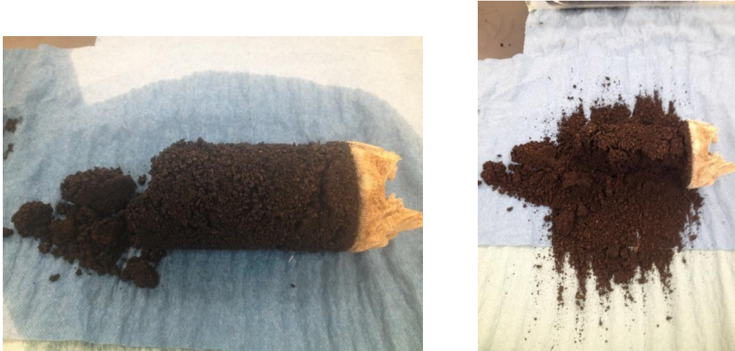
Figure 3-18. Typical organic-rich specimen after MICP treatment using the percolation method showing specimen immediately after extraction (left) and specimen after drying (right)
