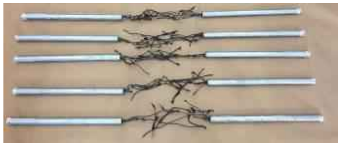
Figure 3.11: Typical failure mode of CFRP tension specimens (NCSU)
