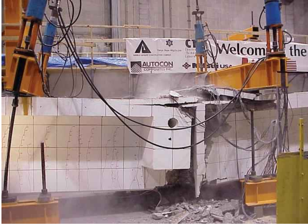
Figure 2.23: Failure of DT girder due to separation of concrete topping and crushing of concrete (Grace et al. 2003).
