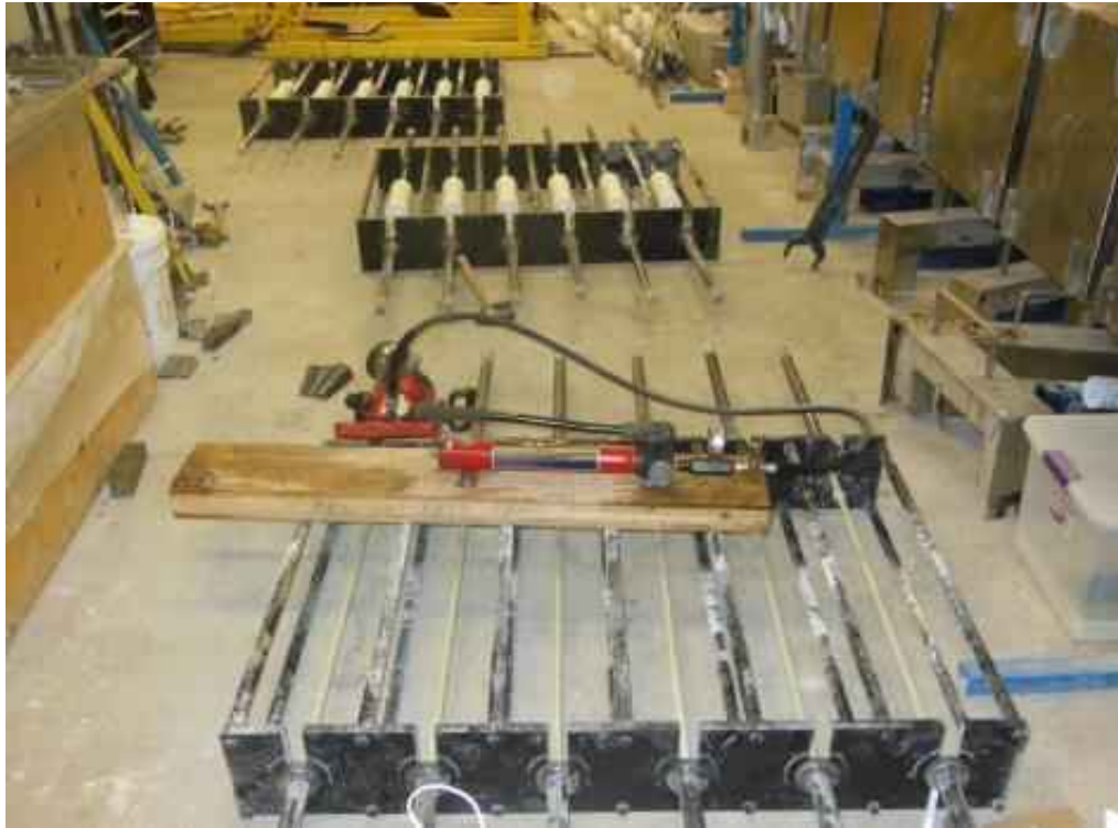
Figure 4.9: Test setup of stressed GFRP bars during the installation
