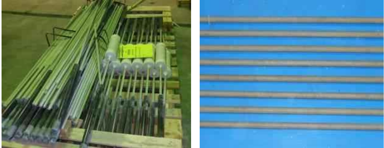
Figure 4.1: Pultrall GFRP bars as received (GFRP #5)
