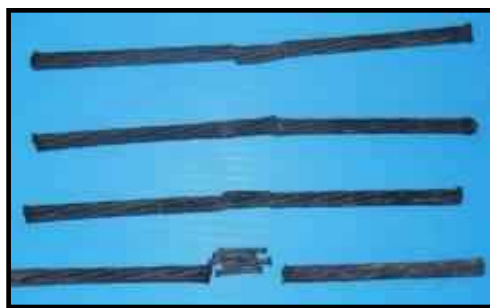
Figure 3.32: Typical shear failure of CFRP specimens
