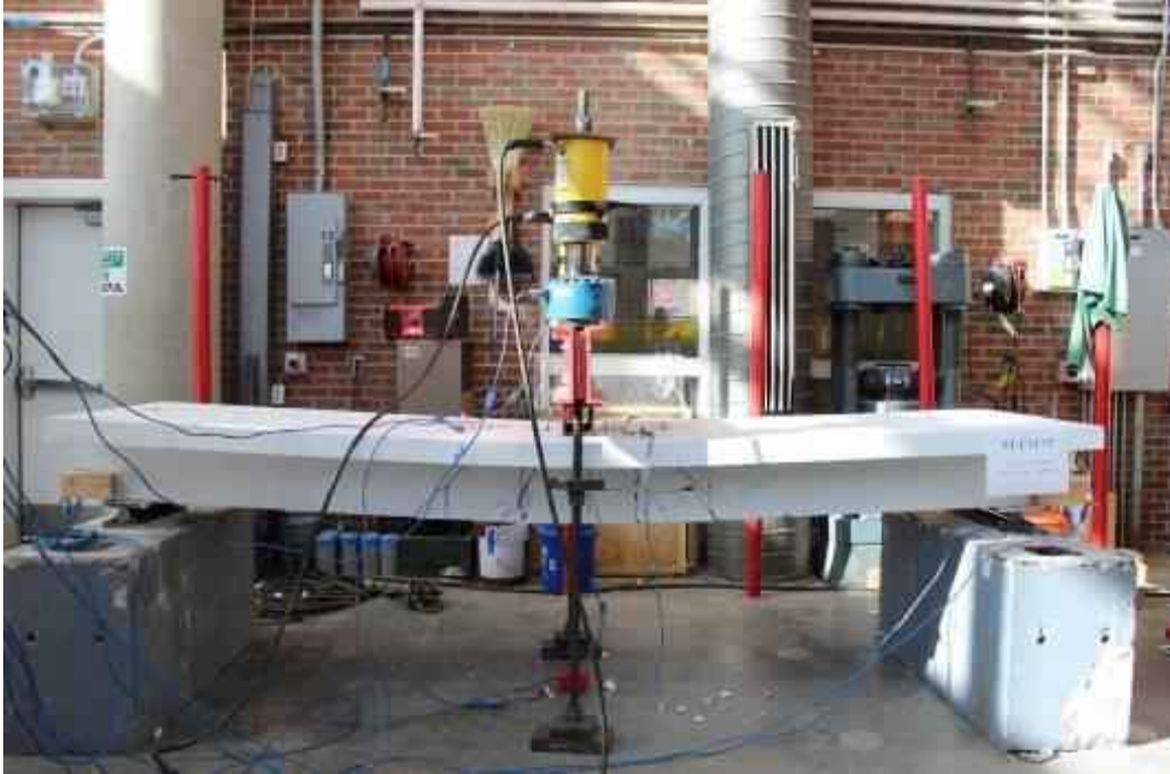
Figure 6.30: Failure of beam#9 after 18 months of exposure (Top Beam).
