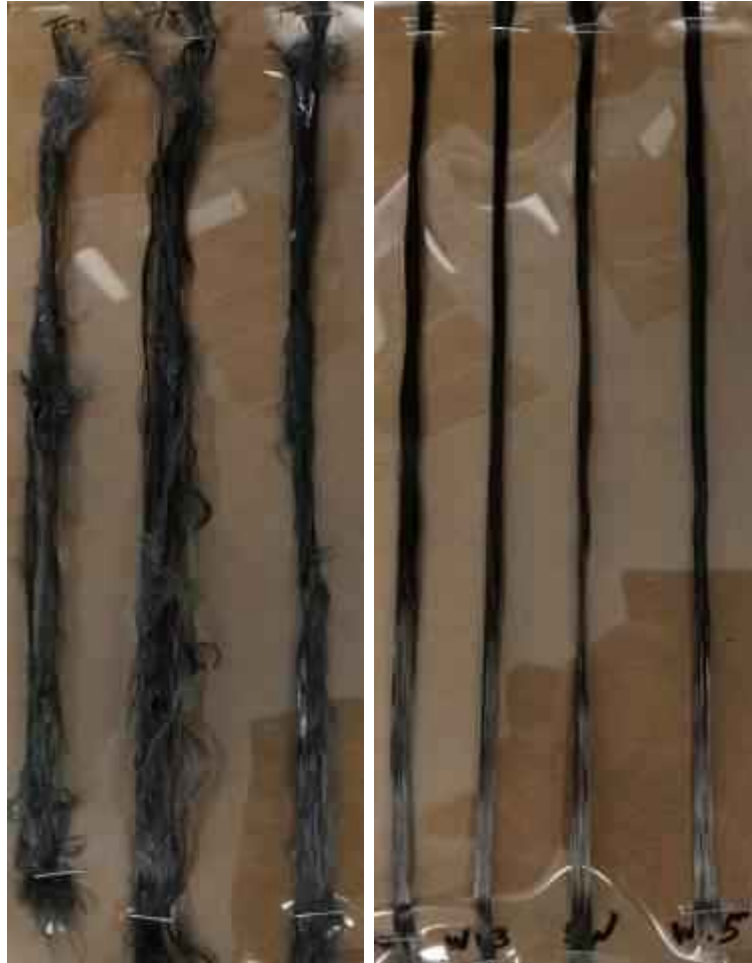
Figure 5.8: Comparison between specimens exposed to alkaline solution (left) and water (right).
