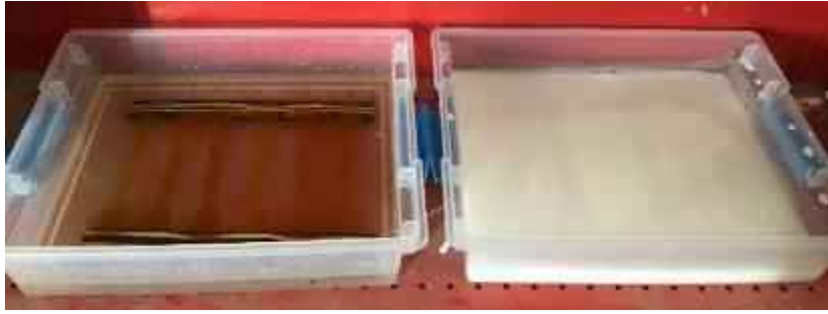
Figure 5.11: Epoxy resin specimens undergoing conditioning at room temperature.
