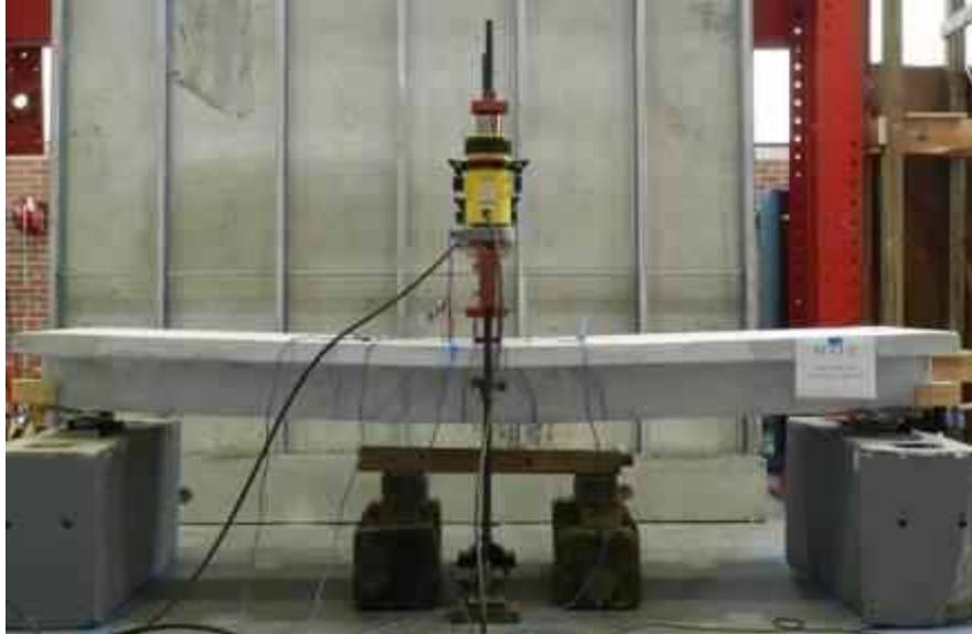
Figure 6.20: Failure of beam#4 after 3 months of exposure (Bottom Beam).
