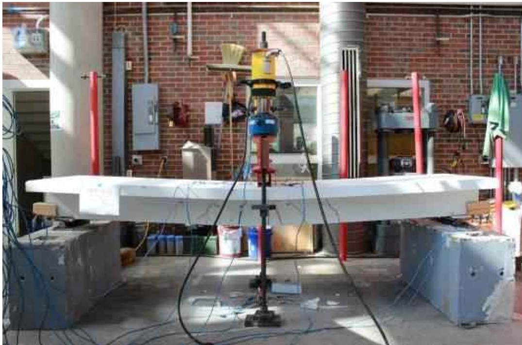
Figure 6.35: Failure of Beam#12 after exposure to sustained load for 18 months (Bottom Beam)
