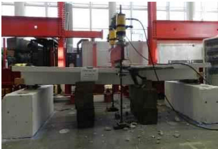
Figure 6.16: Failure of control beam#2
