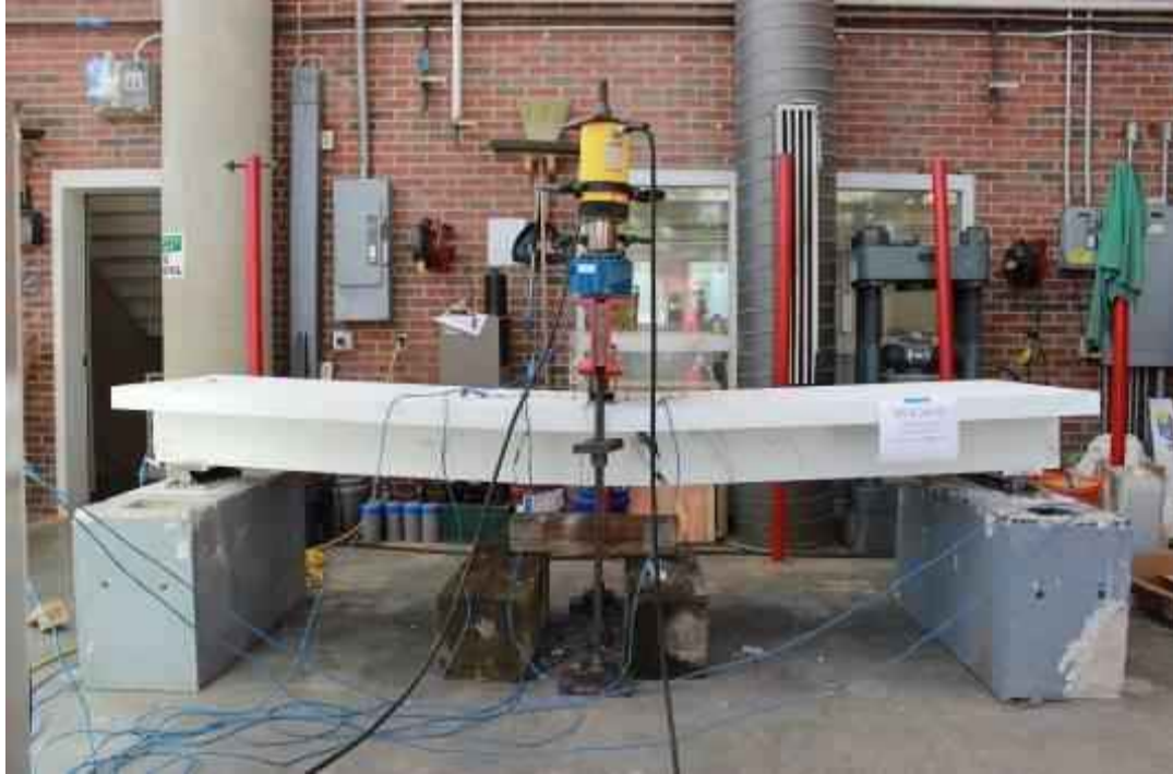
Figure 6.34: Failure of Beam#11 after exposure to sustained load for 18 months (Top Beam)
