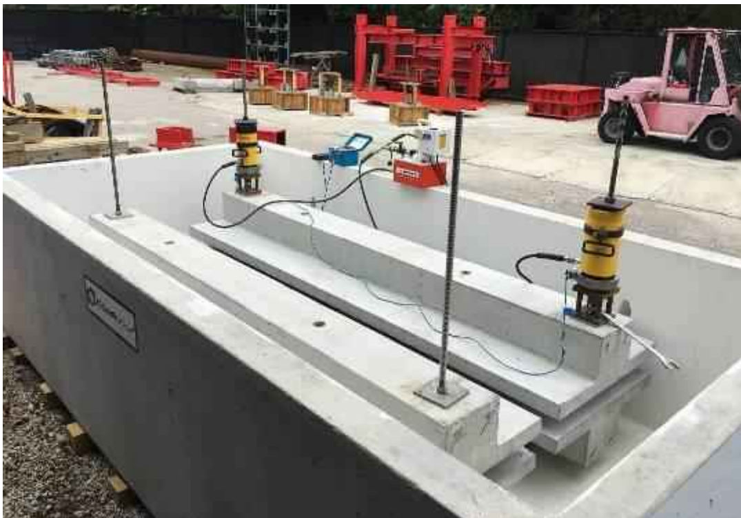
Figure 6.11: Concrete beams in first tank subjected to sustained load.
