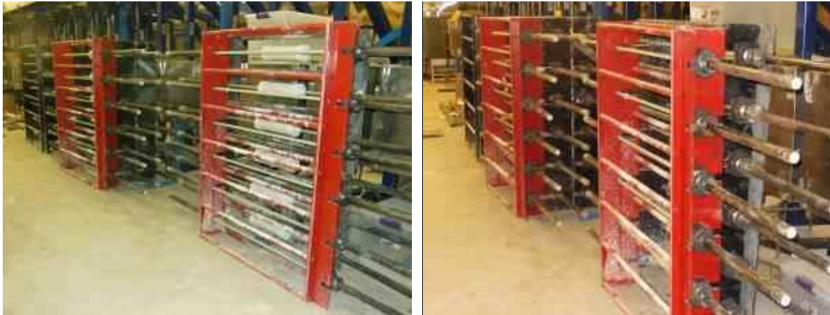
Figure 4.10: GFRP stressed specimens (with 30% of loading) with sustained creep load frame
