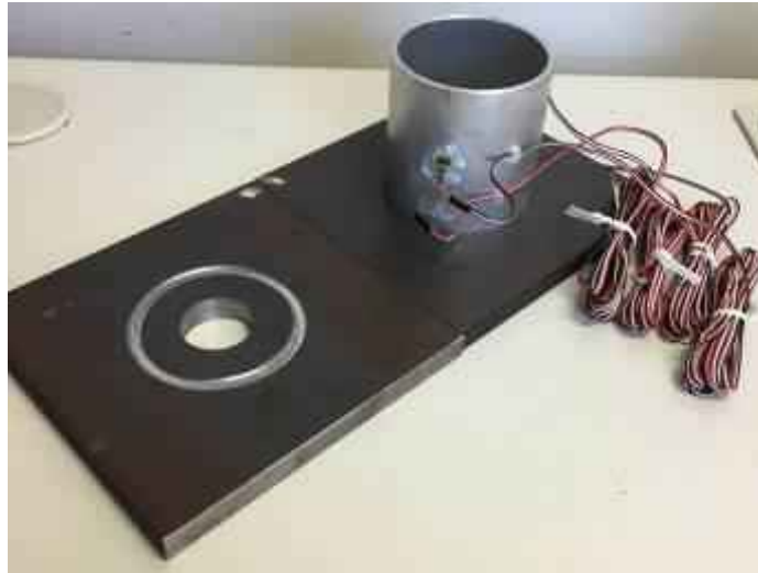
Figure 3.19: Manufactured load cell used at dead end of tensioning
