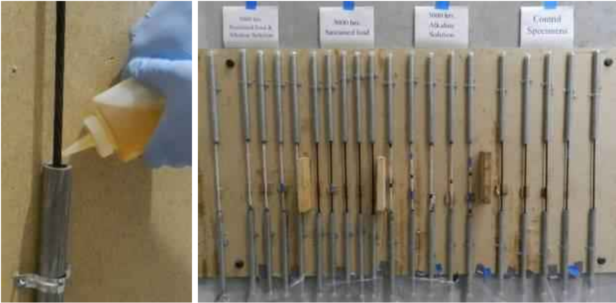
Figure 3.9: Preparation and curing of anchorages at NCSU
