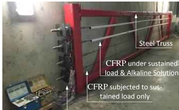
Figure 3.20: Steel truss with 4 tensioned CFRP tendons
