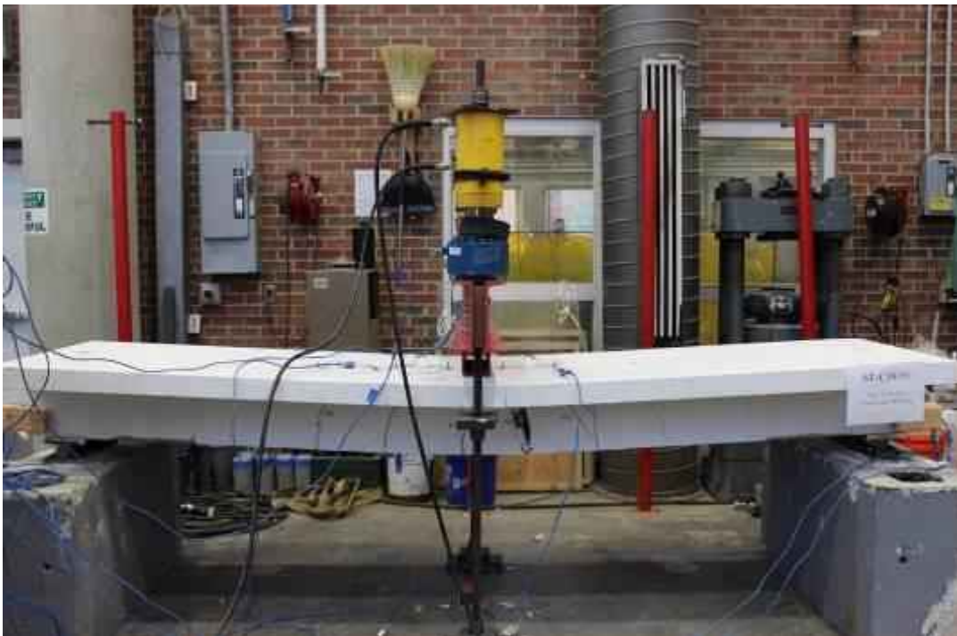
Figure 6.31: Failure of beam#10 after 18 months of exposure (Bottom Beam).
