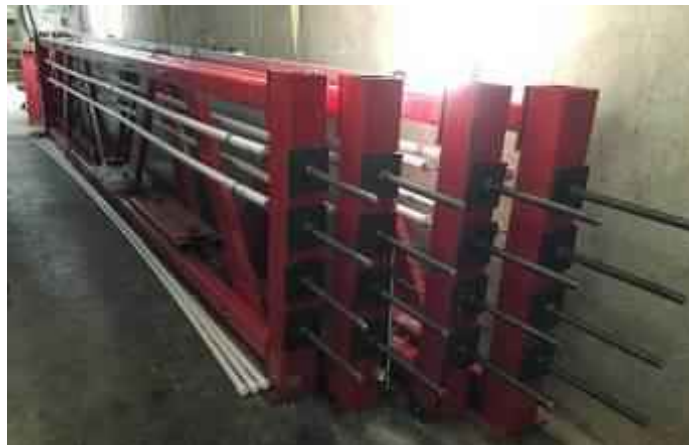
Figure 3.21: Four steel trusses with 16 CFRP tendons under sustained load and environmental exposure
