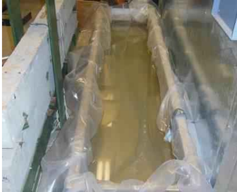
(a) GFRP specimens (without load) in environmental chamber at 22°C [72°F]
