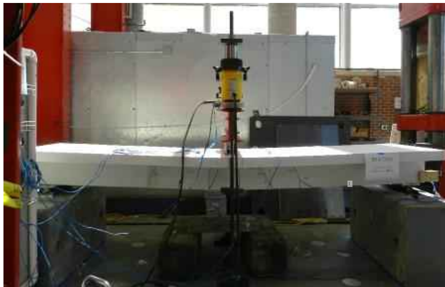
Figure 6.27: Failure of beam#7 after 12 months of exposure (Top Beam).
