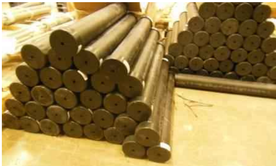
Figure 3.13: The PVC tubes used for CFRP specimens subjected to sustained load and alkaline solution
