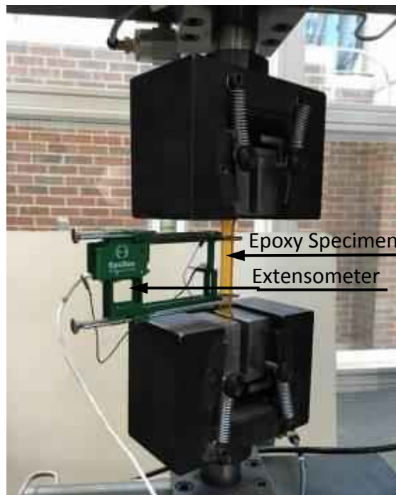
Figure 5.12: Epoxy coupon during testing.
