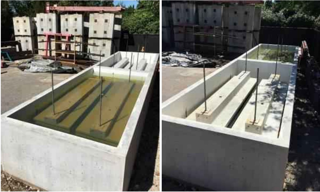
Figure 6.12: Concrete beams in two tanks undergoing wet and dry cycles
