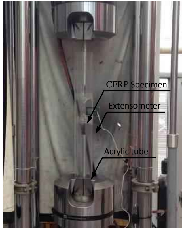
Figure 3.10: Tensile test of CFRP specimen at NCSU
