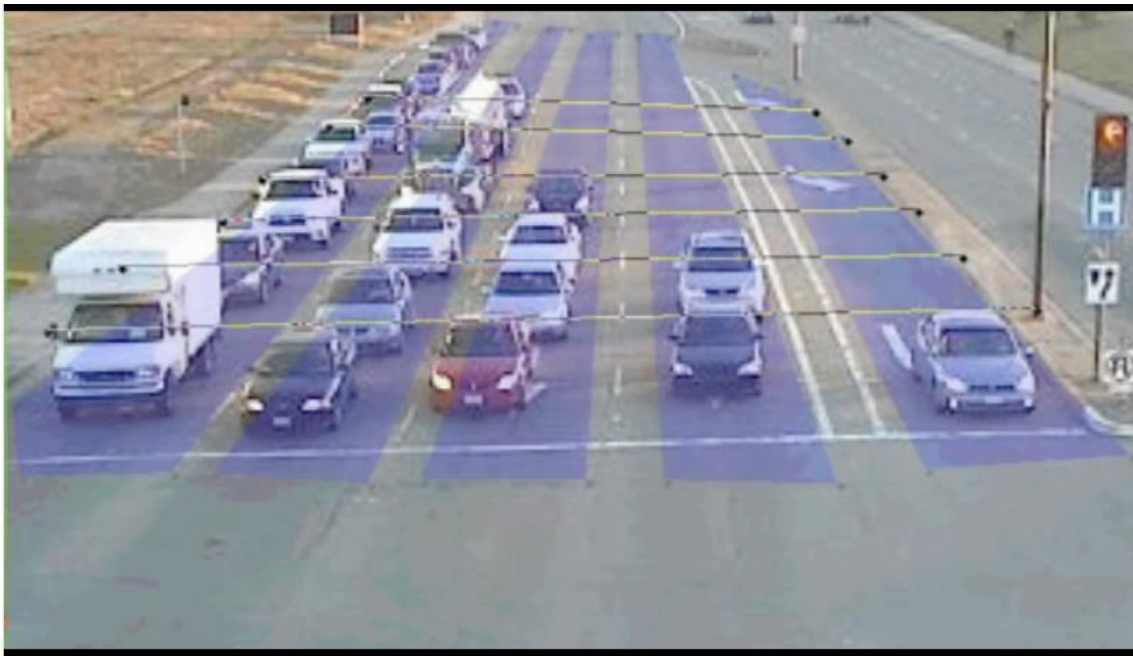
Figure 2.2 InSync cameras detection through image processing [6]
