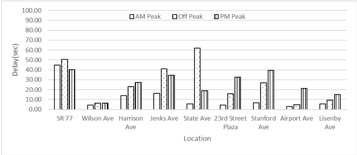
Figure E-2.4 Delay (sec) for each Intersection Through Movement Along the WB Direction
