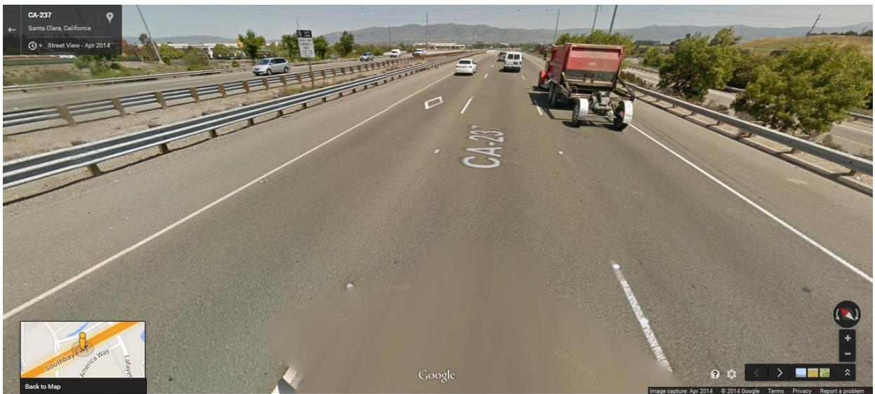
**Figure 3.6 California Painted Stripe Separation on SR-237**
