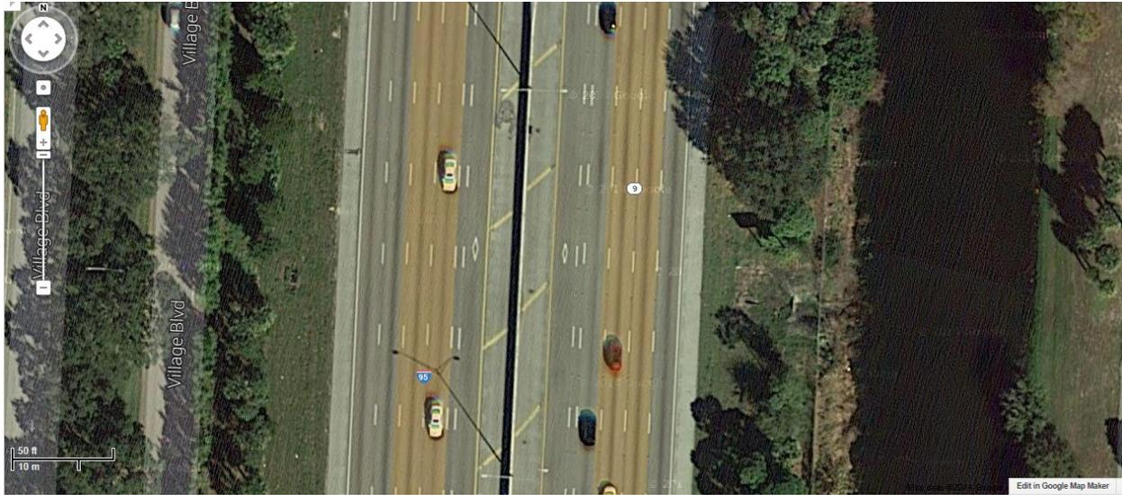
**Figure 3.10 Florida Buffer Separation on I-95**
