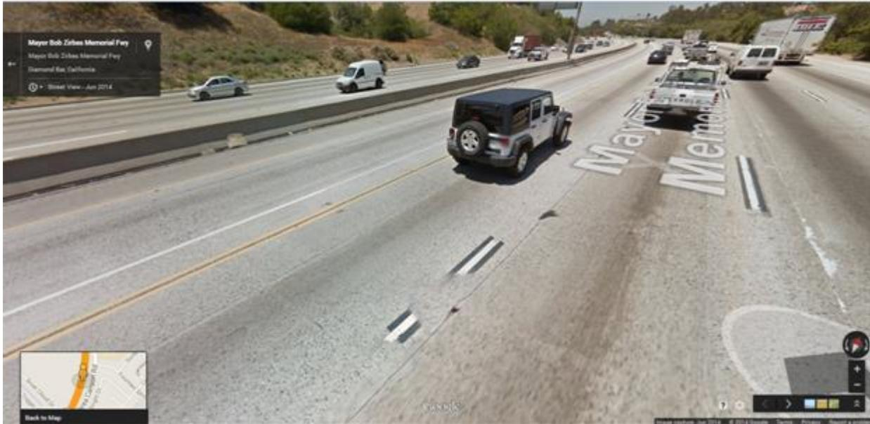
**Figure 3.3 California Buffer Separation on SR-57 (Buffer of 2-3 feet)**
