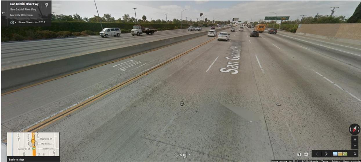
**Figure 3.1 California Buffer Separation on I-605 (Buffer of less than 1 foot)**
