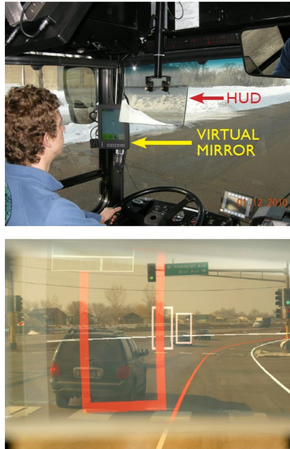
Figure 2-1 – Driver assistance system for driving on shoulders; HUD: heads-up display (Pessaro and Van Nostrand, 2011)
