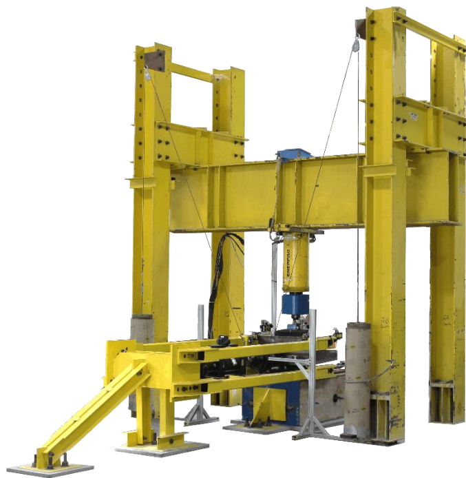
Figure 4-7 Completed bearing pad test setup (FDOT Structures Research Center, Tallahassee, Florida)
