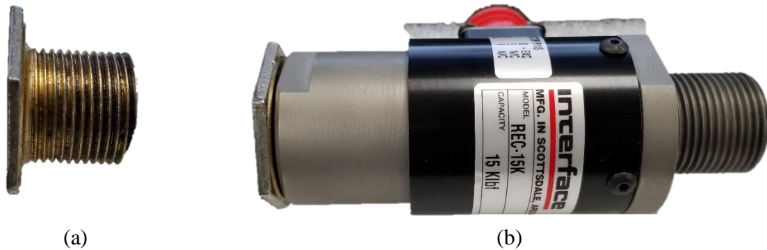
Figure B-15 Rod end compression cell assembly: (a) 1 in. diameter 1 in. length bolt with reduce head thickness; (b) REC cell with bolt
