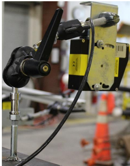
Figure B-19 Typical metal stud used for mounting DZ laser gauges
