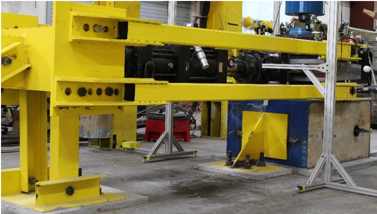
Figure B-11 HSS arms installed in the setup
