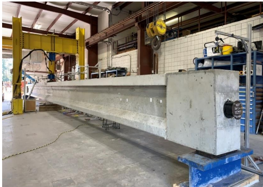
Figure C.16 Beam specimen SS-2 inside test frame
