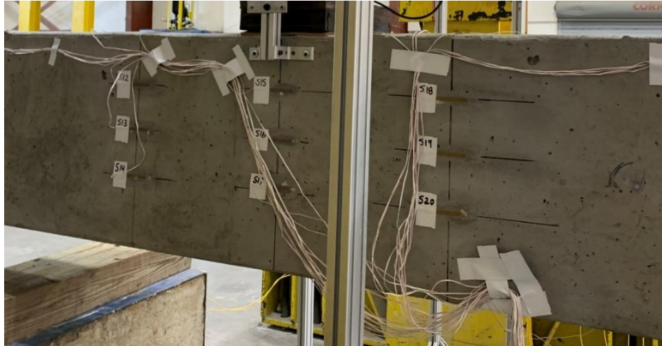
Figure 6.8 60-mm foil strain gages installed on CIP beam specimen SS-5
