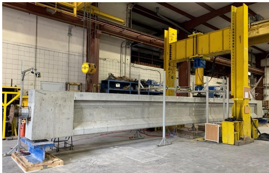
Figure C.27 Beam specimen SS-3 inside test frame
