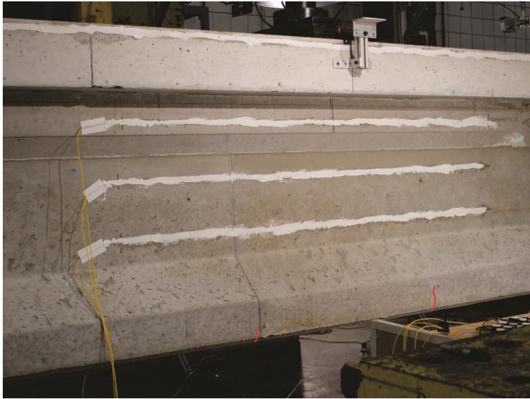
Figure C.17 Specimen SS-2: first observed cracks (marked in red) at P = 77 kip on east side
