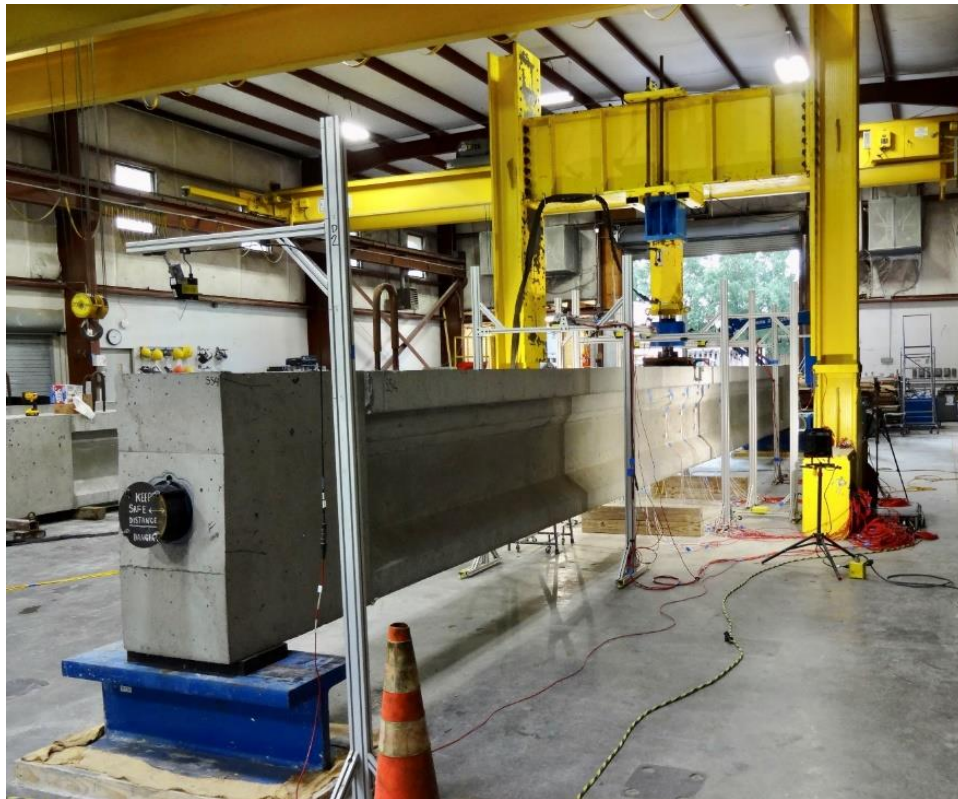
Figure C.38 Beam specimen SS-4 inside test frame
