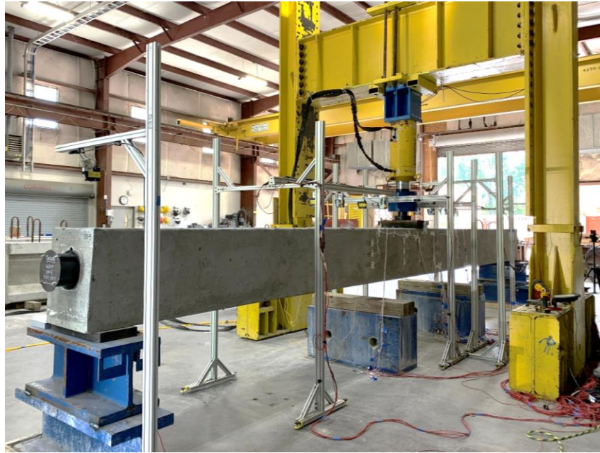
Figure D.5 Beam specimen SS-5 inside test frame
