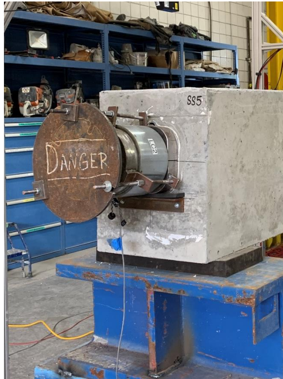
Figure 6.5 Geokon hollow-core load cell installed at dead end of beam specimen SS-5
