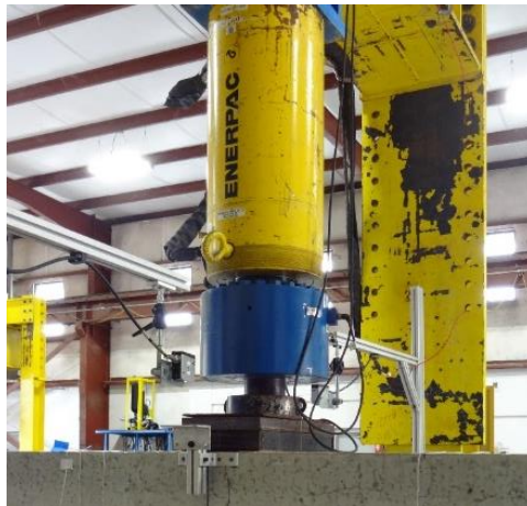
Figure 5.26 Enerpac RR-40018 actuator
