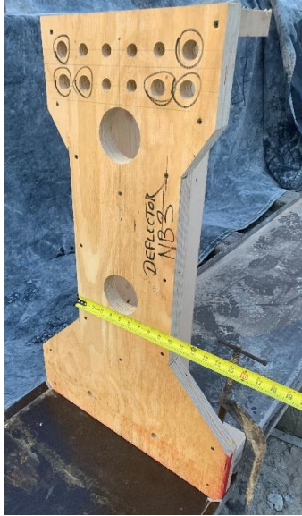
Figure 7.4 Plywood bulkhead for prestressing strands on NB specimens
