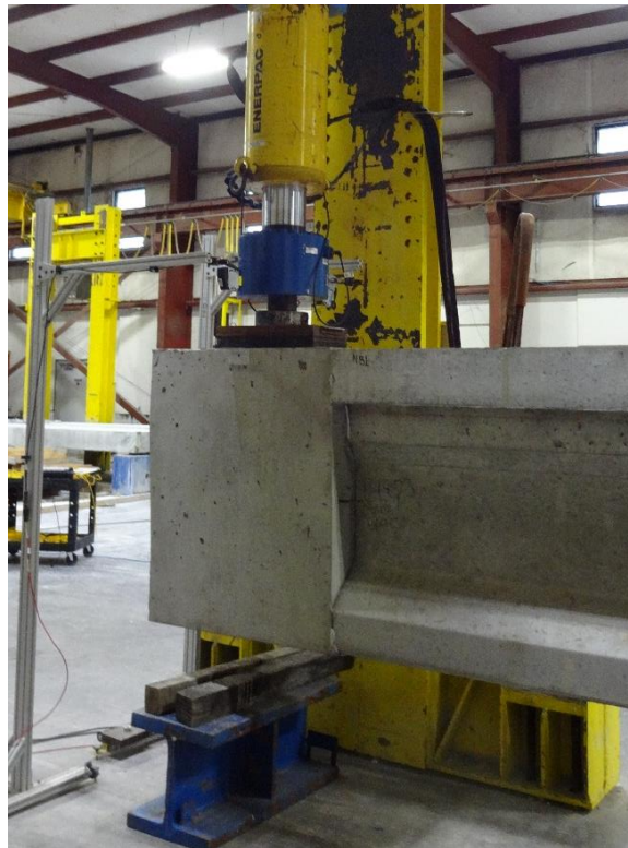
Figure E.7 Beam specimen NB-1: load point
