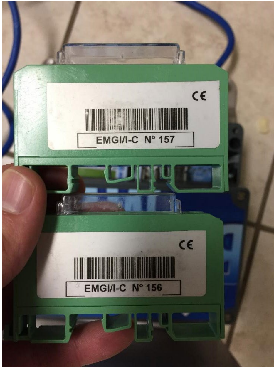
Figure 2-5. Copy modules used to route torque and crowd readings to both systems.
