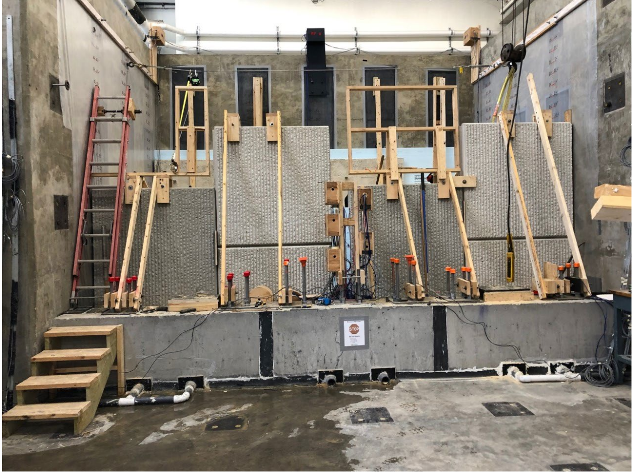
Figure 4-29. Adding the second course of MSE wall panels.
