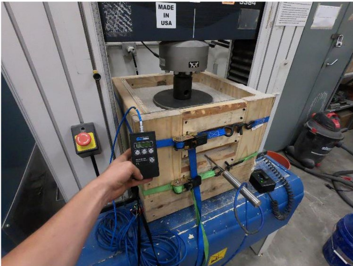
Figure 4-42. Load testing a soil embedded EPC for calibration.
