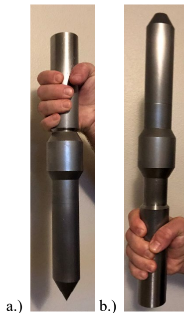
Figure 3-2. O-ring compression hand calibration procedure displaying a.) the probe remaining closed supporting its own weight and b.) the probe remaining open supporting its own weight.
