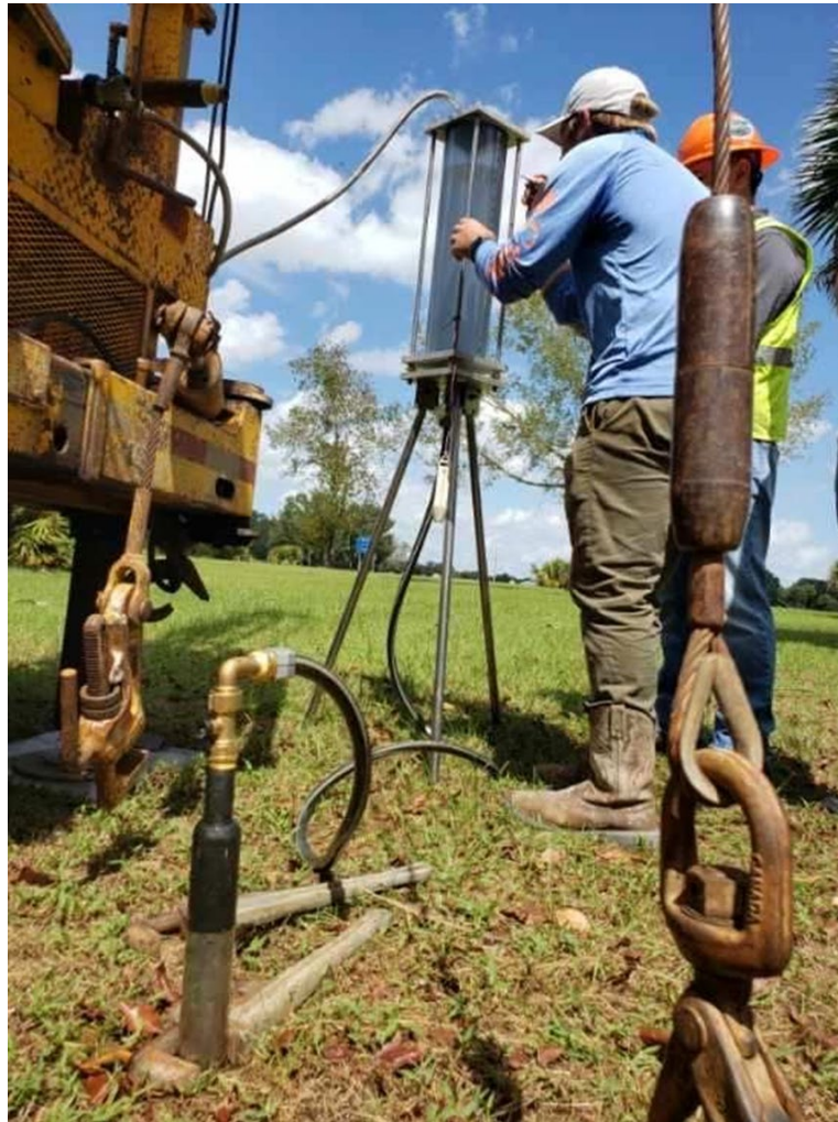
Figure 5-29. VIP being used for an infiltrometer tests.
