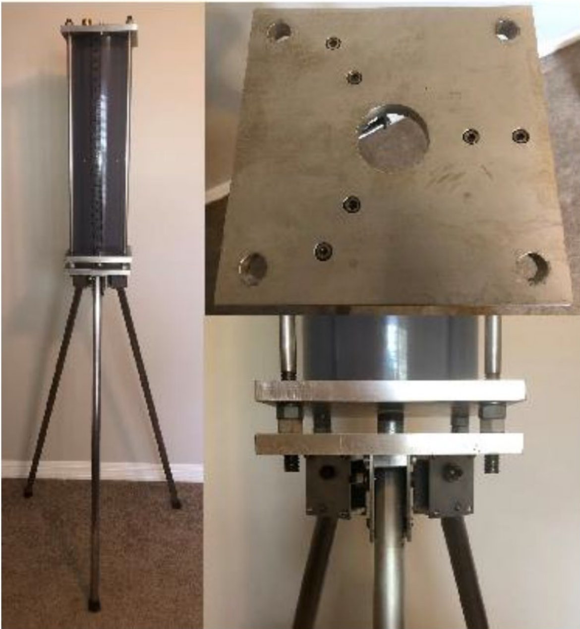
Figure 2-11. New falling head vessel design, displaying removable pieces.
