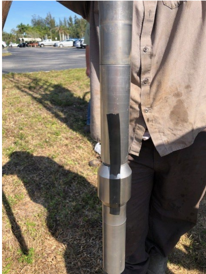
Figure 5-23. VIP probe with electric tape to ensure closed position for open-hole advancement.
