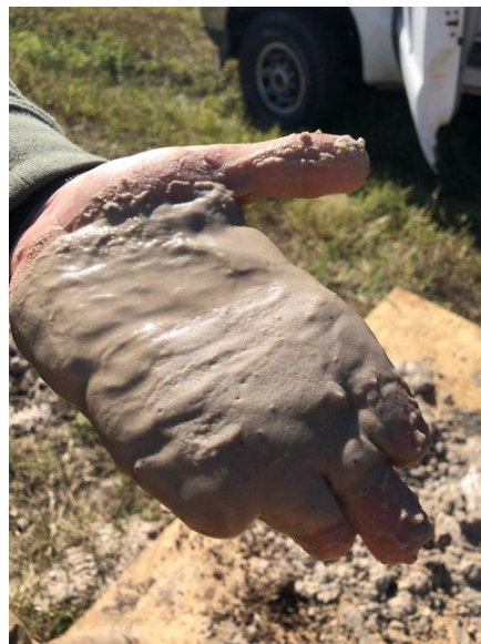
Figure 5-43. Fine grained soil recovered by a hand auger at the Veterans Expressway site.
