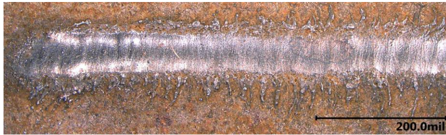
Figure 3-10. HAZ depth trails off as mark continues (above) and associated distances (below). Marked at 15 A and 250 in/min
