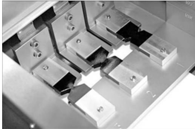
Figure 2-18. DENT samples placed on loading pins (AASHTO TP113-2015)
