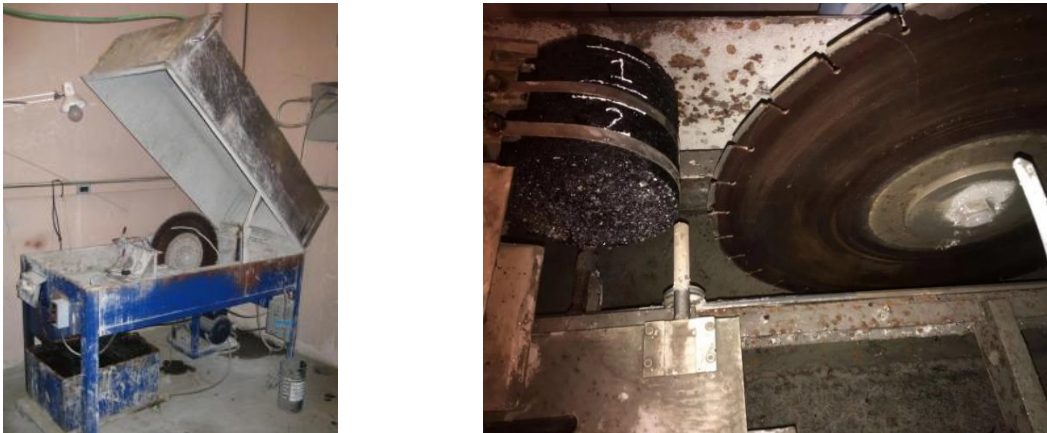
Figure 4-6. Superpave IDT specimen: (a) masonry saw; (b) cutting from an SGC pill
