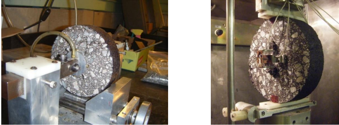
Figure 4-7. Use of strain gauges for accurate determination of fracture properties: (a) stainless steel gauge points attachment; (b) a specimen on the load frame with strain gauges
