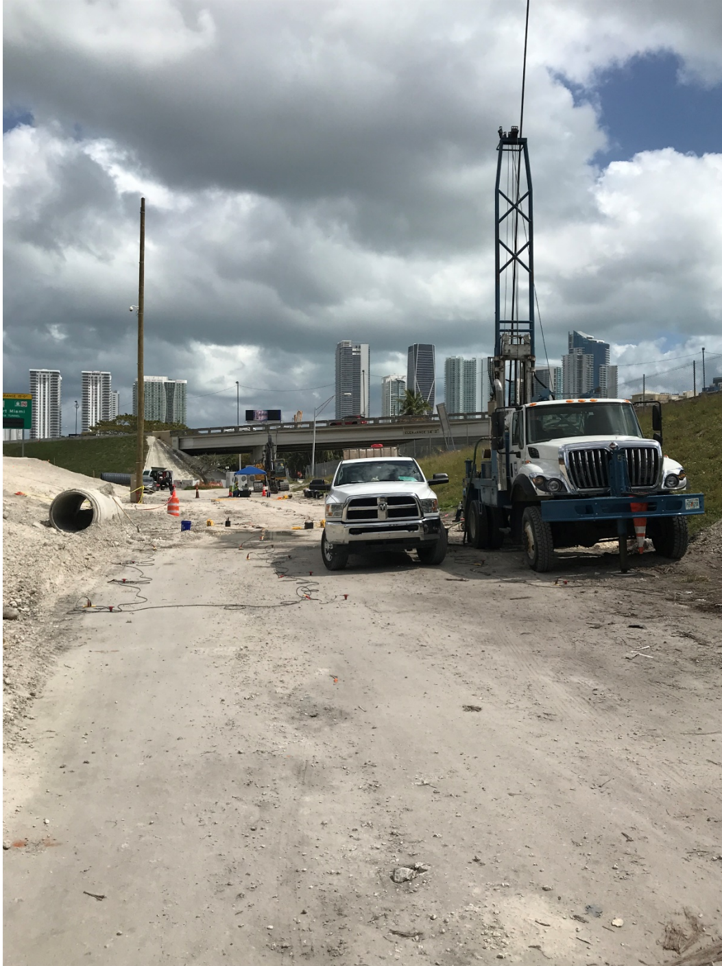
Figure 5.41: Miami test site: in-depth source using SPT seismic approach used to generate seismic waves
