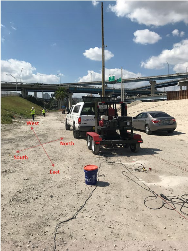
Figure 5.25: Miami test site: Large source used to generate seismic waves
