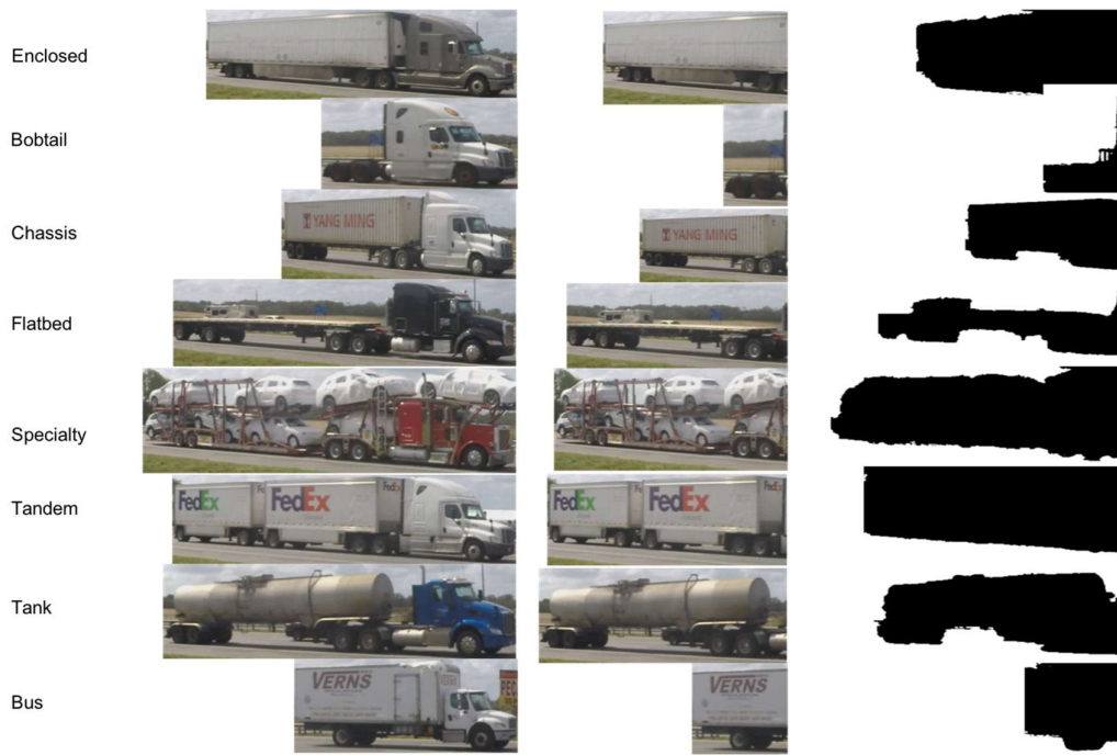
Figure 9: Sample-derived trailers and their corresponding contours. The results were derived from videos taken at I-75 site 9956.
