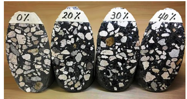
Cross-sections through a series of samples show increasing RAP content, from no RAP at left to 40% RAP at right.
