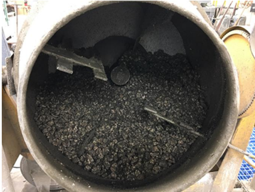
Figure 5-5. Mixing aggregates for 3 minutes to separate the RAP pieces
