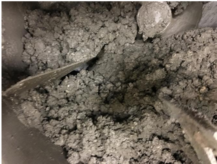
Figure 5-6. Finished concrete mixture incorporating RAP
