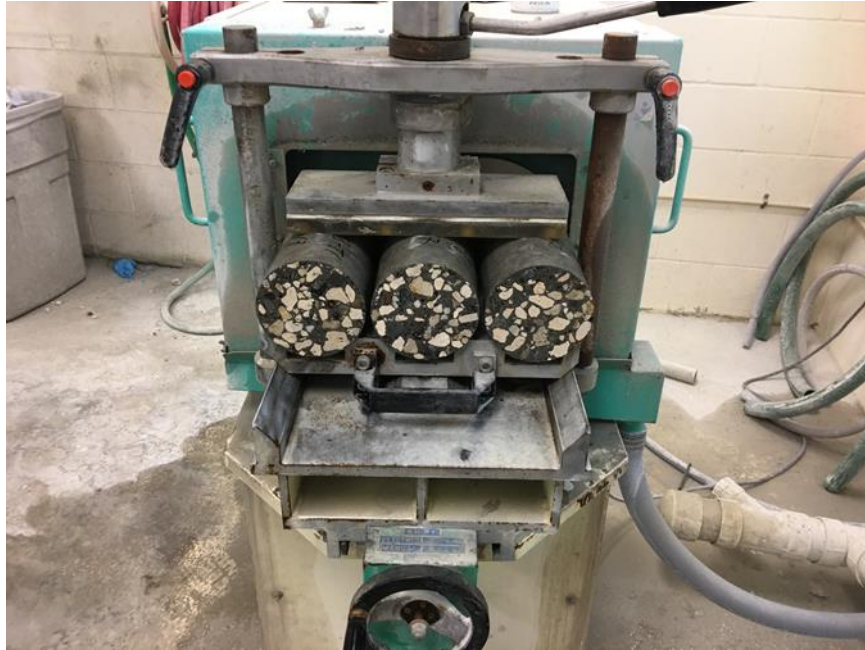
Figure 5-12. Grinding both ends of cylinder samples
