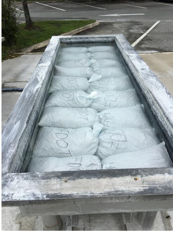
Figure 5-1. Pre-soaked coarse aggregate
