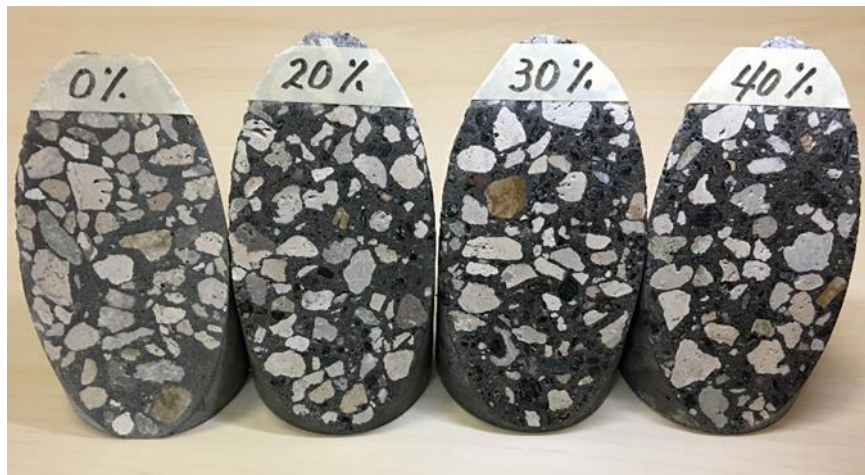
Figure 5-10. Hardened surface of concrete containing RAP
