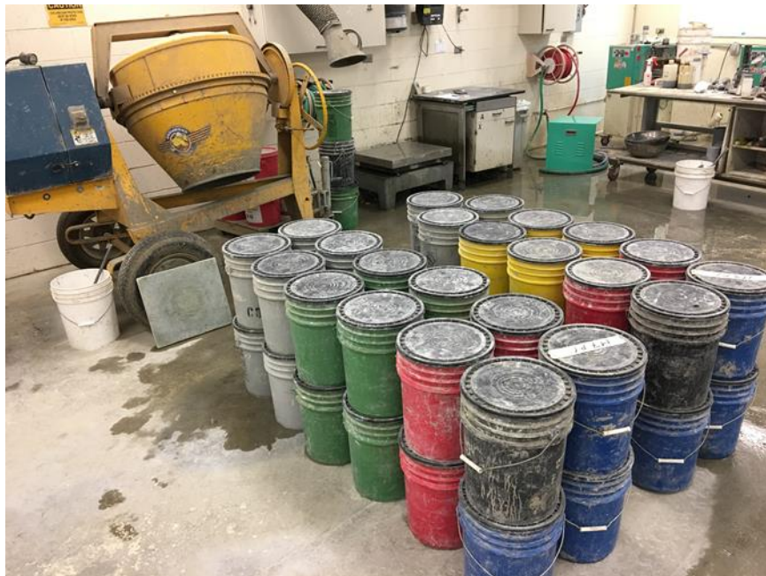
Figure 5-4. Weighted materials in buckets to be used for concrete production
