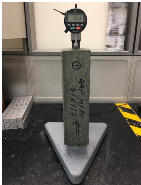
Figure 5-19. Drying shrinkage test set-up
