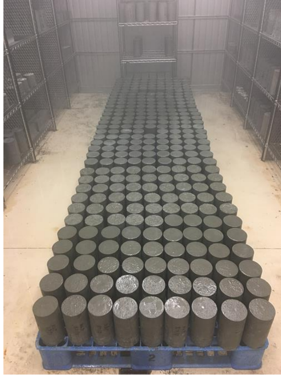
Figure 5-9. Samples in the moist room during curing
