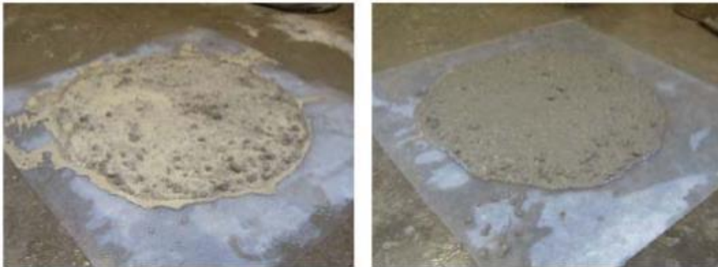
Figure 2-2. Examples of mixtures with insufficient paste volume (left) and sufficient paste volume (right) for filling ability (Koehler and Fowler, 2007)
