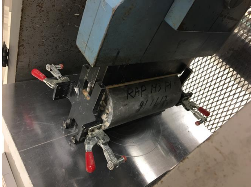
Figure 5-15. Splitting tensile strength test equipment
