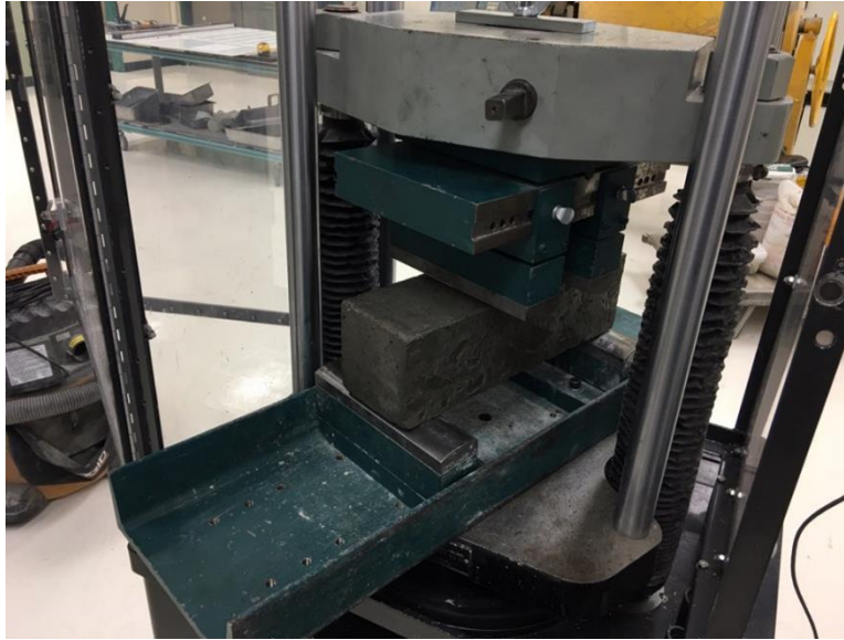
Figure 5-17. Flexural strength test set-up
