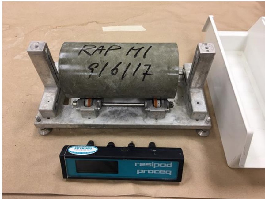
Figure 5-21. Surface resistivity test apparatus
