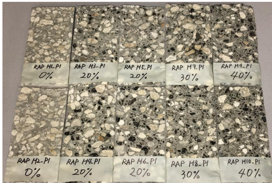
Figure 5-16. Concrete specimens after splitting tensile strength test
