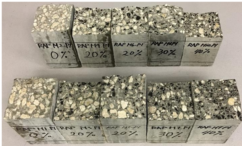
Figure 5-18. Concrete specimens tested in flexural strength
