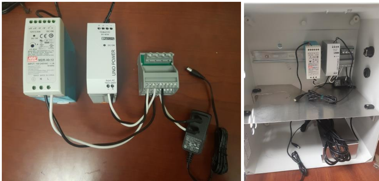
Figure 4-10. Power distribution block connected with power modules and converter (left). Connections mounted on DIN rail (right).
