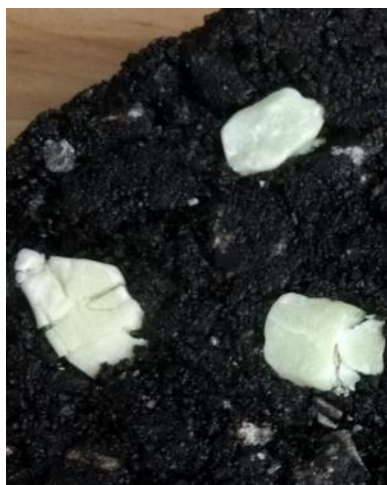
Figure 3-18. Cracked stones as a result of their large size and the compaction process.
