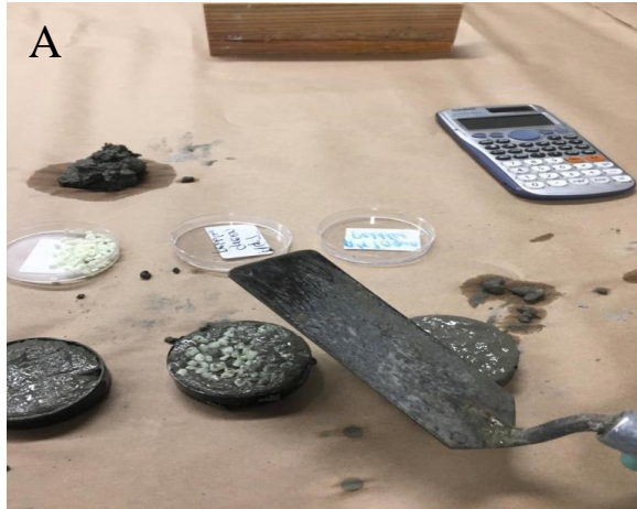
Figure 3-14. Experimental steps for stone placement: (A) Applying stones and smoothing with a trowel and (B) after retarder applied on the surface.
