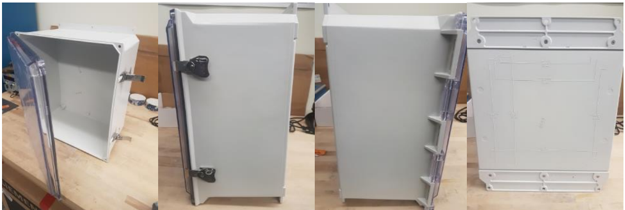
Figure 4-4. Fiberglass instrument enclosure without modifications.
