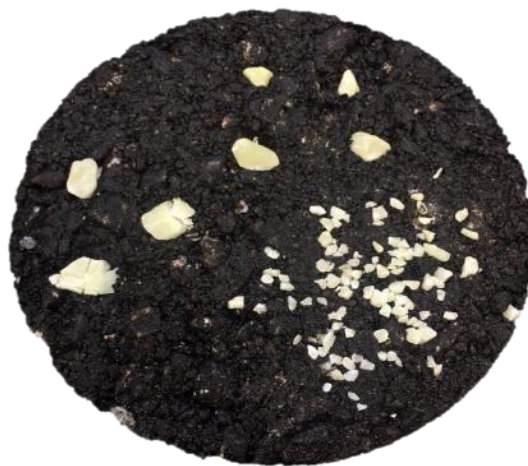
Figure 3-16. Compacted asphalt cylinder. Going in a clockwise manner, notice the 11- to 14-mm, 5- to 8-mm and 3- to 4- mm stones.
