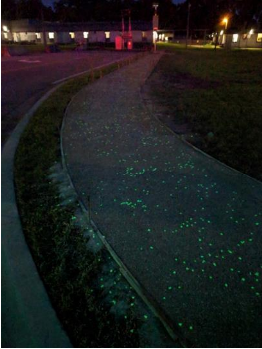
Figure 4-25. Glowing stones on the first night following installation. The surrounding ambient lighting severely hindered observation of the stones' performance.
