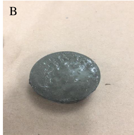
Figure 3-14. Experimental steps for stone placement: (A) Applying stones and smoothing with a trowel and (B) after retarder applied on the surface.
