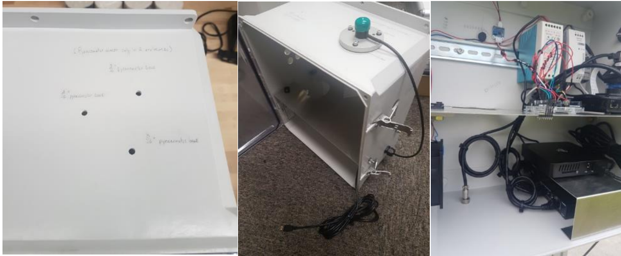
Figure 4-11. Three 3/16" holes for pyranometer attachment (left). Pyranometer locked in place and connected to Mini PC via USB cable (center). Raindrop sensor and outdoor temperature and humidity sensor connected to Arduino (right).
