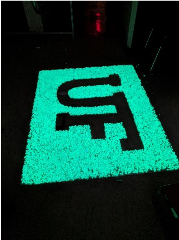
Figure 5-1. Glowing UF logo fabricated by placing Emerald Yellow glow stones on double-sided carpet tape.
