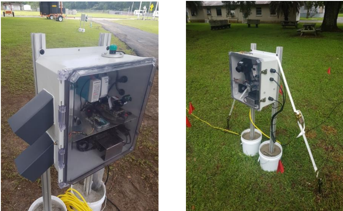
Figure 4-13. Enclosure set up with 80/20 extrusions and secured to the ground.
