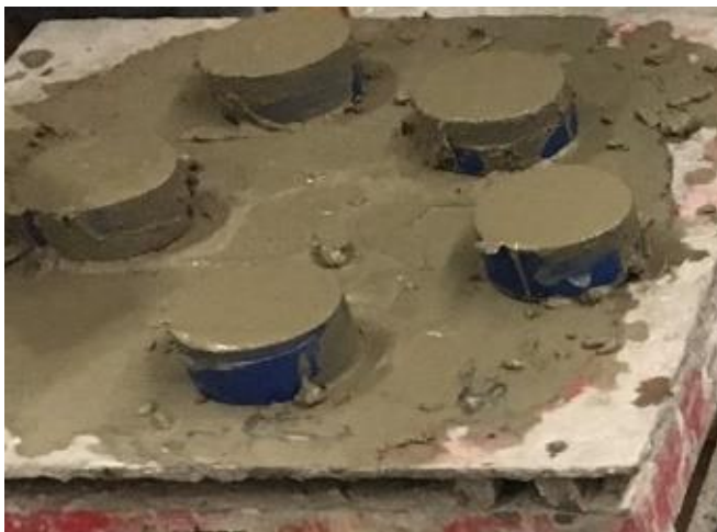
Figure 3-13. Flattened concrete samples placed on a vibrating table. The vibration allows the stones to set into the mix.
