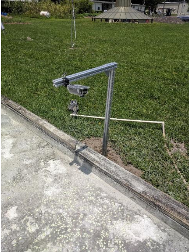
Figure 5-12. Time-lapse camera and concrete installation with Emerald Yellow glow stones embedded at UF's Energy Park.
