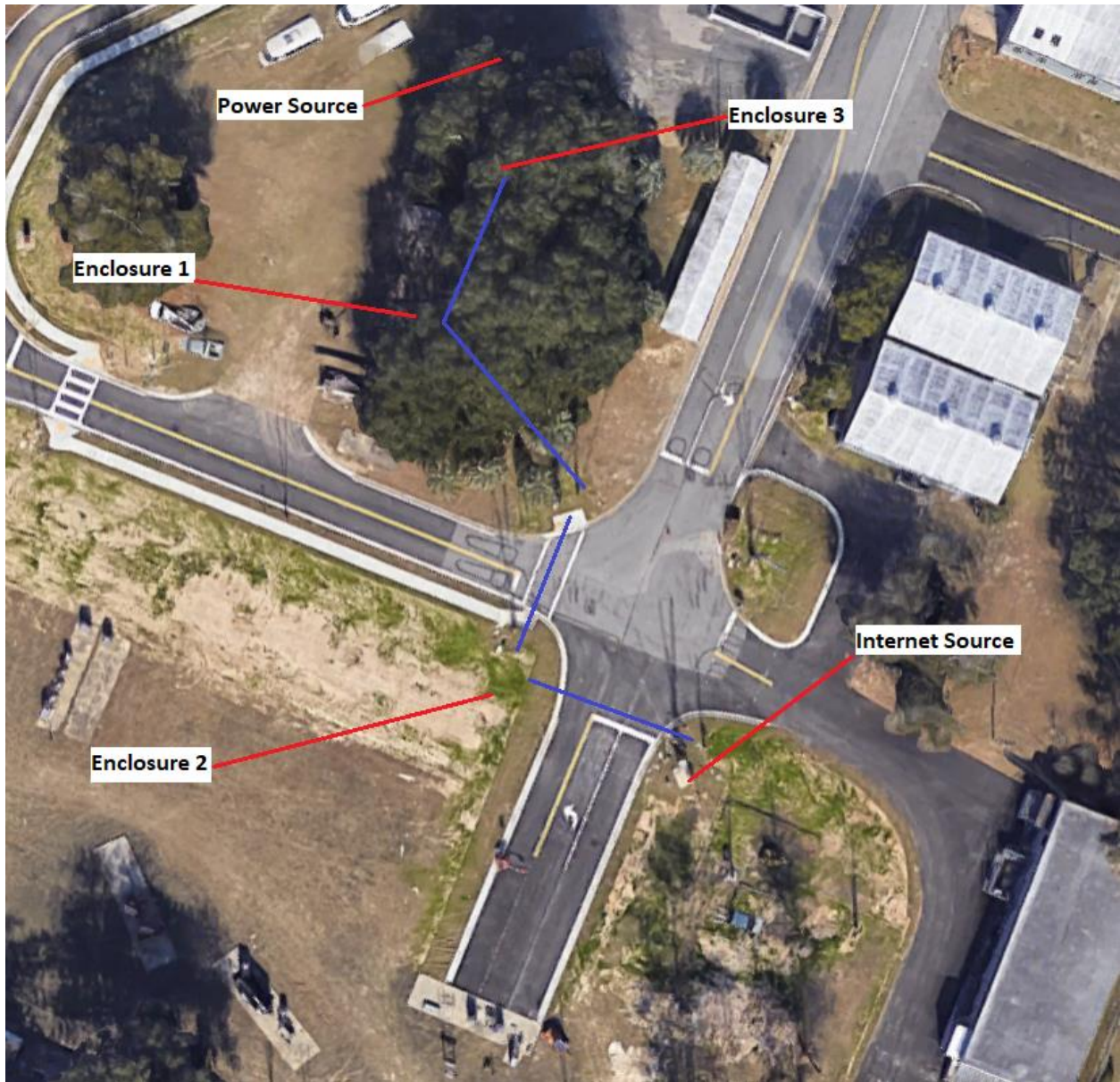
Figure 4-14. Location of enclosures on map. Blue lines denote Ethernet cables.
