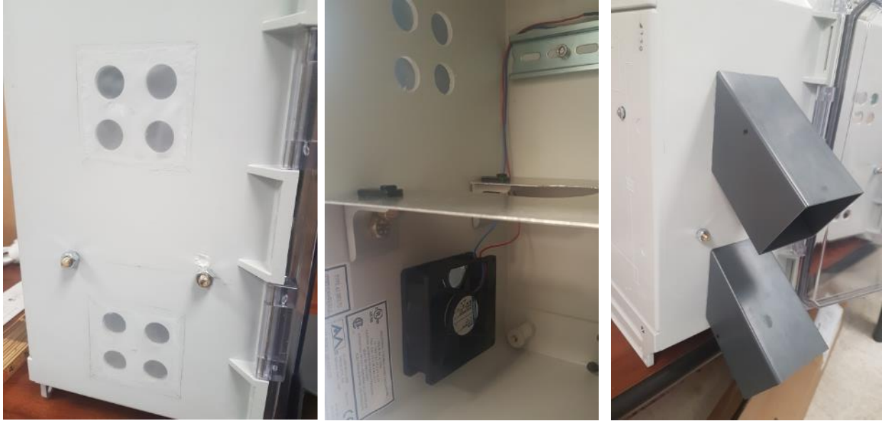
Figure 4-9. Ventilation system. Intake and exhaust with filter paper and powered by a computer fan. PVC pipe placed diagonally on the outside of the enclosure.
