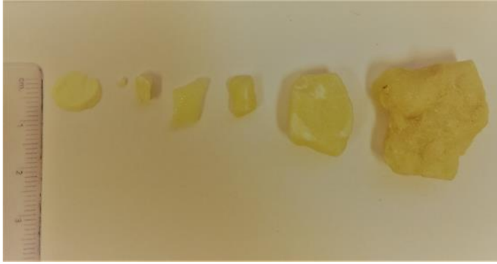
Figure 3-4. Size specification for samples. From left to right: powder, 1-mm pebble, 3- to 4-mm stone, 5- to 8-mm chip, 5- to 8-mm stone, 11- to 14-mm stone and a 25-mm rock.
