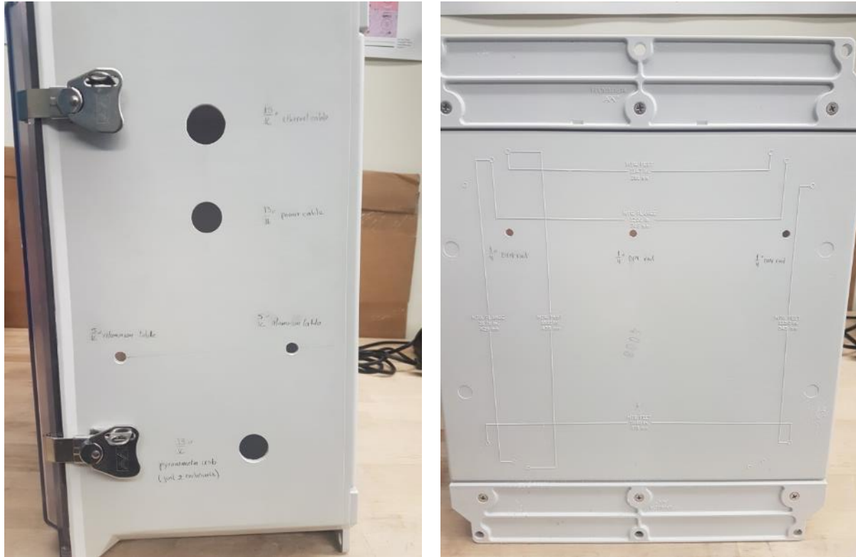
Figure 4-6. Holes drilled on the right side of the enclosure (left) and holes drilled on the back side of the enclosure (right).
