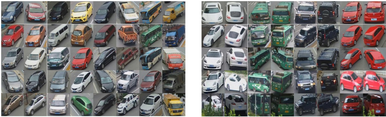
Figure 13: Vehicle samples selected from the VeRi dataset. All images are the same size, and we resize to 64 \times 128 for training. Left: Diversity of vehicle types and colors; right: variation resolutions, viewpoint, and occlusion. Source: Large-scale vehicle re-identification in urban surveillance videos, by Liu et al. published in IEEE International Conference on Multimedia and Expo (ICME), IEEE, New York, NY. Pg. 1–6, 2016.
