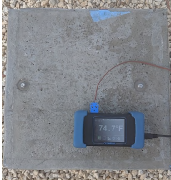
Figure 4-30: Durability block internal temperature measurement with embedded thermocouple.
