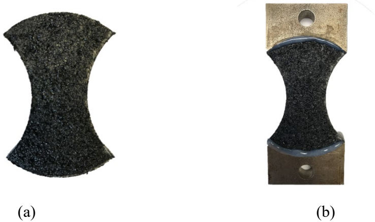
Figure 4-6. ICDT specimen: (a) compacted ICDT specimen and (b) ICDT specimen with loading head
