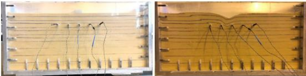
Figure 4.3 Pre and post-test failure surface for boundary condition experiment
