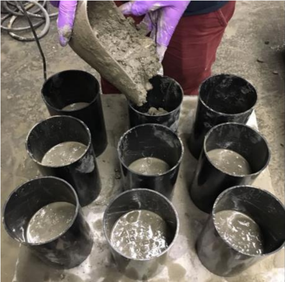
Figure 5-5: Cylinders after being filled with the first layer of concrete
