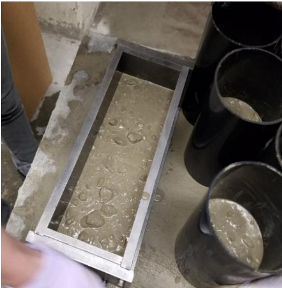
Figure 5-6: Concrete prism mold after first layer of concrete added
