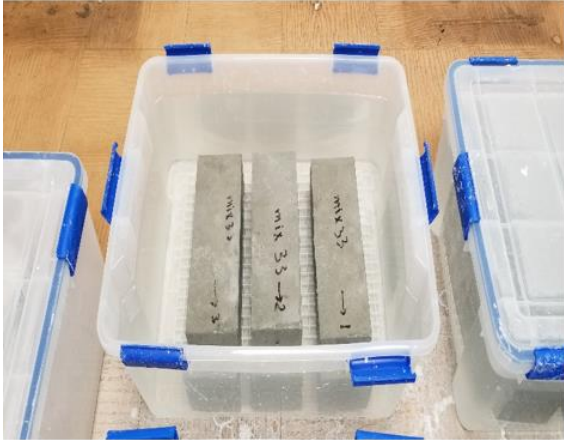
Figure 8-8: Prisms stored in 5% sodium sulfate solution
