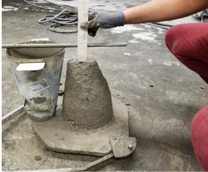
Figure 5-1: Determination of slump
