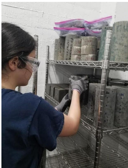
Figure 8-6: Samples placed in moist curing room for curing prior to sulfate exposure
