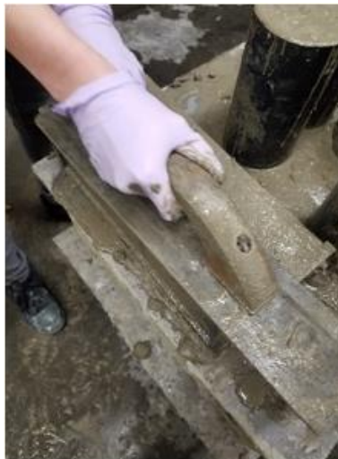
Figure 8-3: Prism being finished
