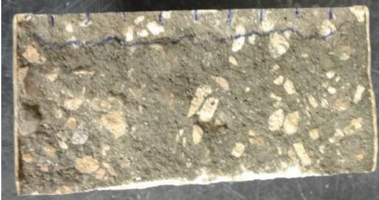
Figure 2-3: RCMT concrete specimen split open showing area near surface with elevated chloride levels stained by silver nitrate solution
