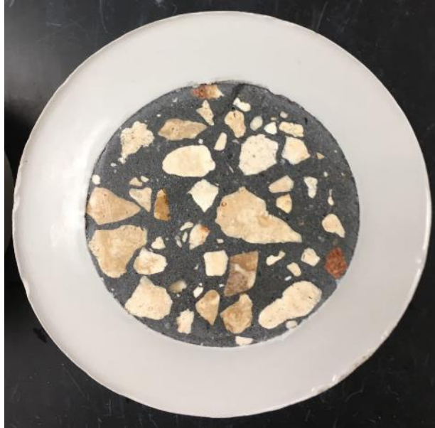
Figure 5-18: Test specimen prepared for the water permeability test
