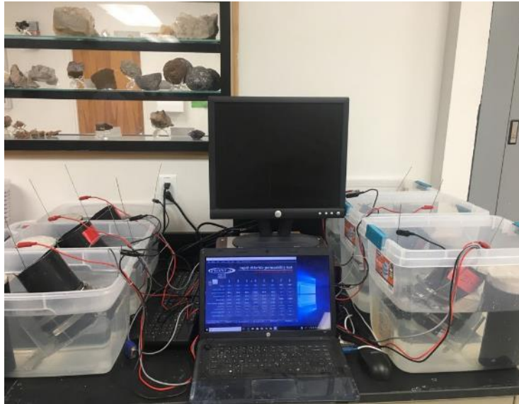
Figure 5-13: RCMT during testing
