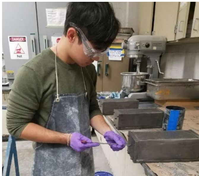
Figure 8-5: Prism demolding after initial curing
