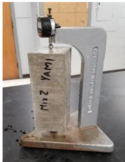
Figure 8-7: Concrete prism in length comparator
