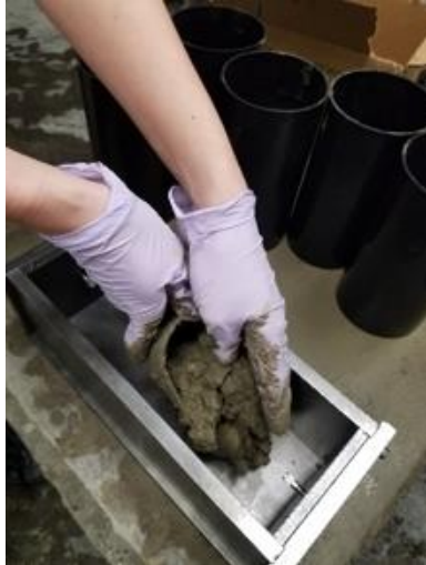
Figure 8-2: Concrete placement in mold
