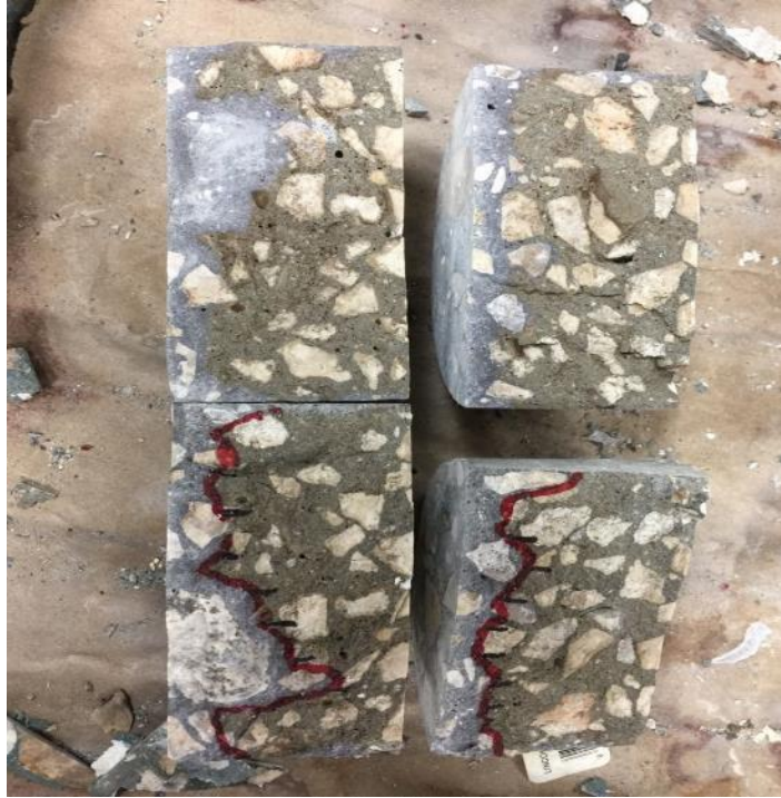
Figure 5-14: Split surface of the specimen sprayed with silver nitrate
