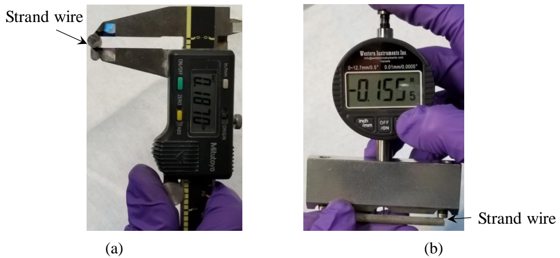
Figure 17-4. Corrosion evaluation of strands measurement (a) Loss in section (b) Pit depth
