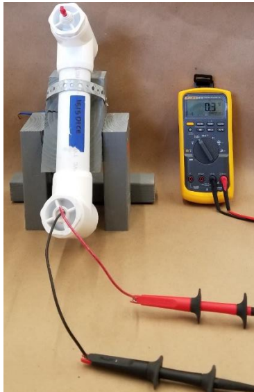
Figure 15-1. Corrosion potential measurement during drying
