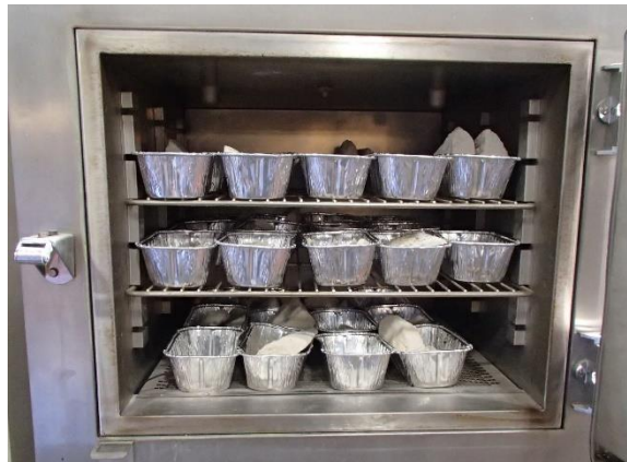
Figure 8-19. Oven drying of grout samples
