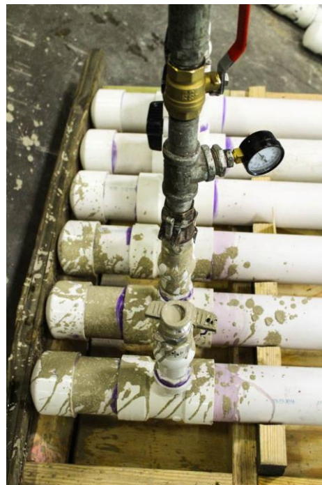
Figure A.3-4. Injection point
