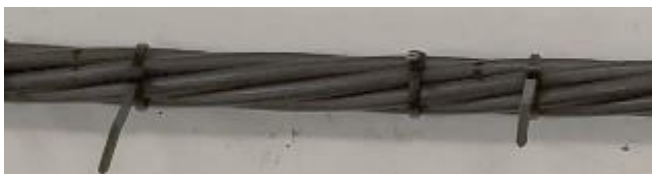
Figure 12-1. Zip ties and marks in preparation for strand cutting
