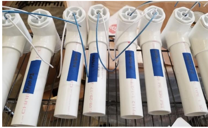
Figure 12-8. Specimens prepped for placement of first grout layer
