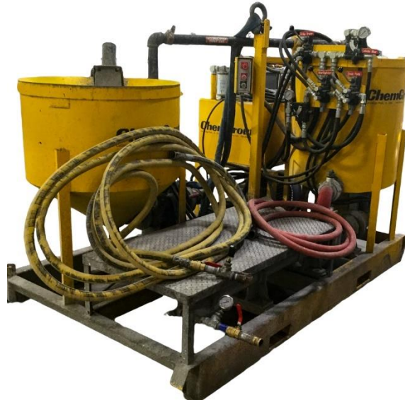
Figure A.3-3. Grout Plant
