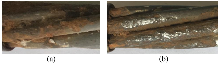
Figure 19-1. Corrosion rating = 6 for strand in 5 PC grout of 15 PC/5 PC D1C specimen: (a) Before cleaning; (b) After cleaning
