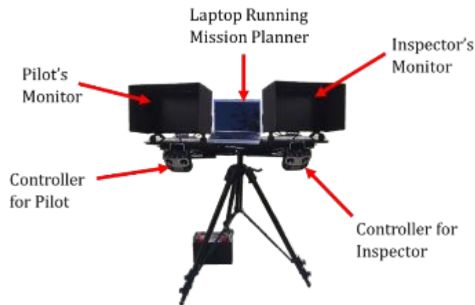
Figure 2-5. Ground station used during inspections
