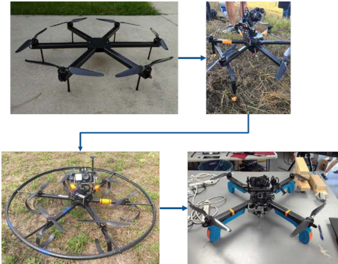
Figure 2-6. Changes to sUAV landing gear
