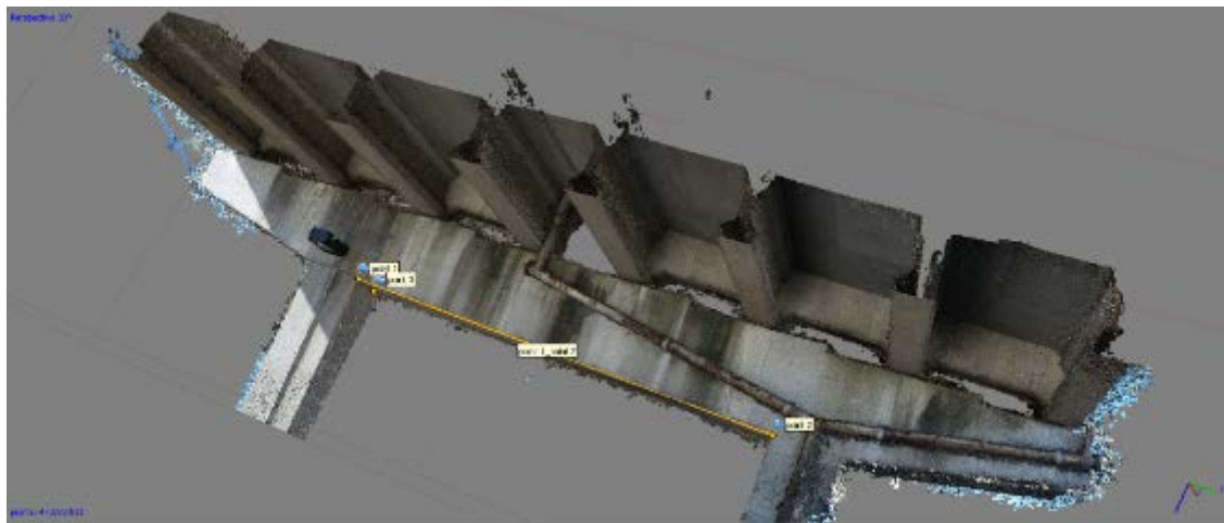
Figure 5-19. Reconstruction of Pier Cap 34 of 720114
