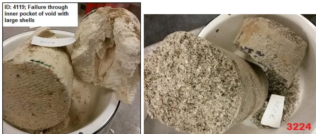
Figure D-1. Rock at failure surface apparently weaker than overall rock specimen
