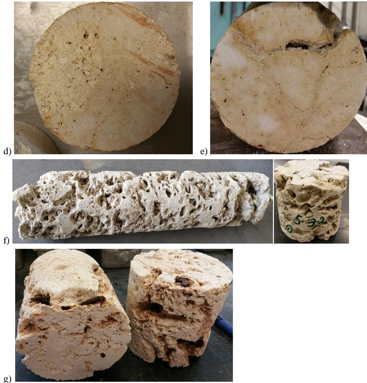
Figure 2-4. Continued; (d) Half solid, half porous specimen; (e) Solid rock with vug; (f) Vuggy and porous limestone specimens; (g) Fresh roots living in the vugs of limestone specimens
