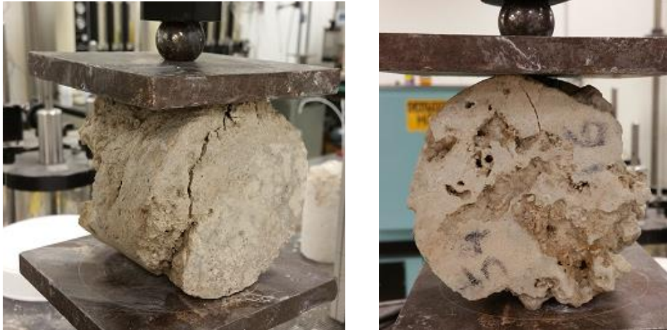
Figure 3-7. Non-center splitting—tests on samples 534-1 and 541-6
