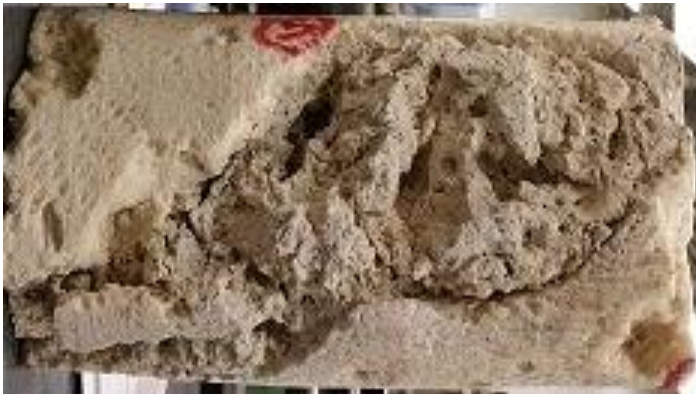
Figure 2-4. Heterogeneous rock specimens: (a) Half vuggy limestone, half coralline specimen; (b) "Scaled" coralline limestone specimen; (c) Two different limestones within one specimen
