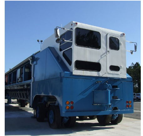
The heavy vehicle simulator can simulate up to 20 years of pavement wear in about three months.
