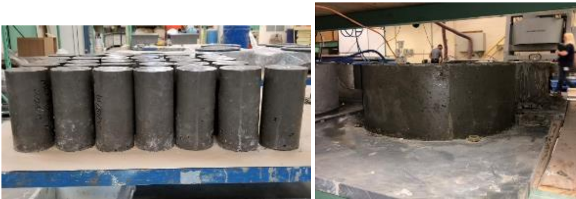
Fig 3.6 Cylinder specimens (left) and ring specimen (right) after unmolding.
