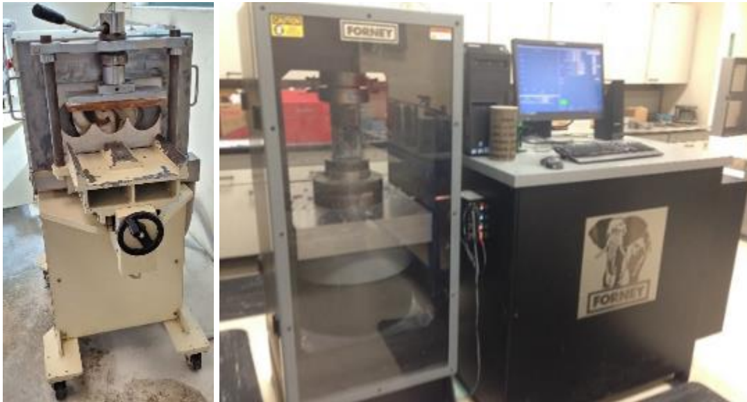
Fig 3.10 Automatic grinding machine (left) and compressive strength specimen being tested (right).
