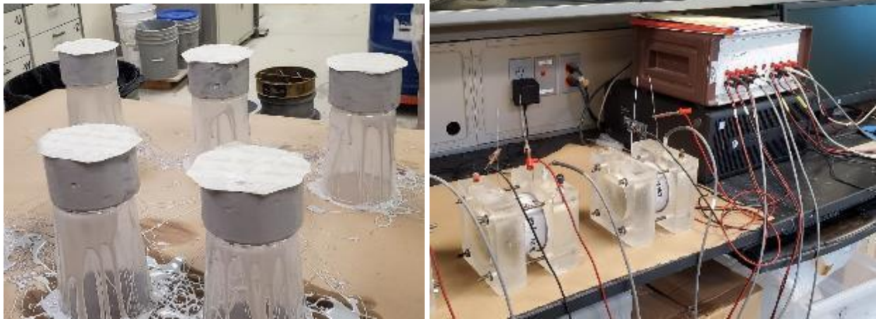
Fig 3.19 RCP specimens coated with epoxy (left) and being tested (right).
