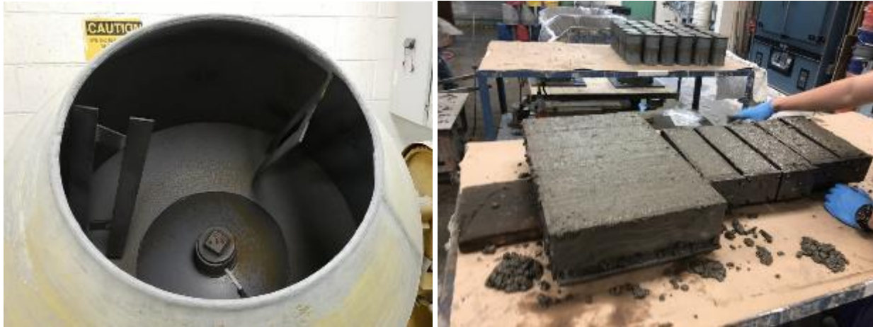
Fig 3.5 Drum mixer used for production mixing (left) and beam, prism, and cylinder specimens after consolidation (right).
