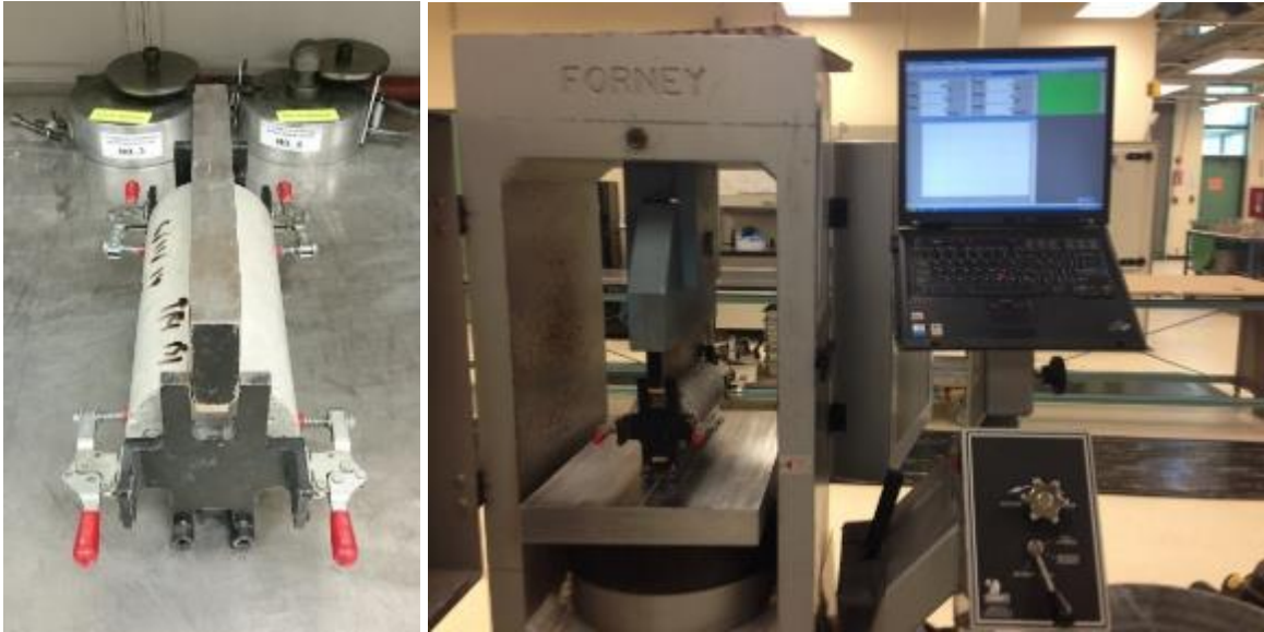
Fig 3.11 Splitting tensile testing apparatus (left) and splitting tensile strength specimen being tested (right).
